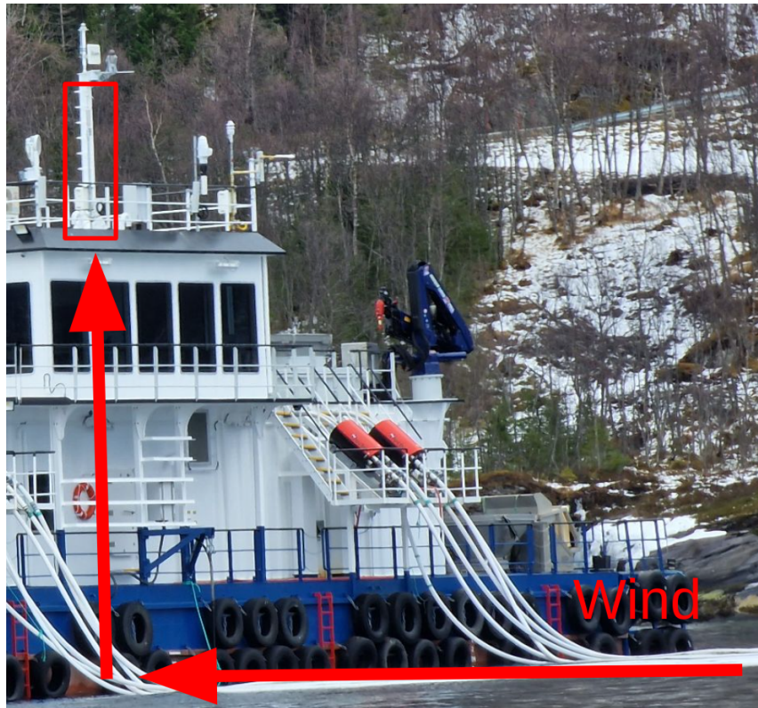
Figure 18: Feeding barge affecting the vertical wind velocities during southwesterly flow. Photo: Eirik Mikal Samuelsen.
