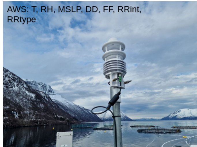
Figure 2: All weather sensor (AWS) with outputs like temperature ( T ), relative humidity ( RH ), mean sea level pressure ( MSLP ), horizontal wind direction ( DD ), horizontal wind speed ( FF ), precipitation intensity ( RR_{int} ), and precipitation type ( RR_{type} ). Photo: Eirik Mikal Samuelsen.
