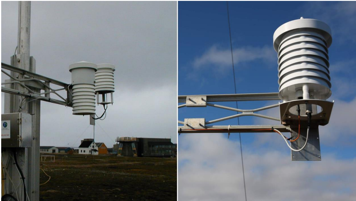
FIGURE 7 | Cylindrical temperature screens. Left: Photo from 2000 of with temperature and humidity sensors in separate screens. The smaller screen to the right is the MI-74, a circular double louvered plastic screen. The one on the left was used for the humidity sensor before both temperature and humidity sensor were placed in the same screen in 2013. Right: The MI-2001B, a circular double louvered plastic screen with co-located temperature and humidity sensor, photo taken in 2013. Photo: MET Norway.
