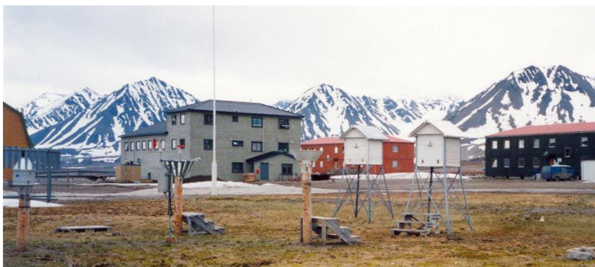
FIGURE 6 | The two temperature screens MI-33 (left) and MI-46 (right) in 1994. The MI-33 has double-boarded walls and floor and was to be used at sites in harsh climates. The MI-46 has double-boarded floor and walls to the north and south, while the eastern and western walls are double-louvered. Of the precipitation gauges in the picture, the gauge to the left is the Geonor T-200 (automatic gauge). The gauge in the middle is a Russian type (used for test purposes). To the right is the manual Norwegian gauge. Photo: MET Norway.
