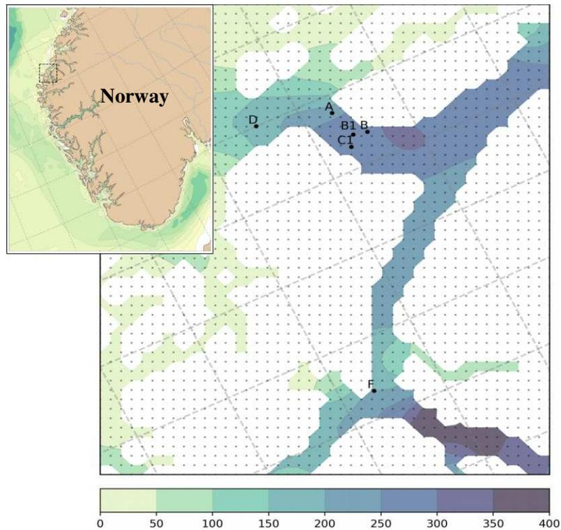
Figure 5: Distribution of moorings in Sulafjorden (A, B, B1, C1), Breisundet (D) and Vartdalsfjorden (F) as part of the project “Fergefri E39” at the West Coast of Norway. The color scale ranging from 0 to 400 meters indicates the depth of the NorKyst800 model in the area. Also shown are the grid points of the model (small gray dots).
