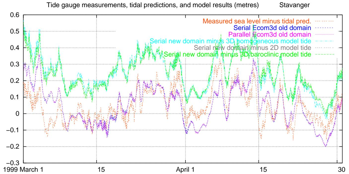
Fig. 36. Measured and modelled water level, excluding tides, Stavanger, 1999 March–April
