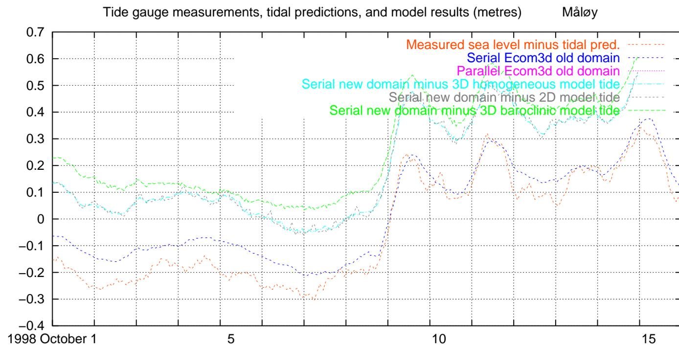
Fig. 43. Measured and modelled water level, excluding tides, Måløy, 1998 October 1–15
