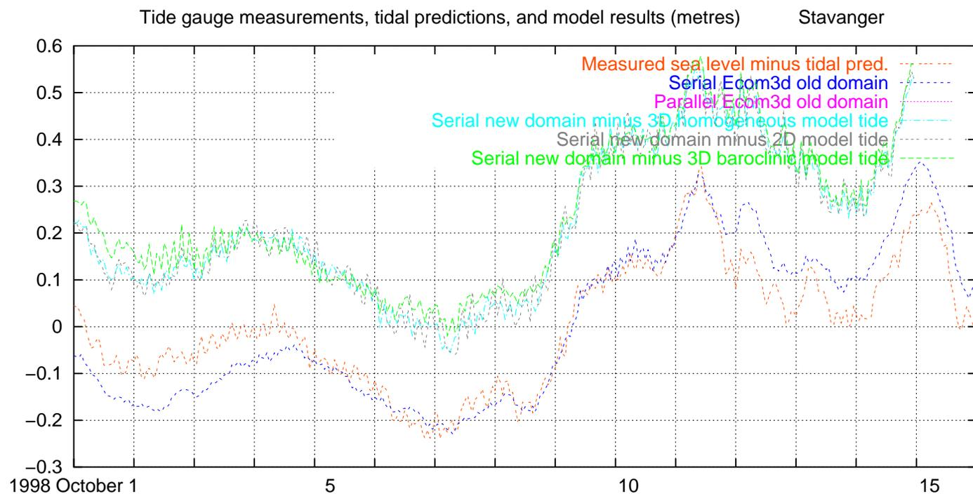
Fig. 35. Measured and modelled water level, excluding tides, Stavanger, 1998 October 1–15
