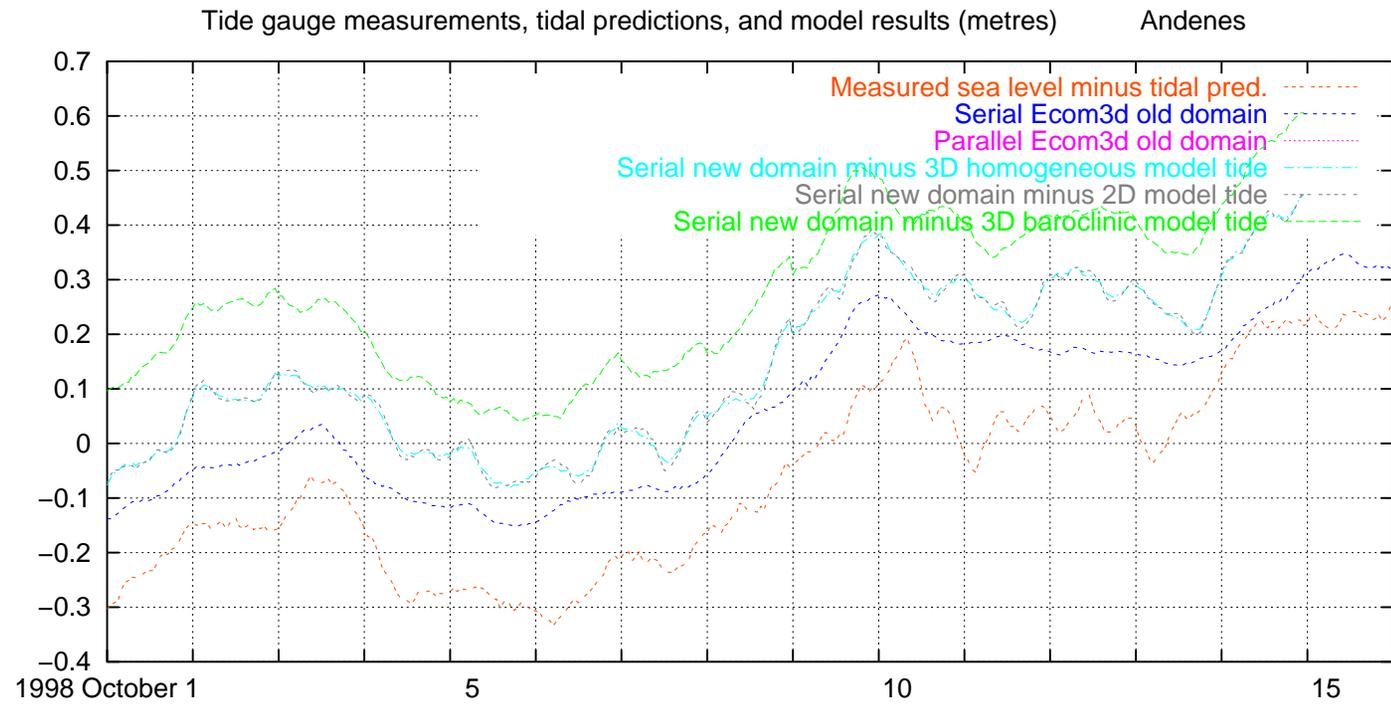
Fig. 79. Measured and modelled water level, excluding tides, Andenes, 1998 October 1–15
