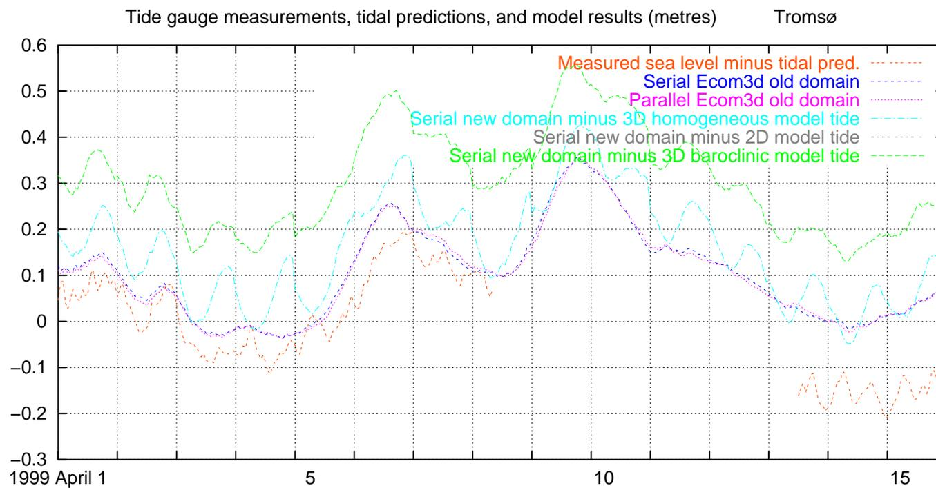
Fig. 85. Measured and modelled water level, excluding tides, Tromsø, 1999 April 1–15
