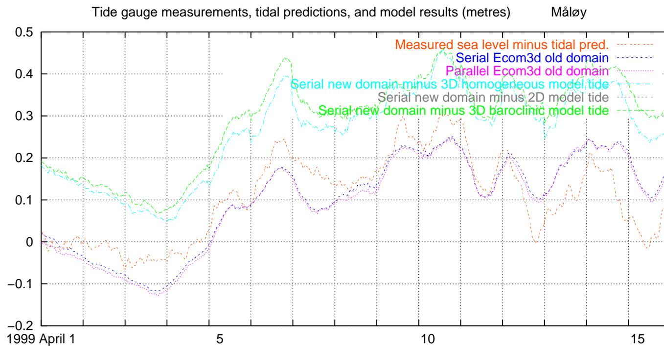
Fig. 45. Measured and modelled water level, excluding tides, Måløy, 1999 April 1–15
