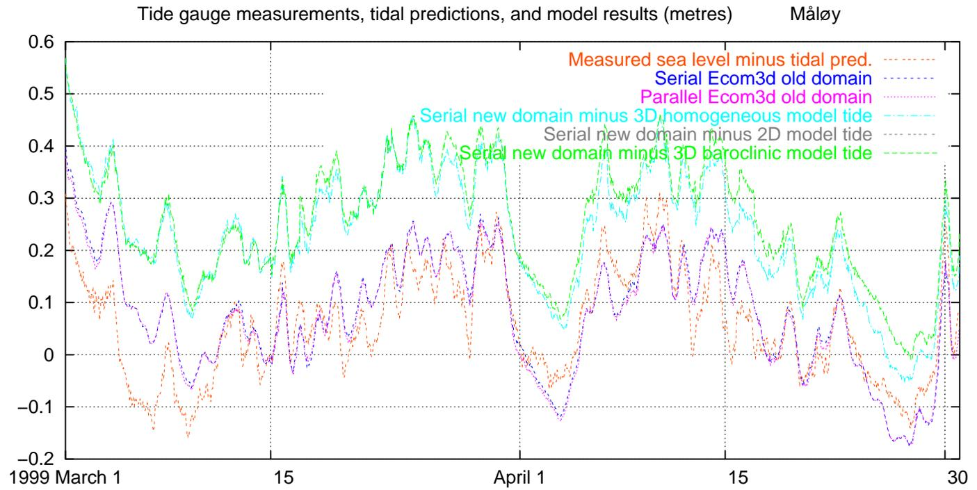
Fig. 44. Measured and modelled water level, excluding tides, Måløy, 1999 March–April
