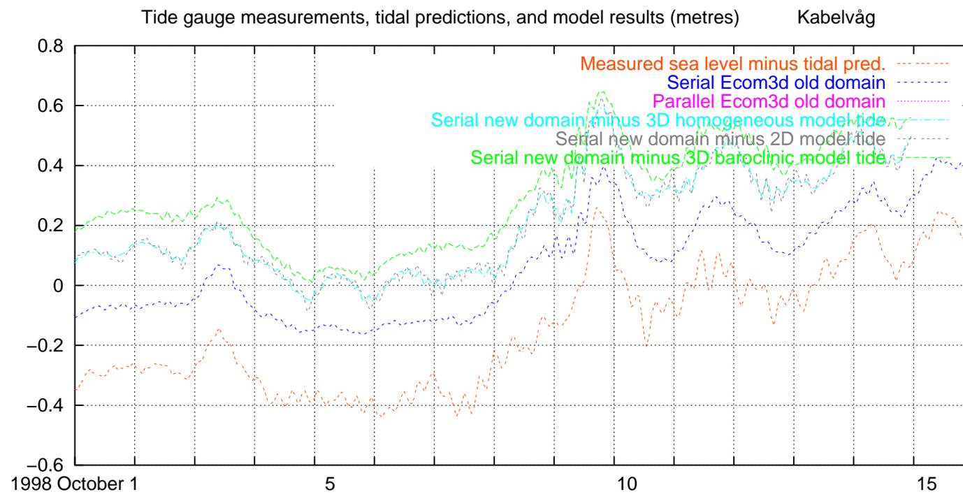
Fig. 67. Measured and modelled water level, excluding tides, Kabelvåg, 1998 October 1–15
