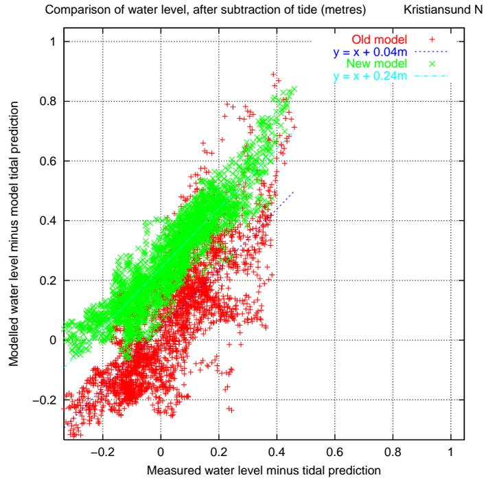
Fig. 11. Modelled v. measured water level for Kristiansund N
