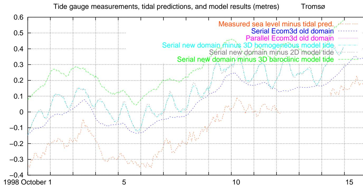
Fig. 83. Measured and modelled water level, excluding tides, Tromsø, 1998 October 1–15
