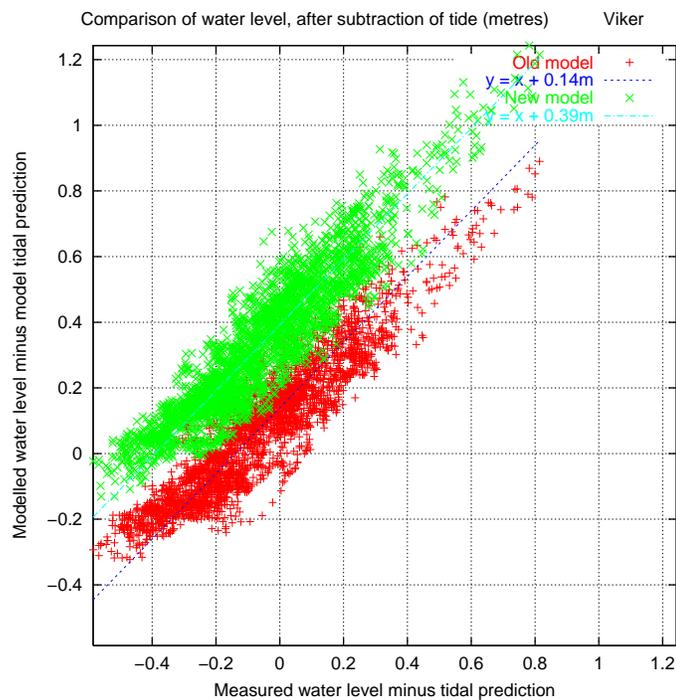
Fig. 4. Modelled v. measured water level for Viker
