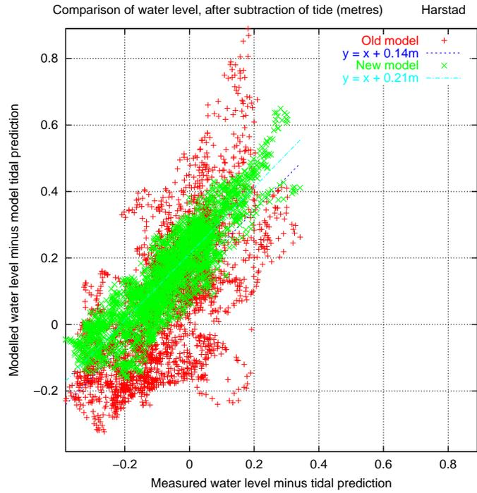
Fig. 17. Modelled v. measured water level for Harstad
