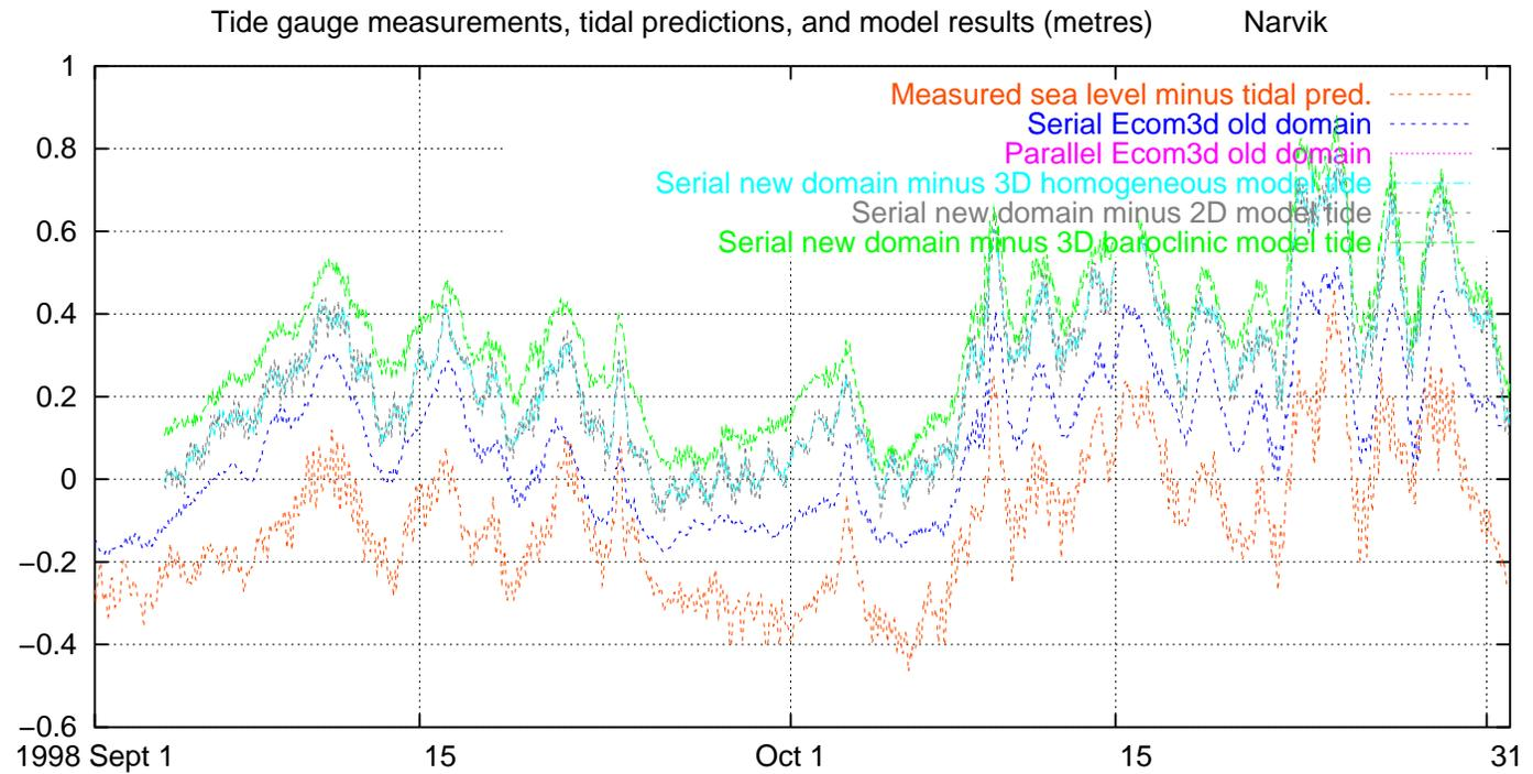
Fig. 70. Measured and modelled water level, excluding tides, Narvik, 1998 September–October
