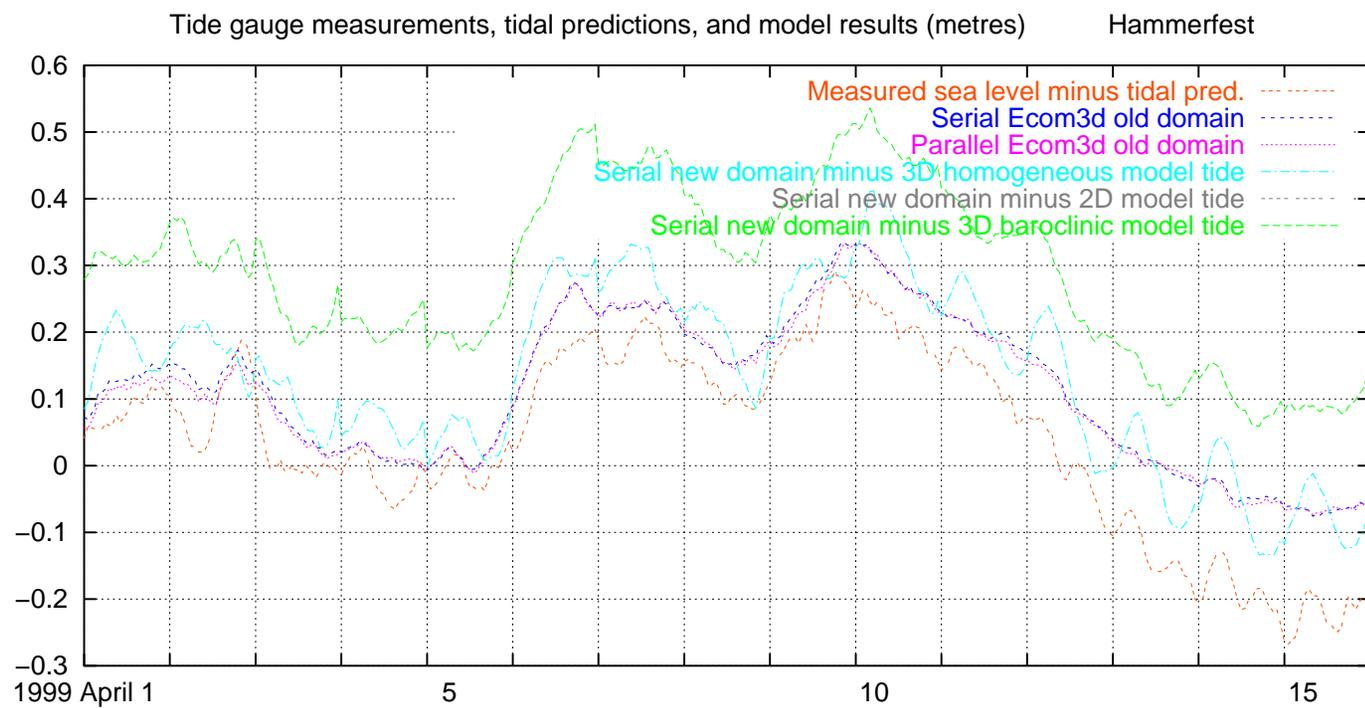
Fig. 89. Measured and modelled water level, excluding tides, Hammerfest, 1999 April 1–15
