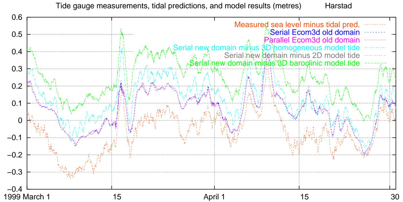
Fig. 76. Measured and modelled water level, excluding tides, Harstad, 1999 March–April
