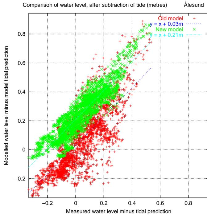
Fig. 10. Modelled v. measured water level for Ålesund
