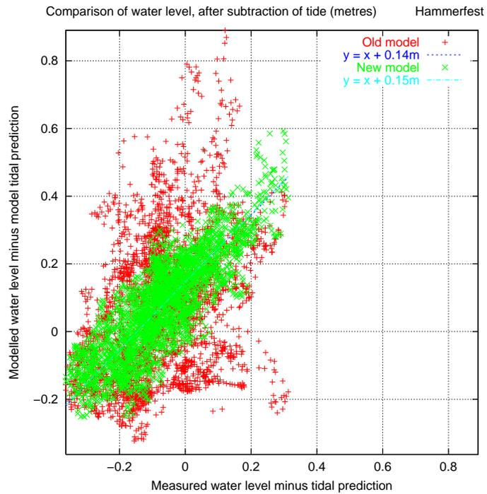
Fig. 20. Modelled v. measured water level for Hammerfest
