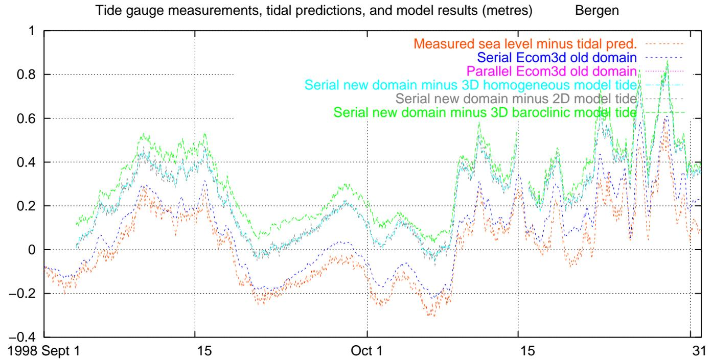
Fig. 38. Measured and modelled water level, excluding tides, Bergen, 1998 September–October
