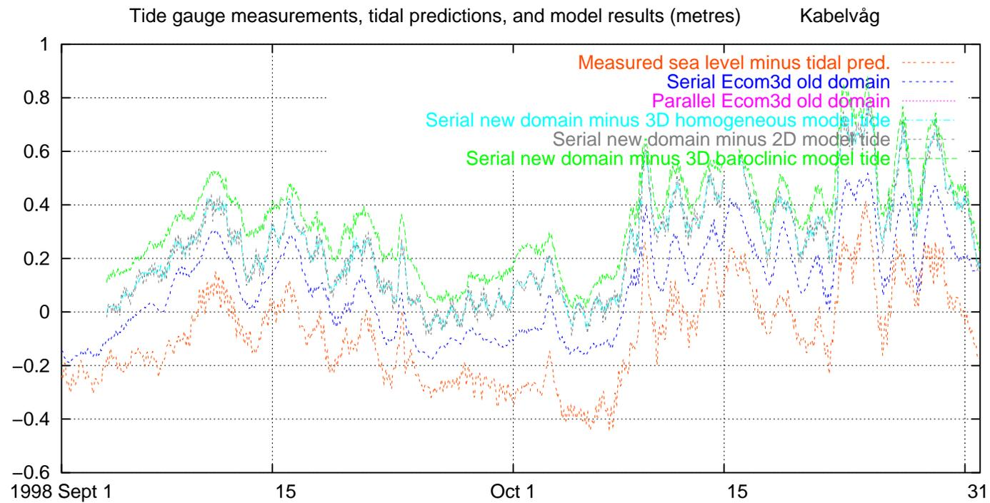
Fig. 66. Measured and modelled water level, excluding tides, Kabelvåg, 1998 September–October
