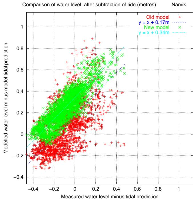
Fig. 16. Modelled v. measured water level for Narvik
