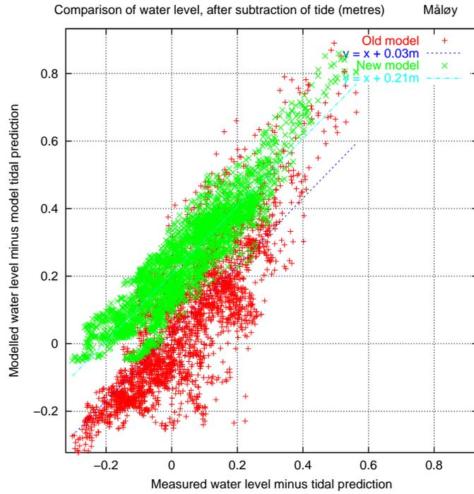
Fig. 9. Modelled v. measured water level for Måløy
