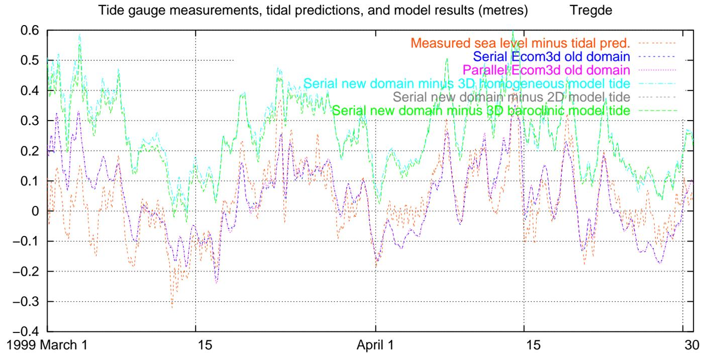
Fig. 32. Measured and modelled water level, excluding tides, Tregde, 1999 March–April
