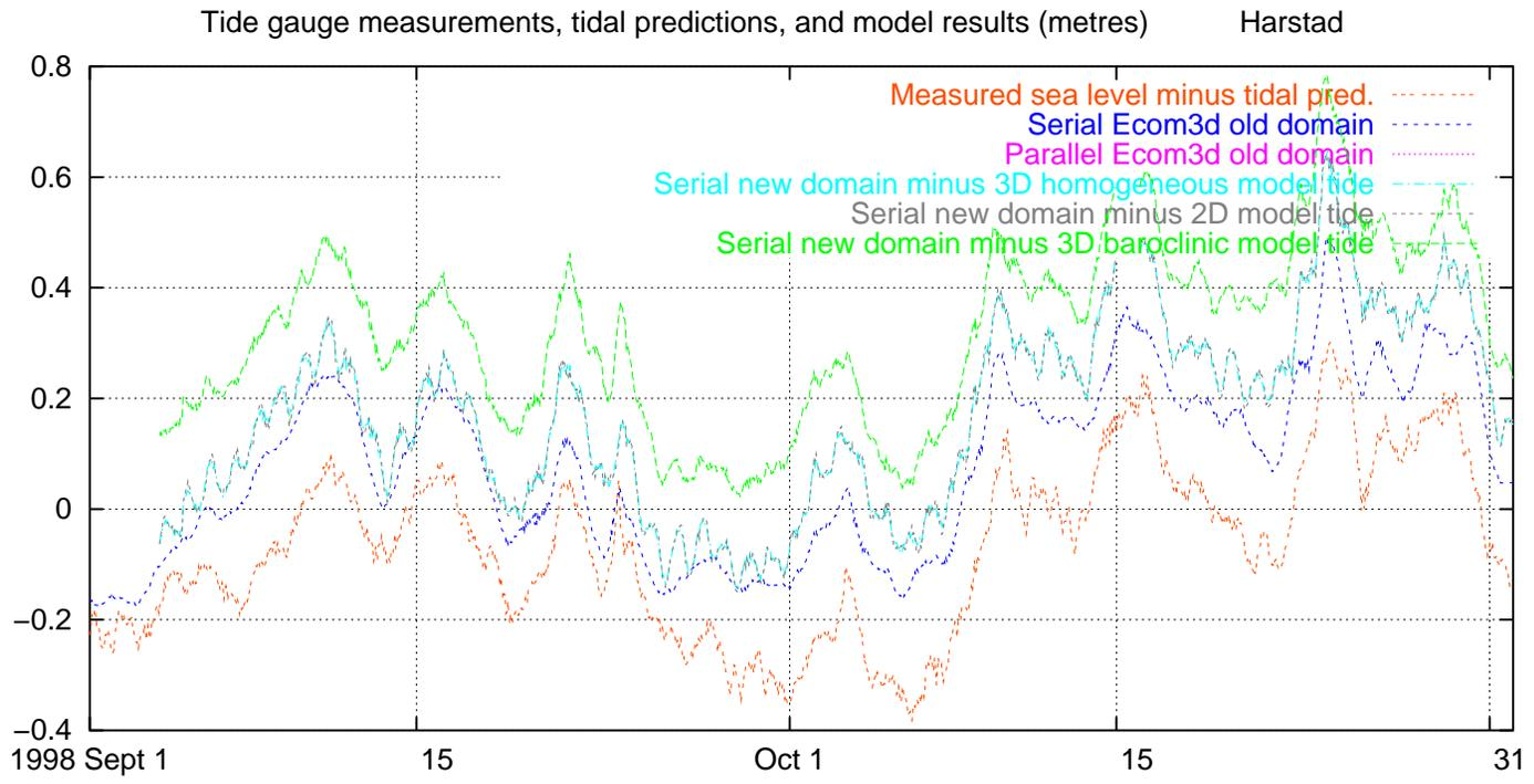
Fig. 74. Measured and modelled water level, excluding tides, Harstad, 1998 September–October
