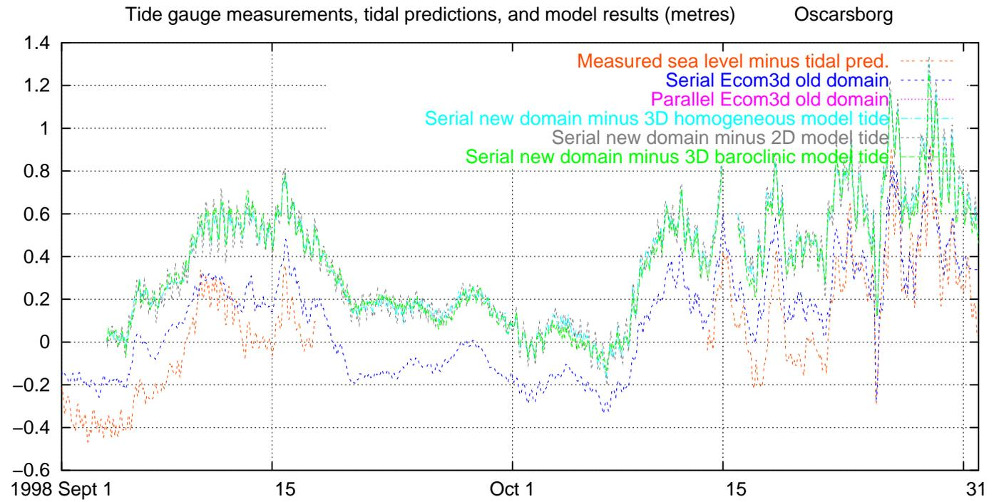
Fig. 26. Measured and modelled water level, excluding tides, Oscarsborg, 1998 September–October
