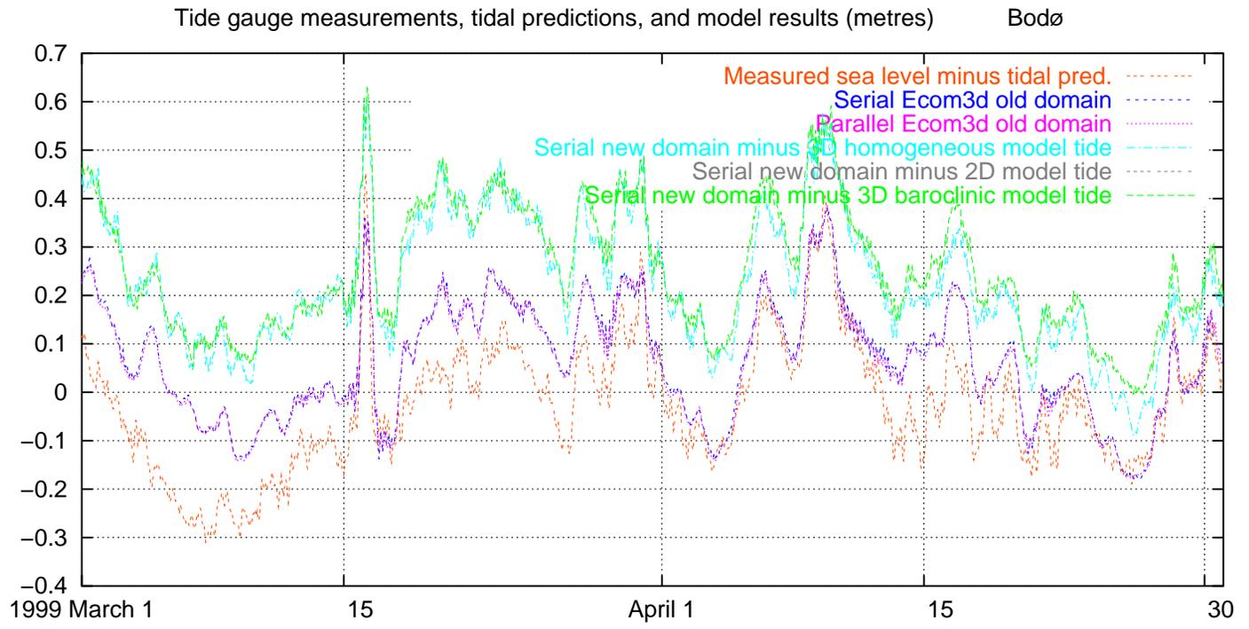
Fig. 64. Measured and modelled water level, excluding tides, Bodø, 1999 March–April
