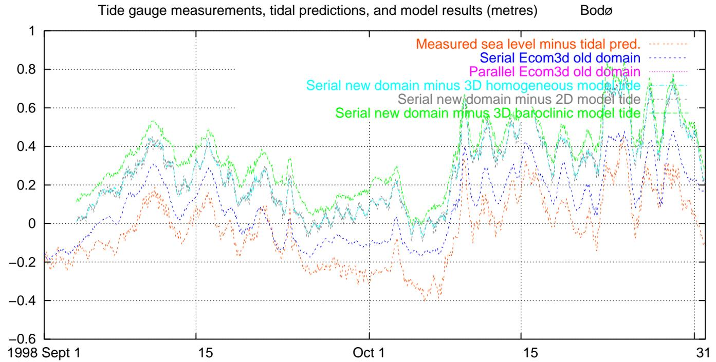
Fig. 62. Measured and modelled water level, excluding tides, Bodø, 1998 September–October
