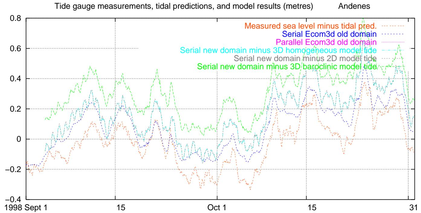
Fig. 78. Measured and modelled water level, excluding tides, Andenes, 1998 September–October
