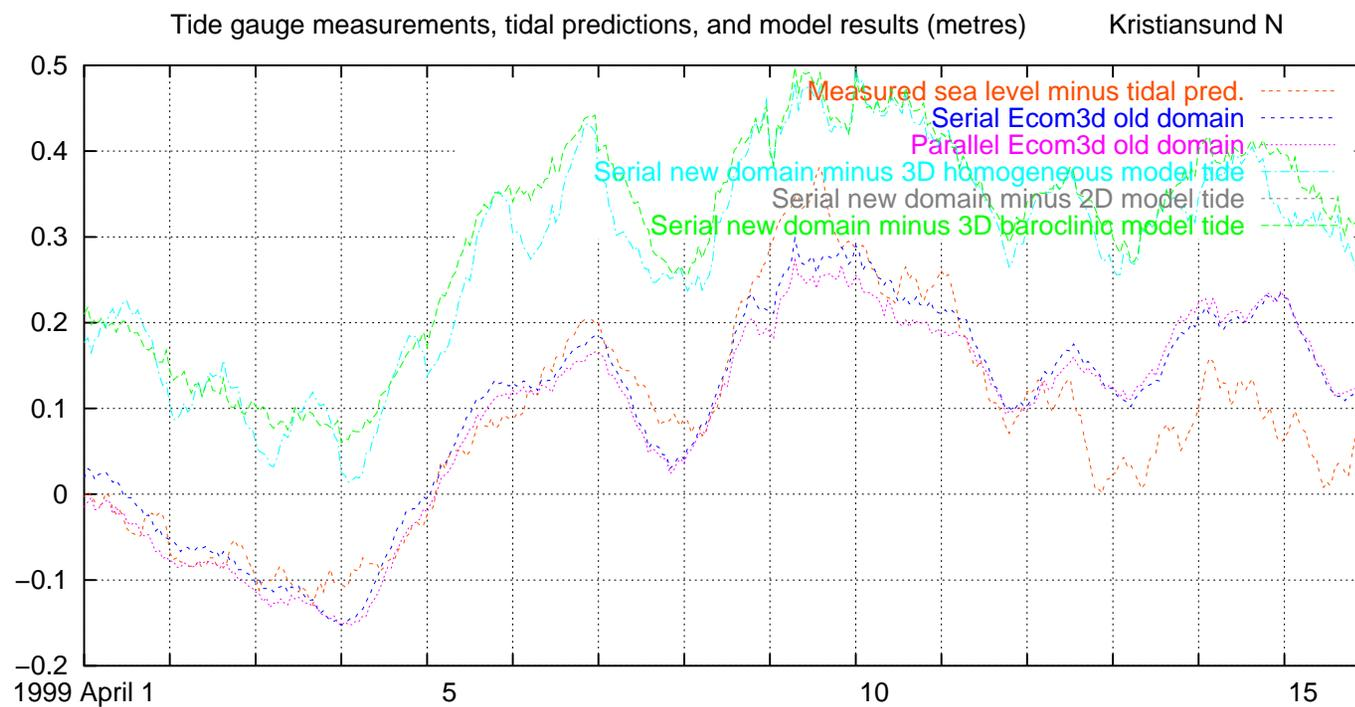
Fig. 53. Measured and modelled water level, excluding tides, Kristiansund N, 1999 April 1–15
