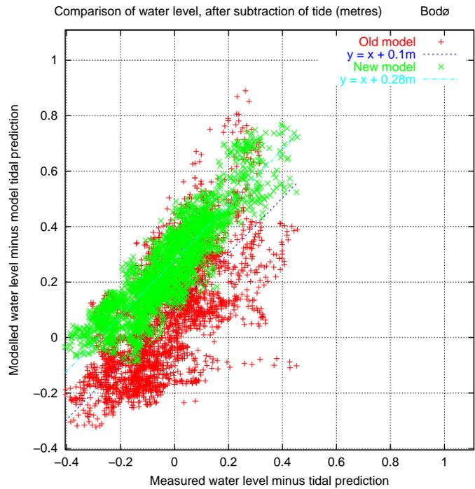
Fig. 14. Modelled v. measured water level for Bodø
