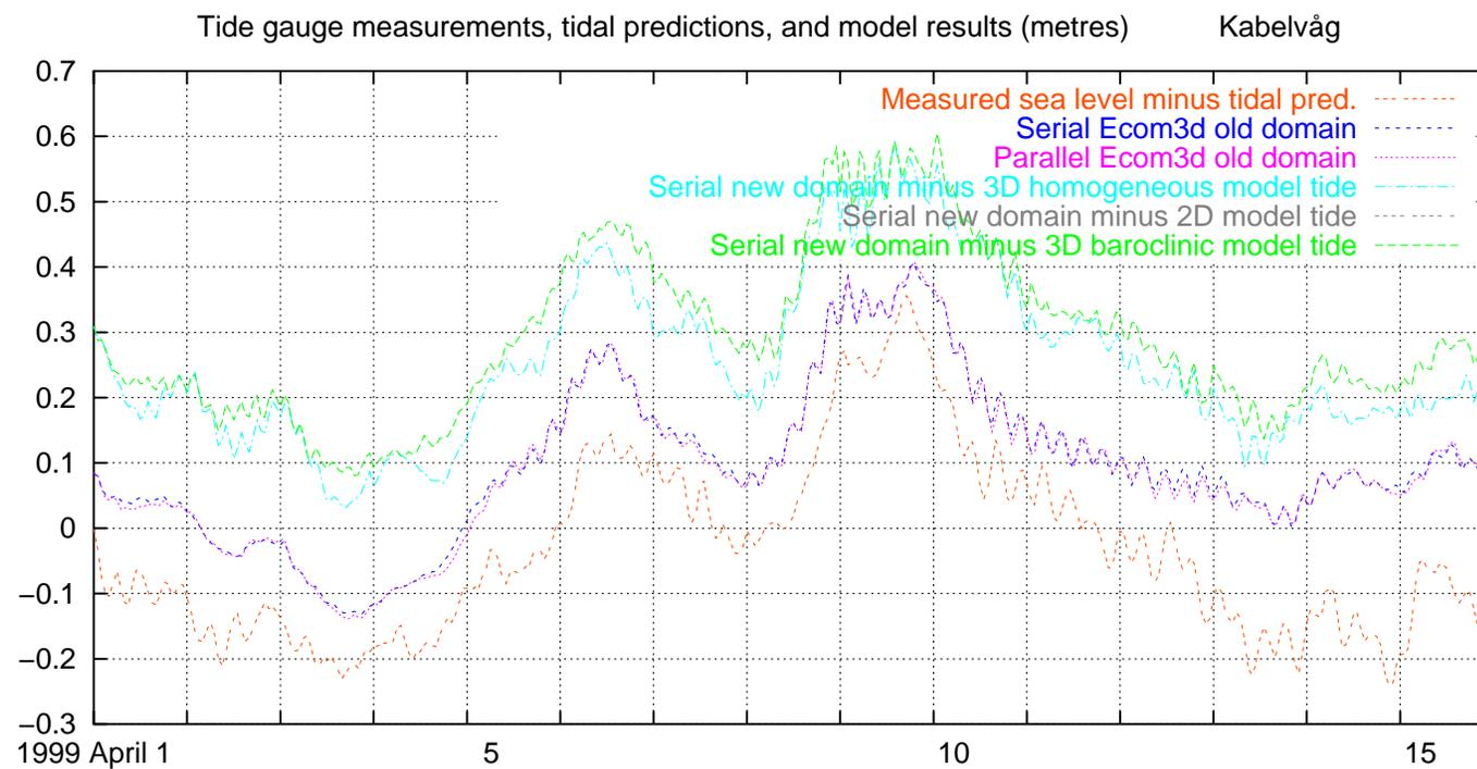
Fig. 69. Measured and modelled water level, excluding tides, Kabelvåg, 1999 April 1–15
