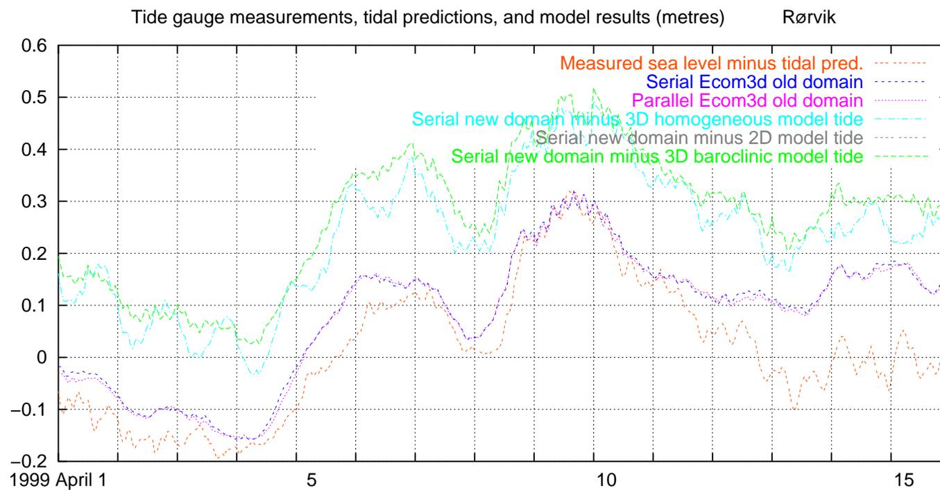
Fig. 61. Measured and modelled water level, excluding tides, Rørvik, 1999 April 1–15
