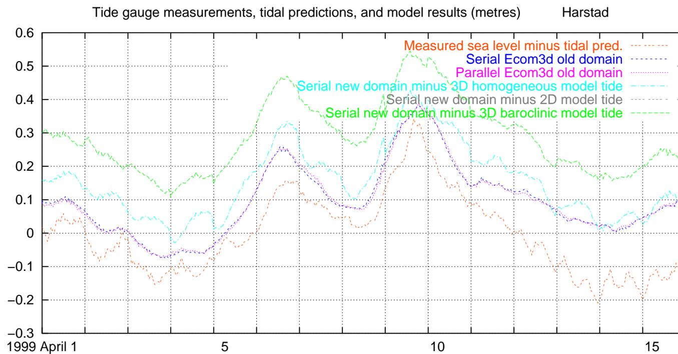
Fig. 77. Measured and modelled water level, excluding tides, Harstad, 1999 April 1–15
