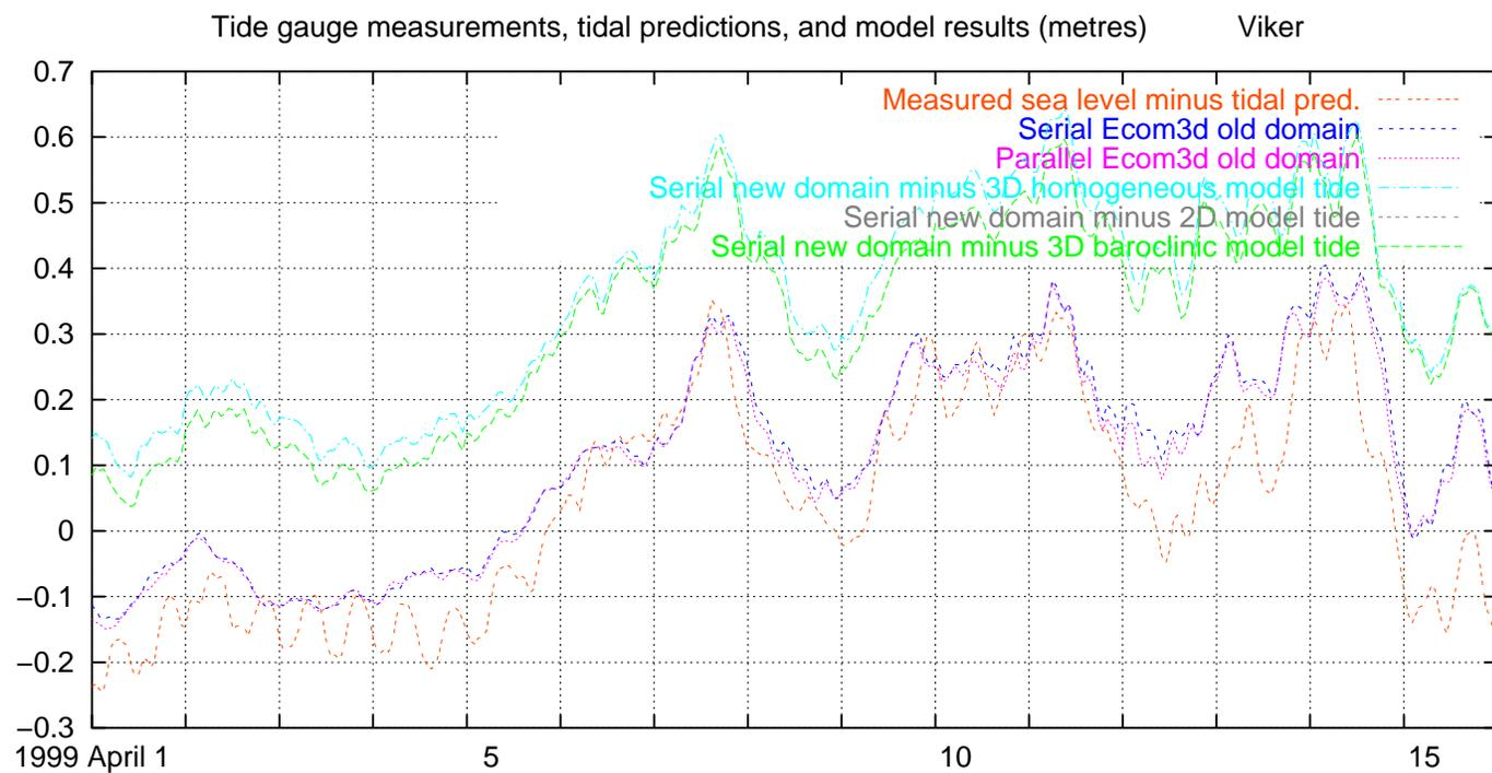
Fig. 25. Measured and modelled water level, excluding tides, Viker, 1999 April 1–15
