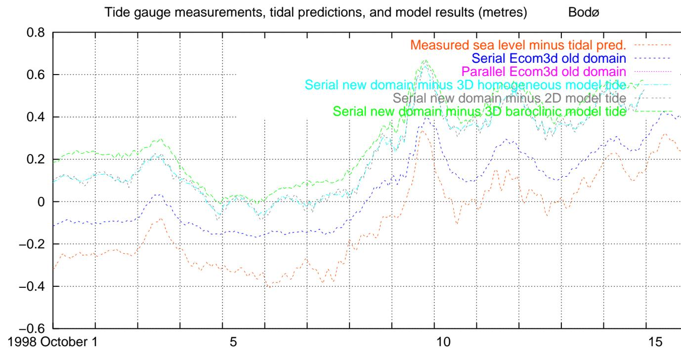
Fig. 63. Measured and modelled water level, excluding tides, Bodø, 1998 October 1–15
