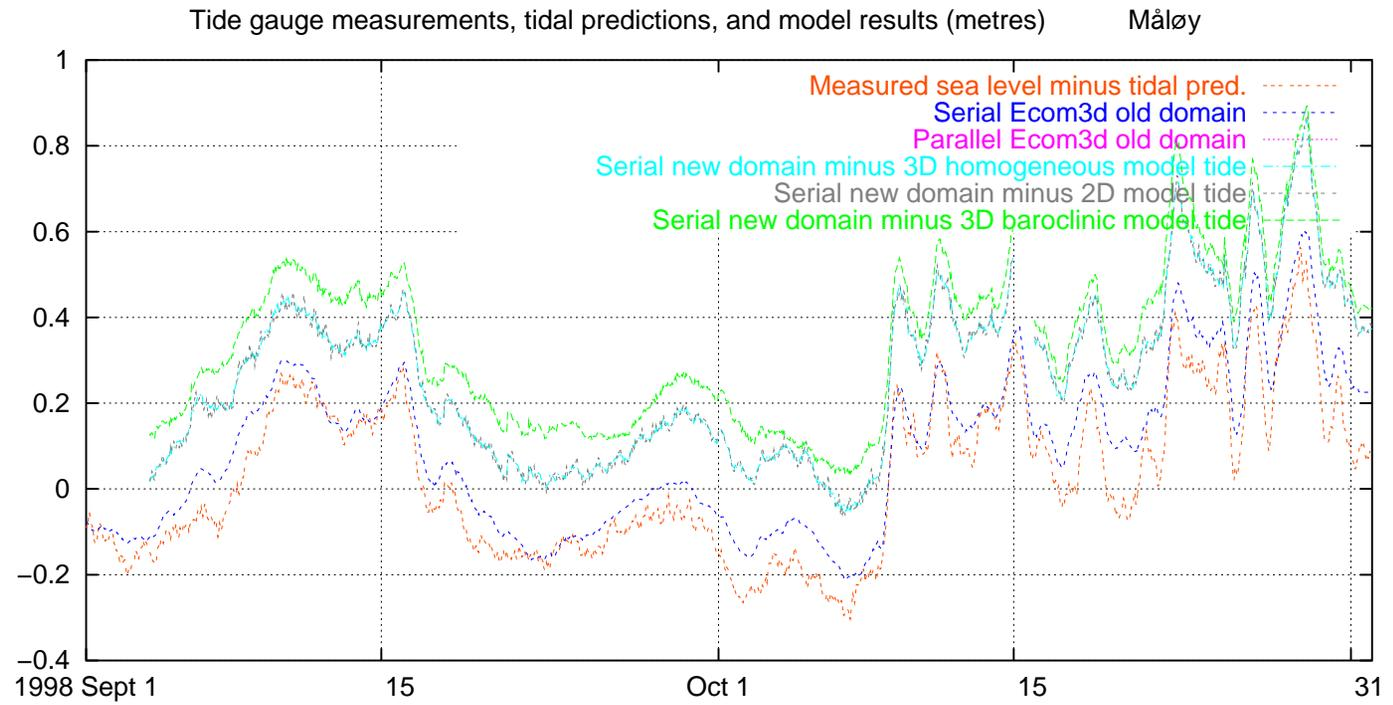
Fig. 42. Measured and modelled water level, excluding tides, Måløy, 1998 September–October
