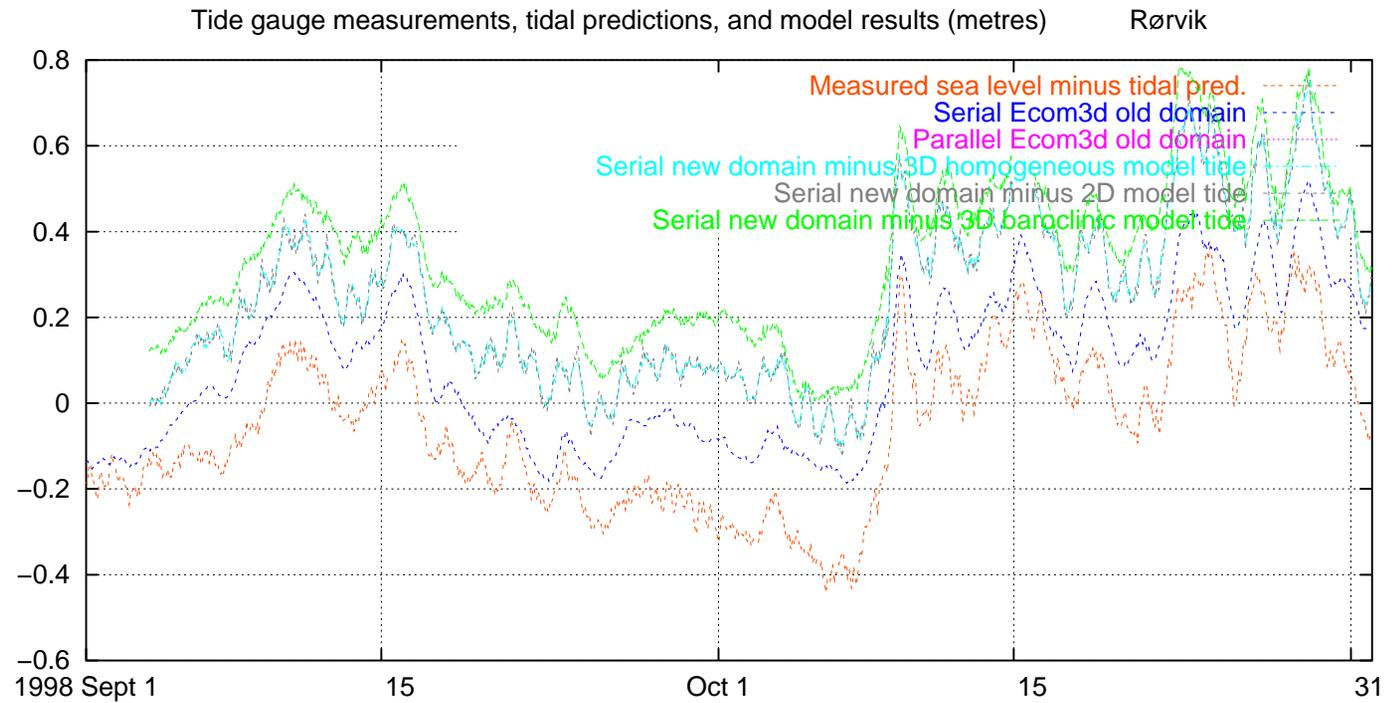
Fig. 58. Measured and modelled water level, excluding tides, Rørvik, 1998 September–October
