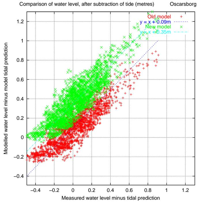
Fig. 5. Modelled v. measured water level for Oscarsborg
