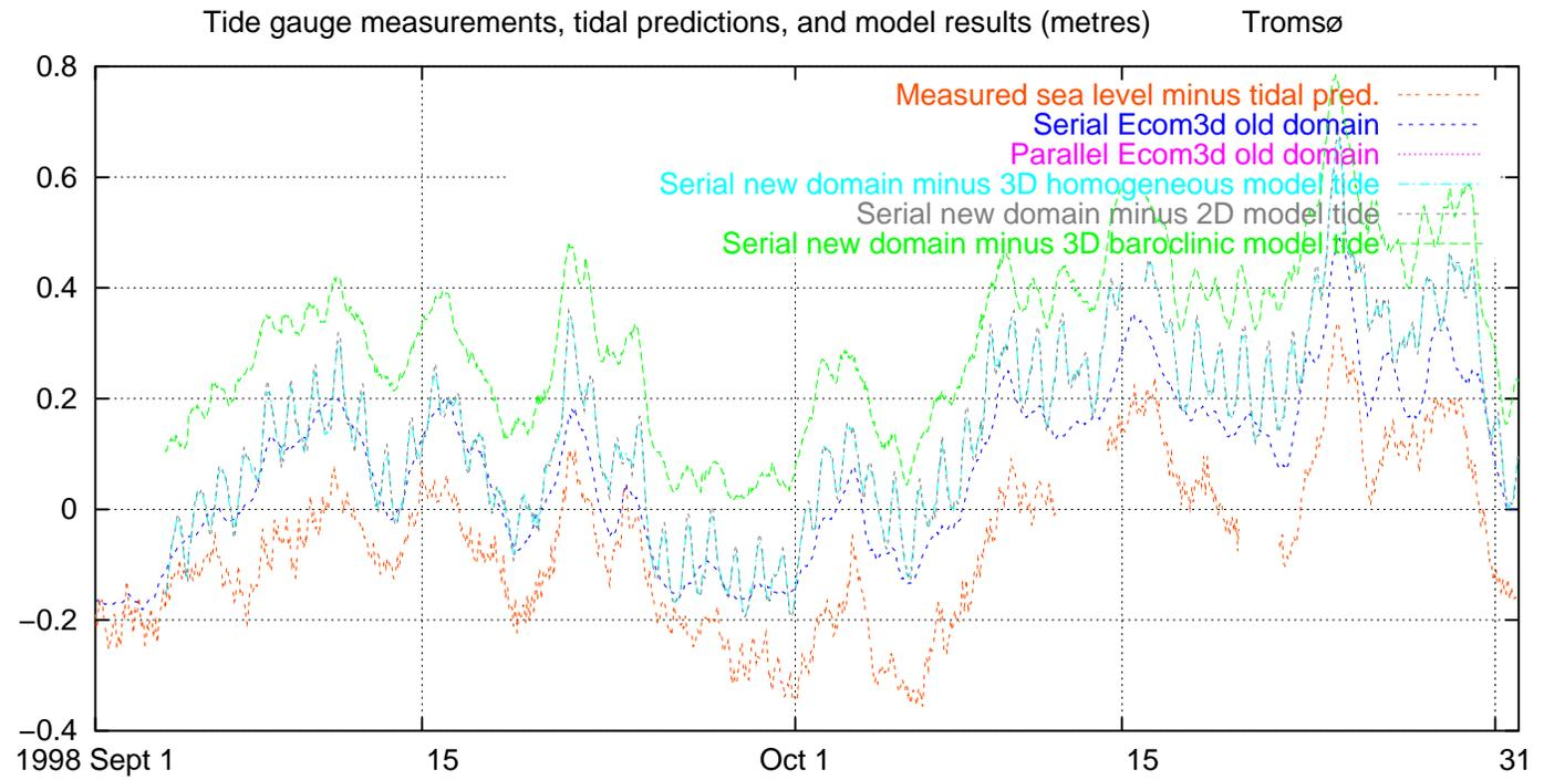
Fig. 82. Measured and modelled water level, excluding tides, Tromsø, 1998 September–October
