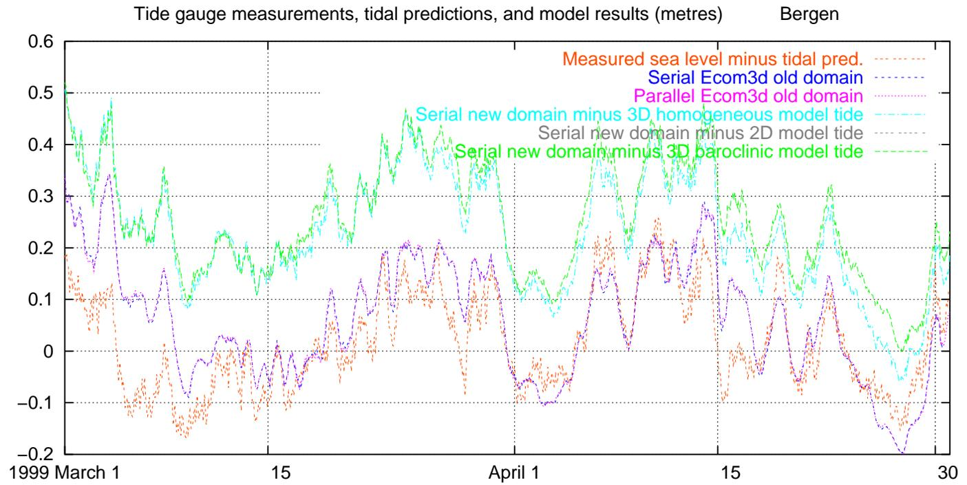
Fig. 40. Measured and modelled water level, excluding tides, Bergen, 1999 March–April
