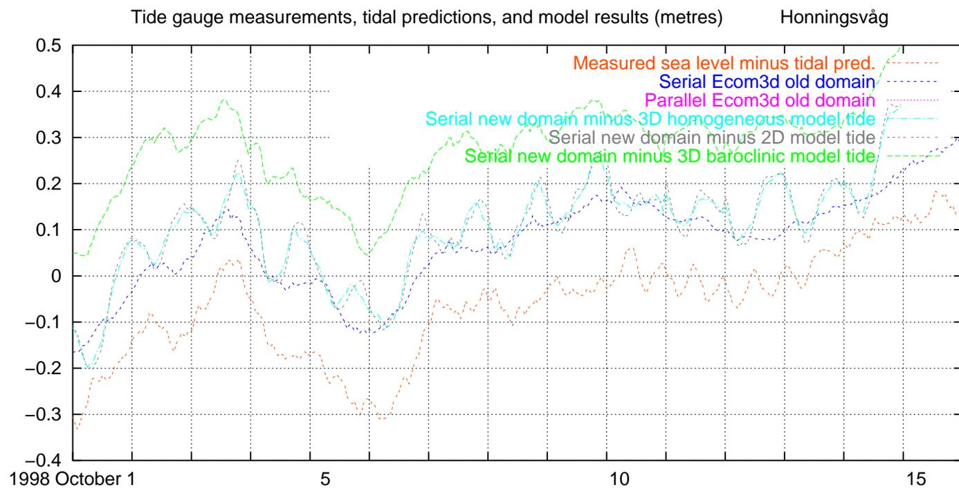
Fig. 91. Measured and modelled water level, excluding tides, Honningsvåg, 1998 October 1–15
