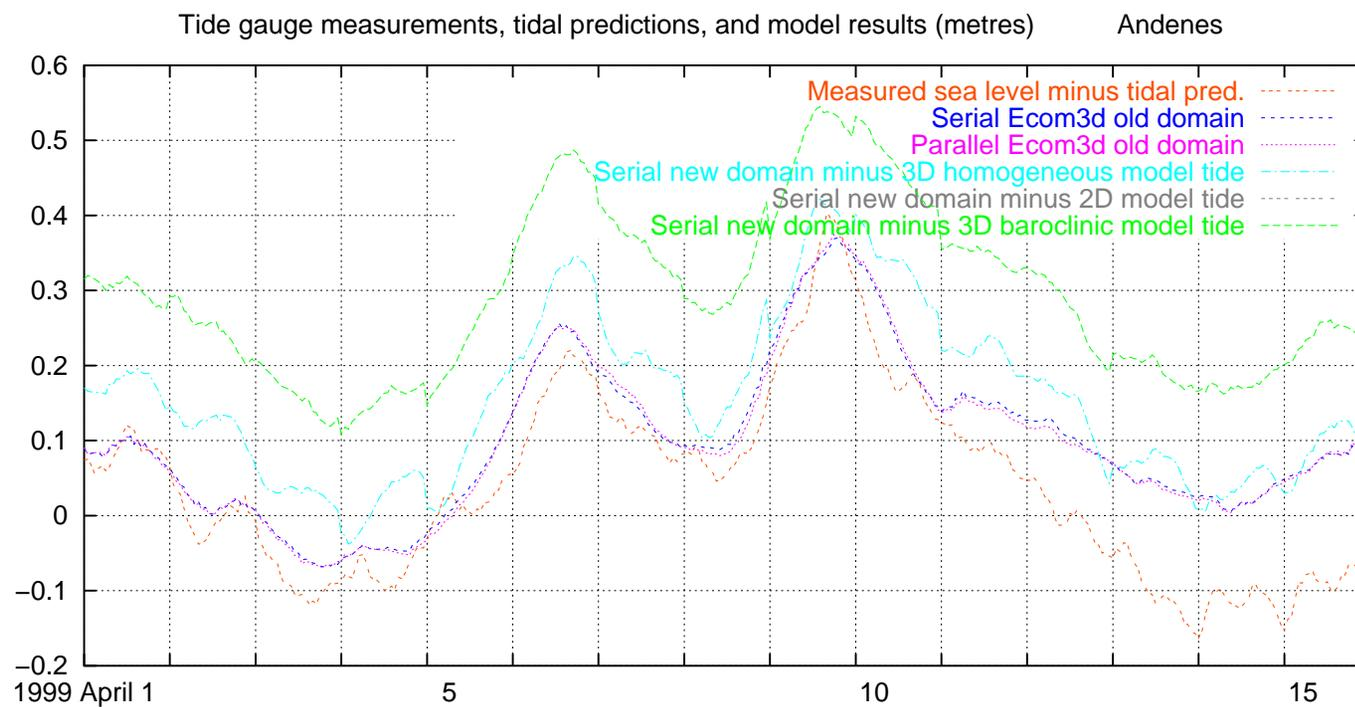
Fig. 81. Measured and modelled water level, excluding tides, Andenes, 1999 April 1–15
