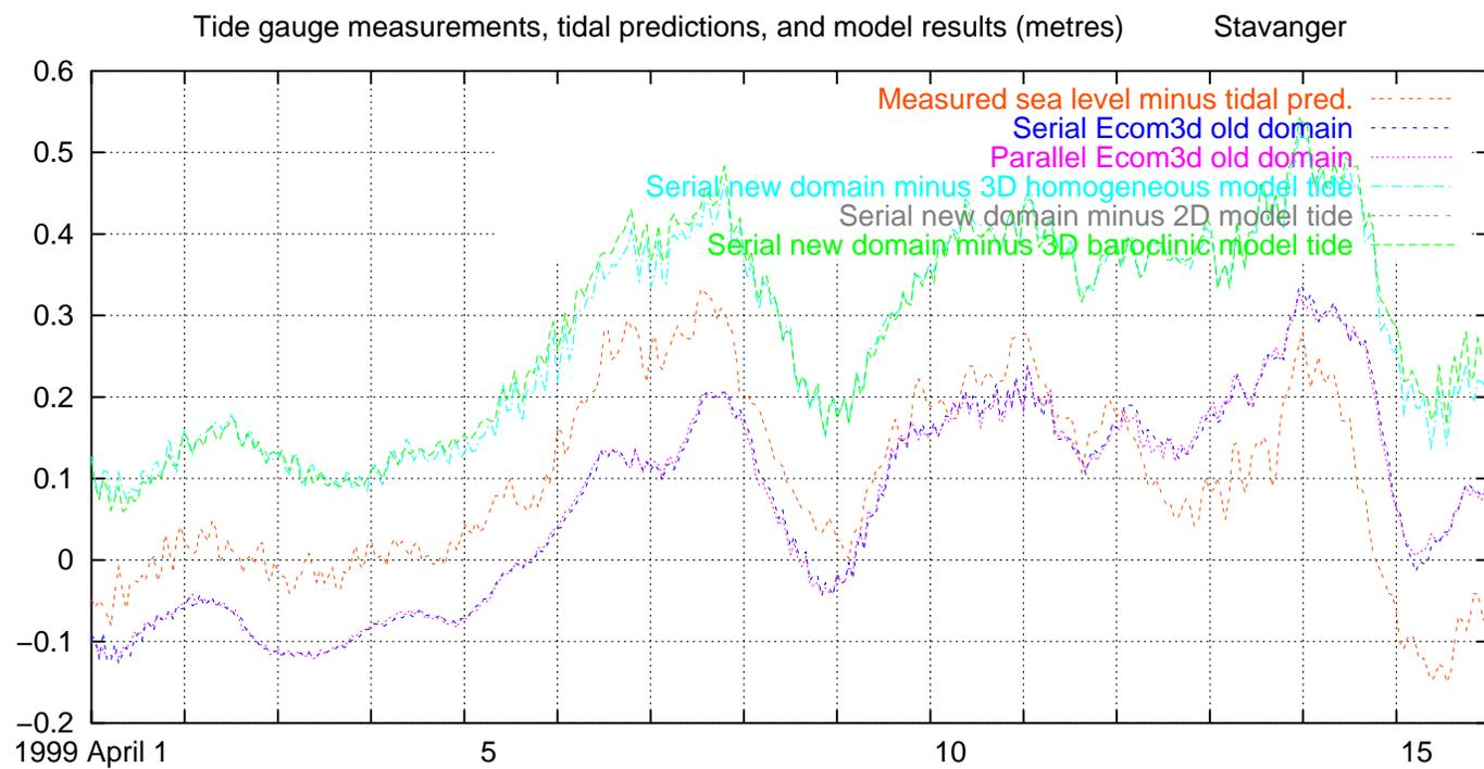
Fig. 37. Measured and modelled water level, excluding tides, Stavanger, 1999 April 1–15
