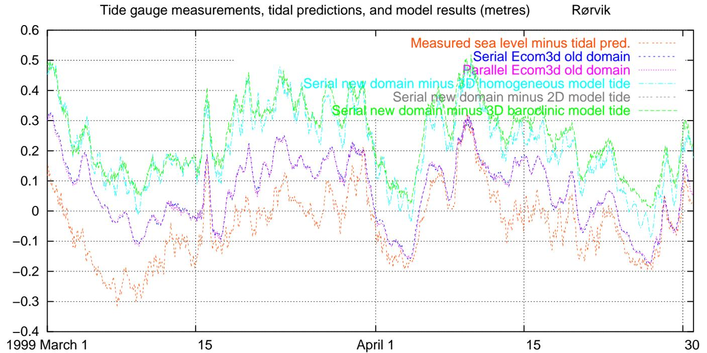
Fig. 60. Measured and modelled water level, excluding tides, Rørvik, 1999 March–April
