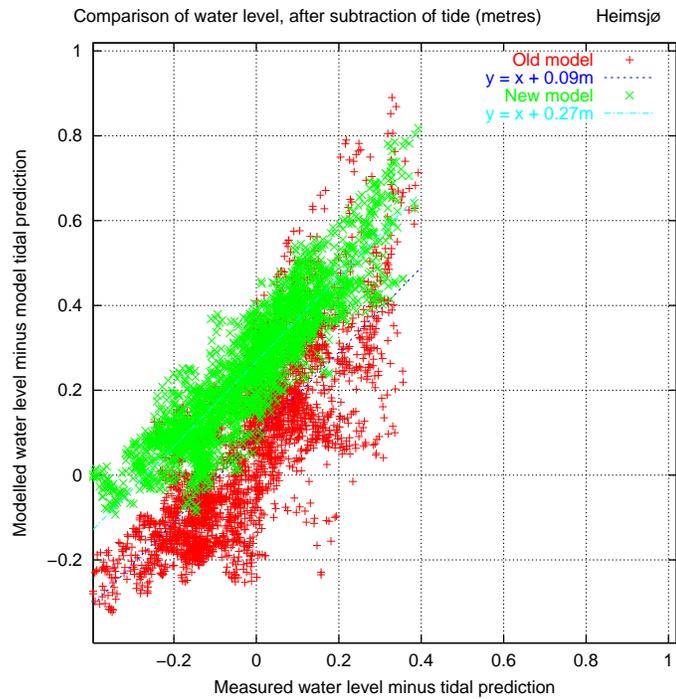
Fig. 12. Modelled v. measured water level for Heimsjø
