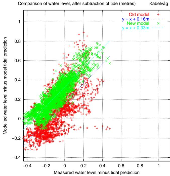
Fig. 15. Modelled v. measured water level for Kabelvåg
