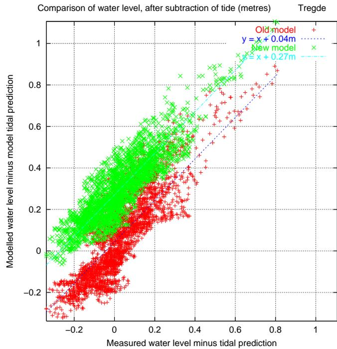
Fig. 6. Modelled v. measured water level for Tregde
