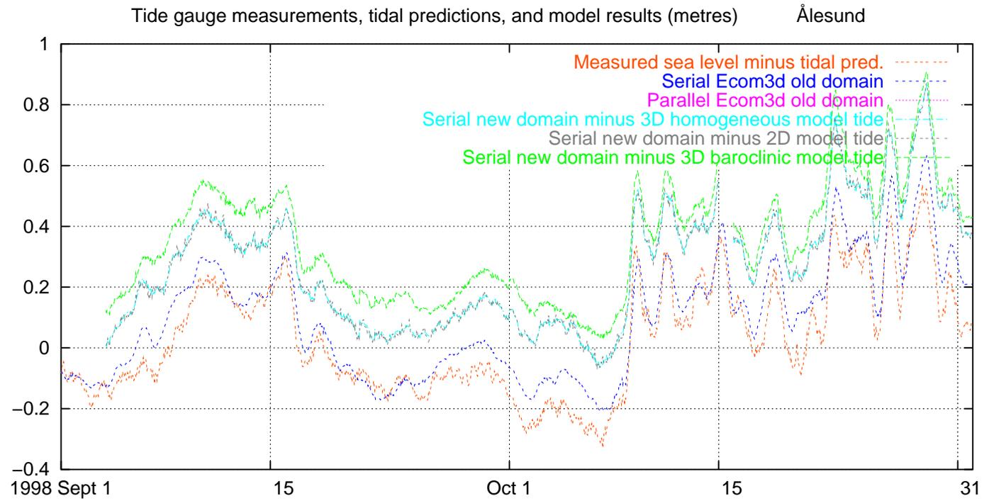
Fig. 46. Measured and modelled water level, excluding tides, Ålesund, 1998 September–October
