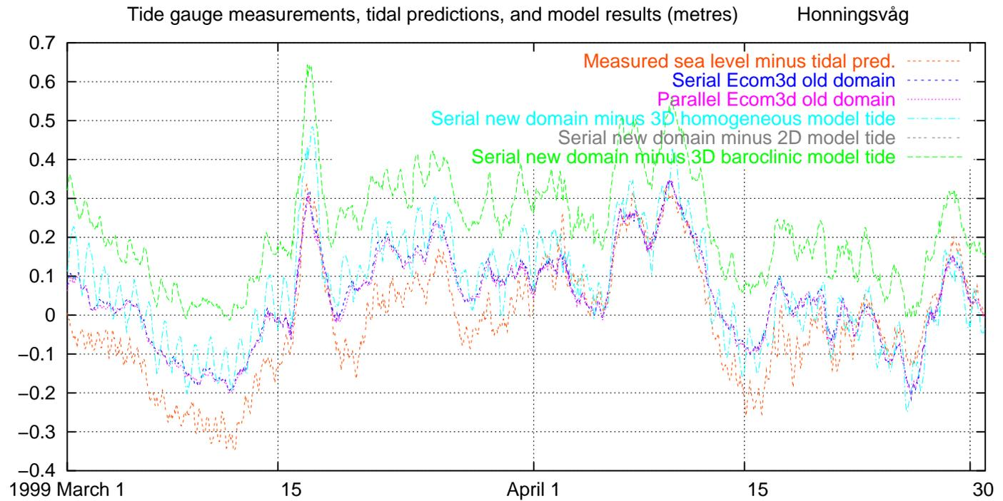
Fig. 92. Measured and modelled water level, excluding tides, Honningsvåg, 1999 March–April
