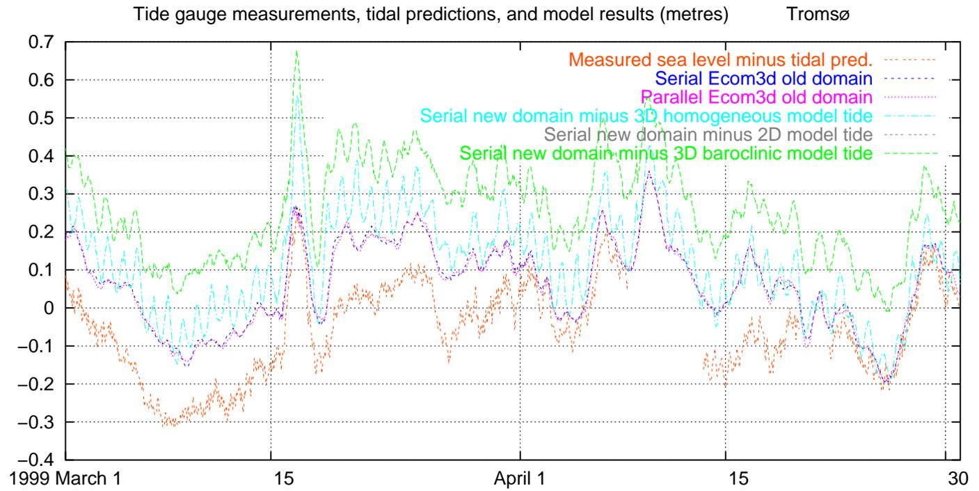
Fig. 84. Measured and modelled water level, excluding tides, Tromsø, 1999 March–April
