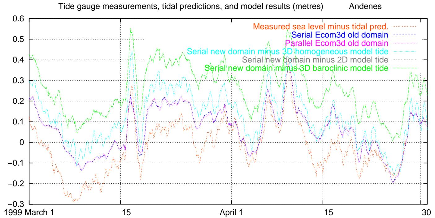
Fig. 80. Measured and modelled water level, excluding tides, Andenes, 1999 March–April
