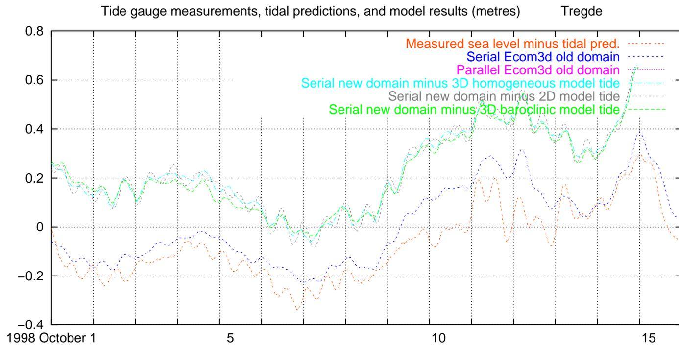
Fig. 31. Measured and modelled water level, excluding tides, Tregde, 1998 October 1–15
