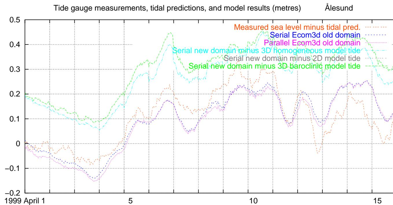
Fig. 49. Measured and modelled water level, excluding tides, Ålesund, 1999 April 1–15
