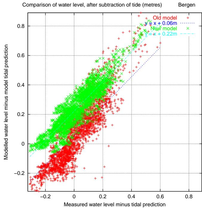
Fig. 8. Modelled v. measured water level for Bergen
