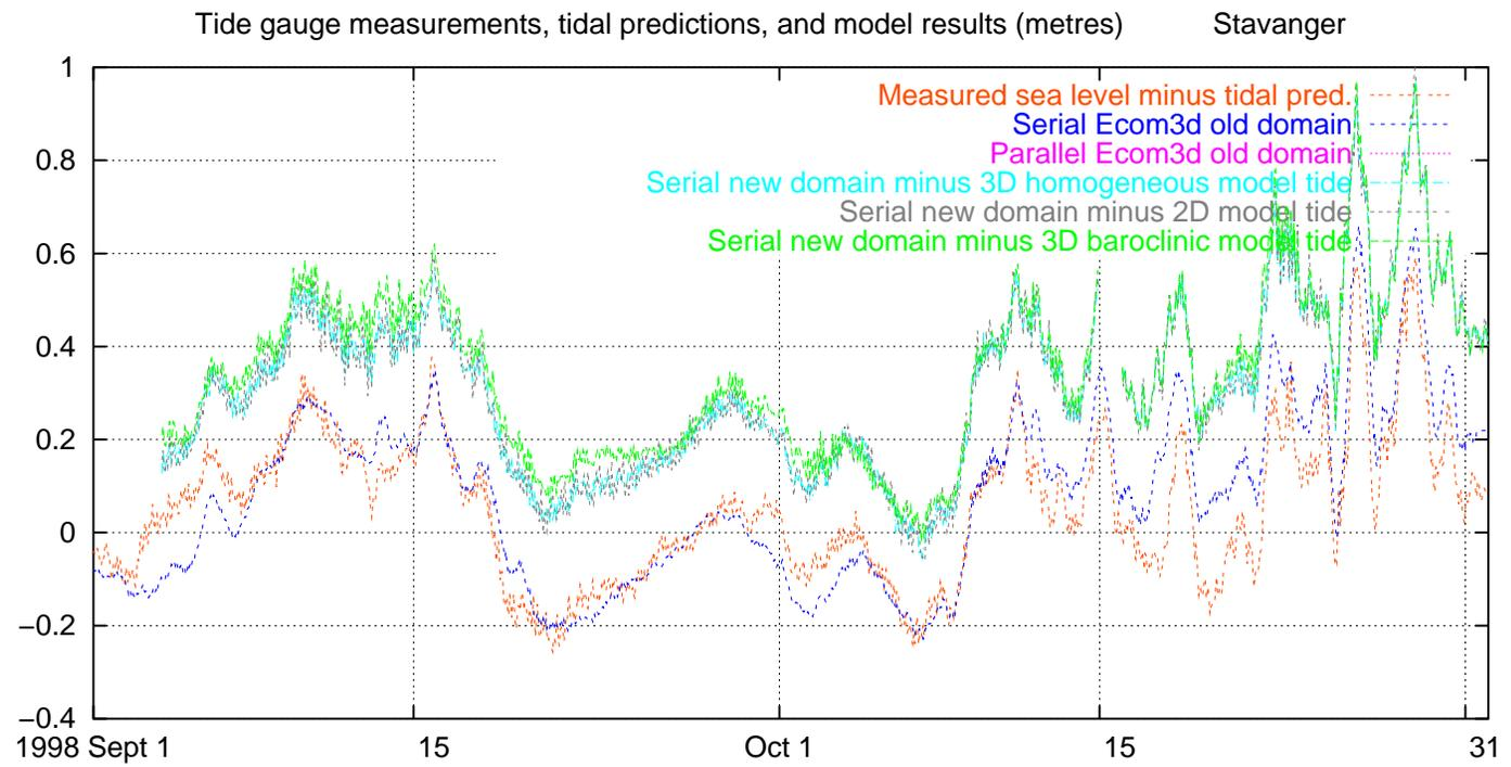
Fig. 34. Measured and modelled water level, excluding tides, Stavanger, 1998 September–October
