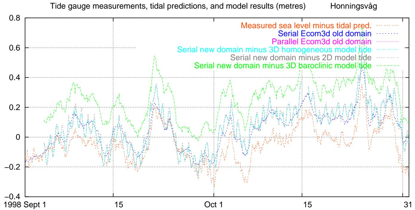
Fig. 90. Measured and modelled water level, excluding tides, Honningsvåg, 1998 September–October
