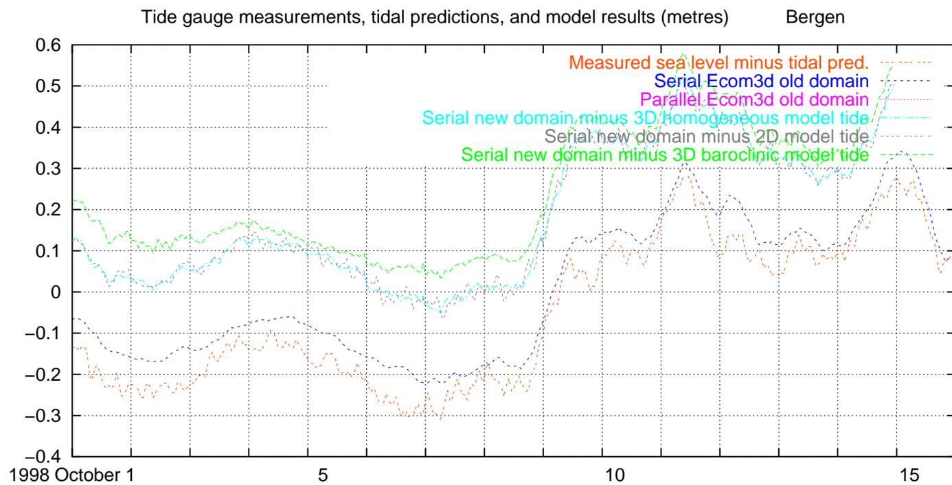
Fig. 39. Measured and modelled water level, excluding tides, Bergen, 1998 October 1–15
