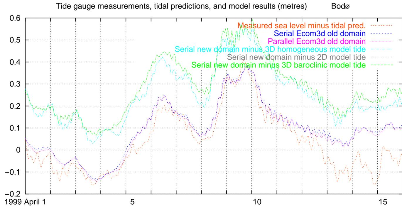
Fig. 65. Measured and modelled water level, excluding tides, Bodø, 1999 April 1–15
