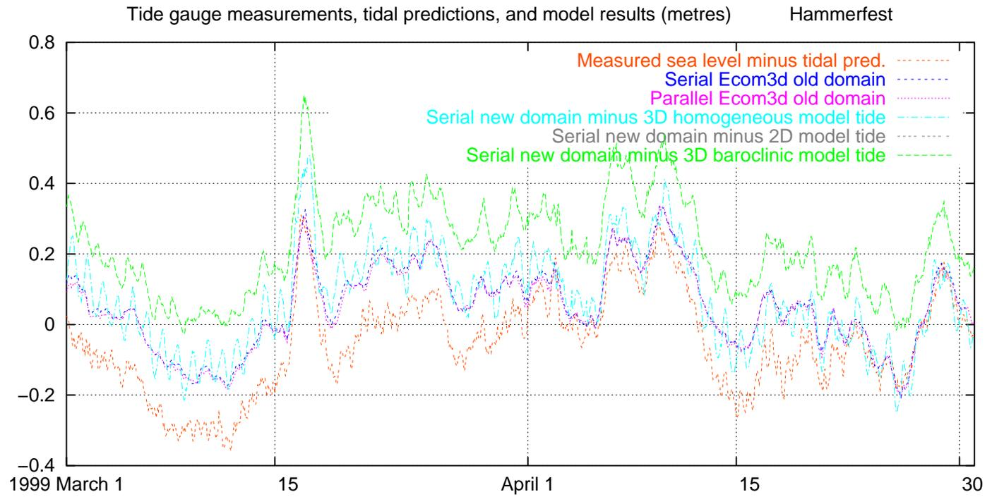
Fig. 88. Measured and modelled water level, excluding tides, Hammerfest, 1999 March–April
