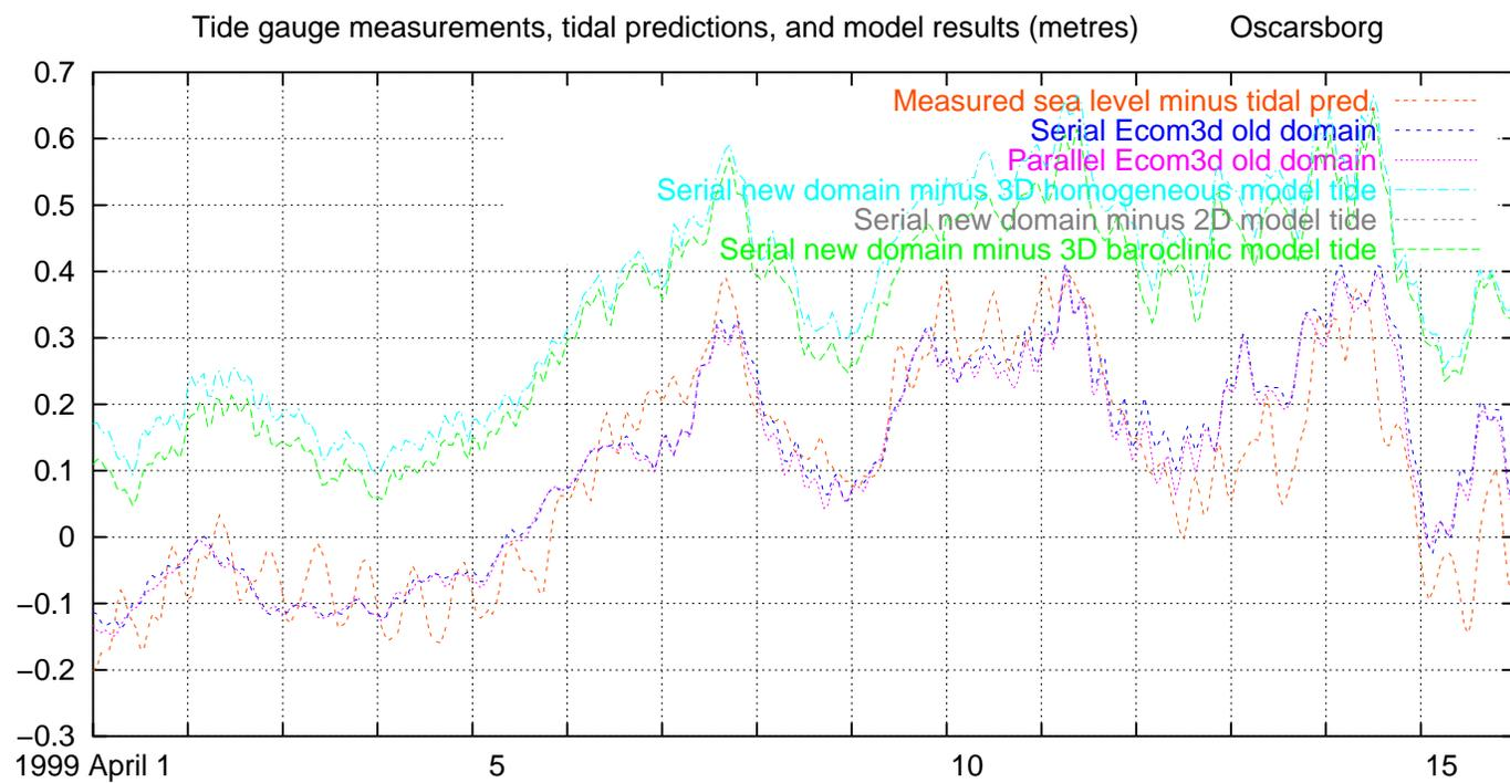
Fig. 29. Measured and modelled water level, excluding tides, Oscarsborg, 1999 April 1–15
