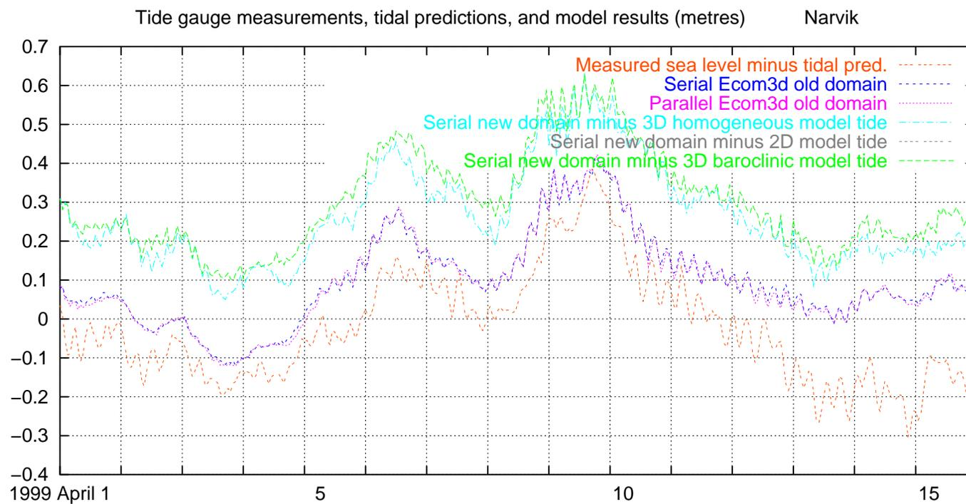
Fig. 73. Measured and modelled water level, excluding tides, Narvik, 1999 April 1–15
