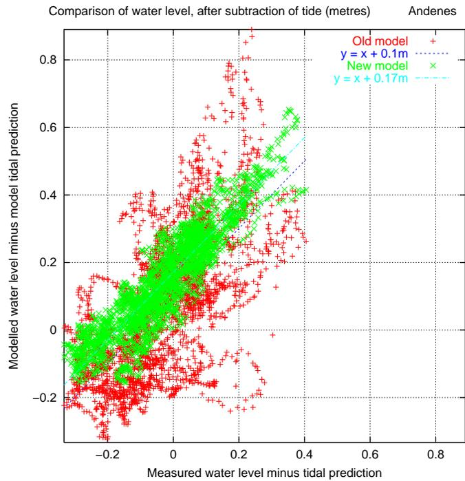
Fig. 18. Modelled v. measured water level for Andenes
