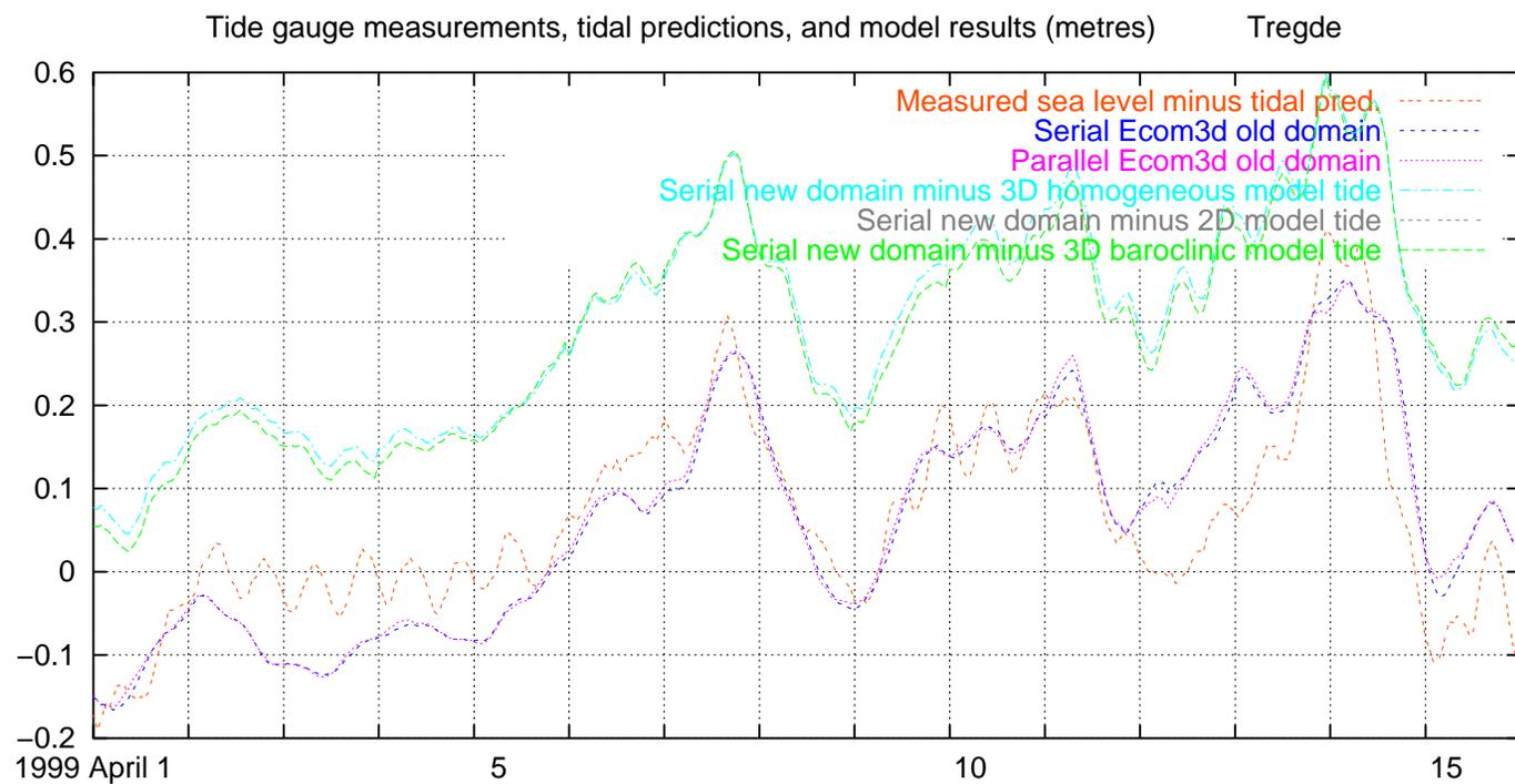
Fig. 33. Measured and modelled water level, excluding tides, Tregde, 1999 April 1–15
