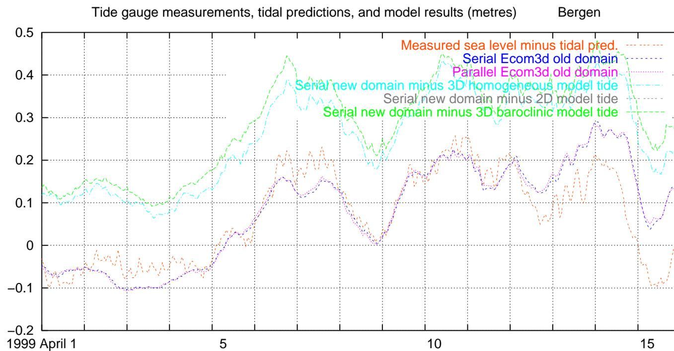
Fig. 41. Measured and modelled water level, excluding tides, Bergen, 1999 April 1–15
