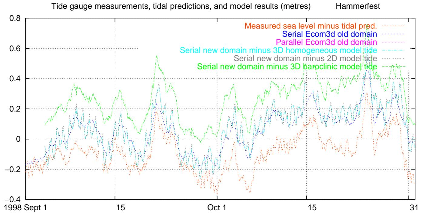
Fig. 86. Measured and modelled water level, excluding tides, Hammerfest, 1998 September–October
