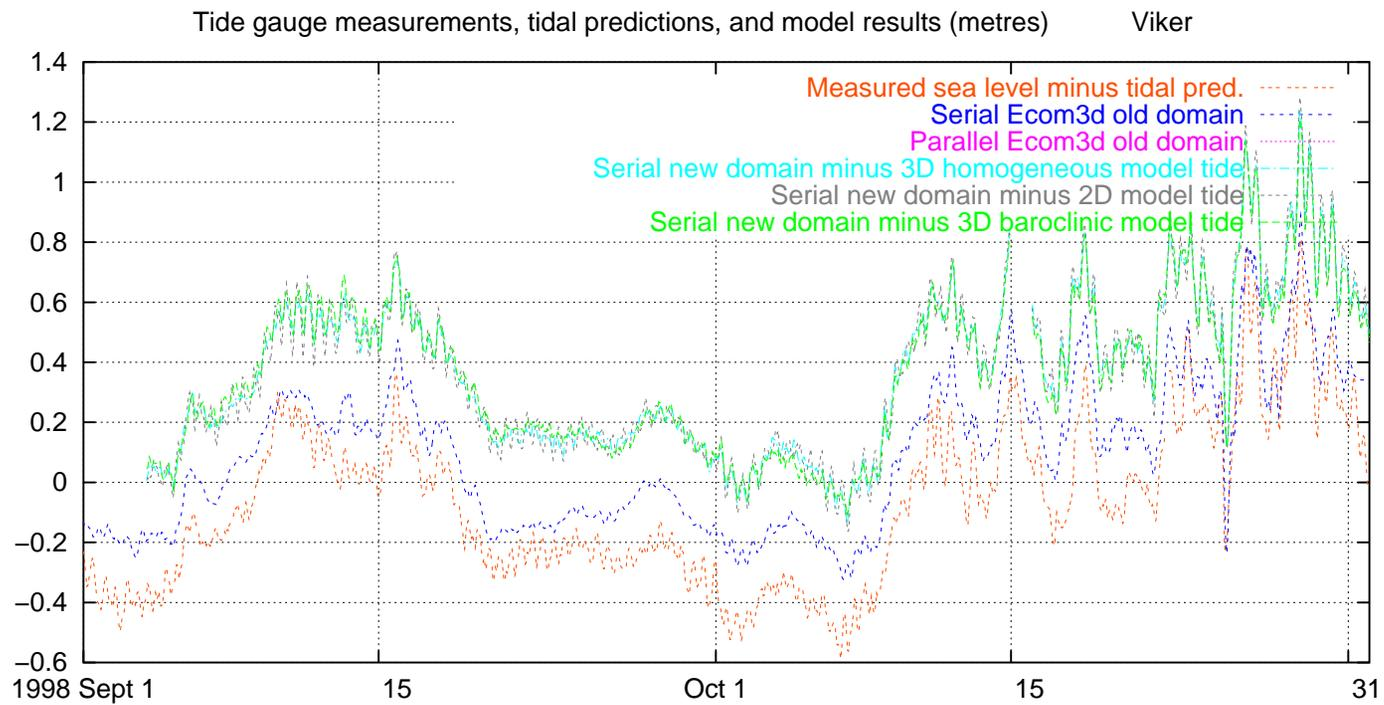
Fig. 22. Measured and modelled water level, excluding tides, Viker, 1998 September–October
