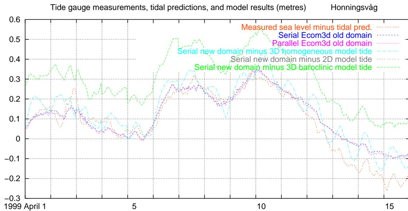
Fig. 93. Measured and modelled water level, excluding tides, Honningsvåg, 1999 April 1–15
