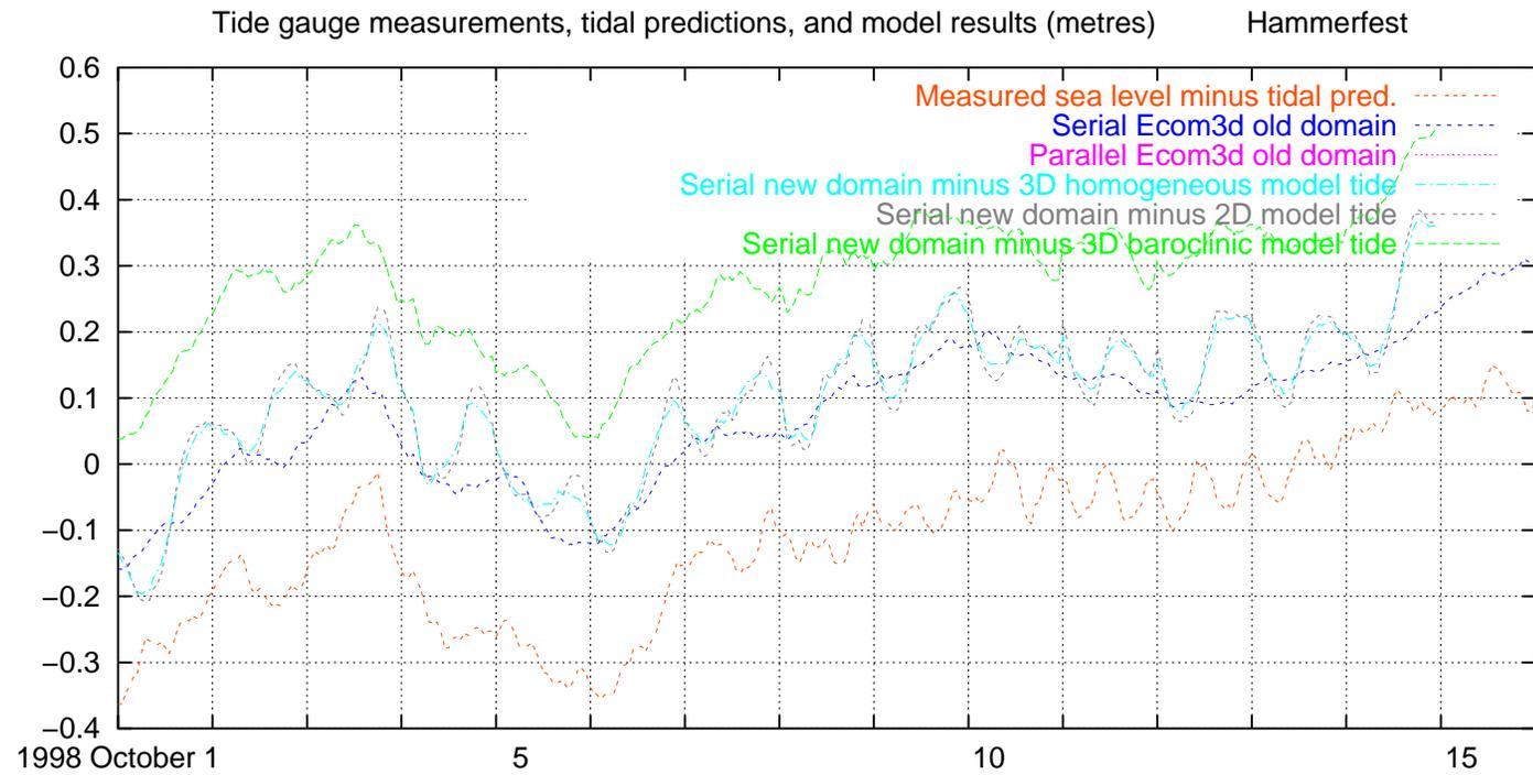
Fig. 87. Measured and modelled water level, excluding tides, Hammerfest, 1998 October 1–15
