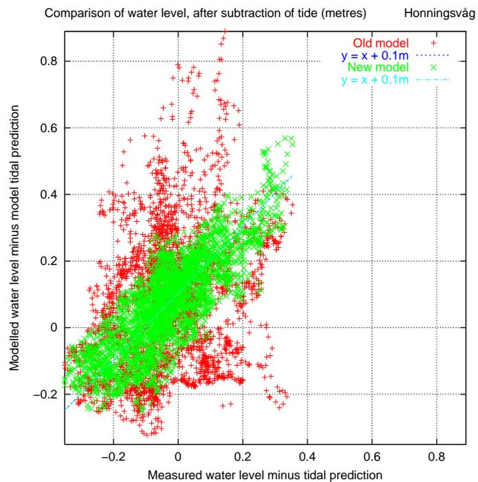
Fig. 21. Modelled v. measured water level for Honningsvåg
