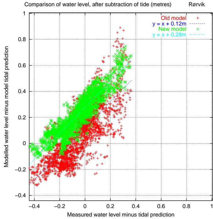
Fig. 13. Modelled v. measured water level for Rørvik
