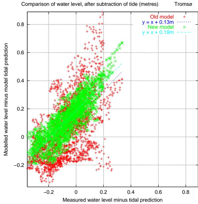
Fig. 19. Modelled v. measured water level for Tromsø
