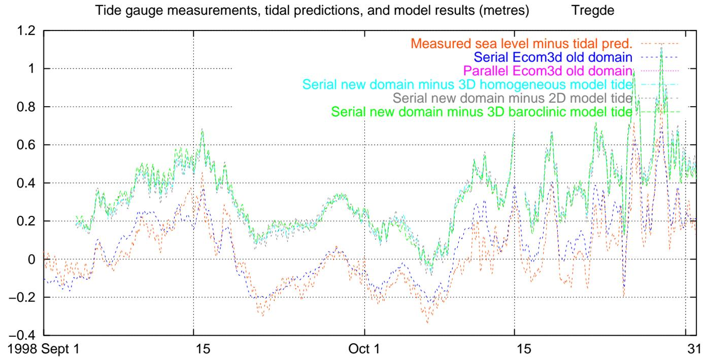
Fig. 30. Measured and modelled water level, excluding tides, Tregde, 1998 September–October
