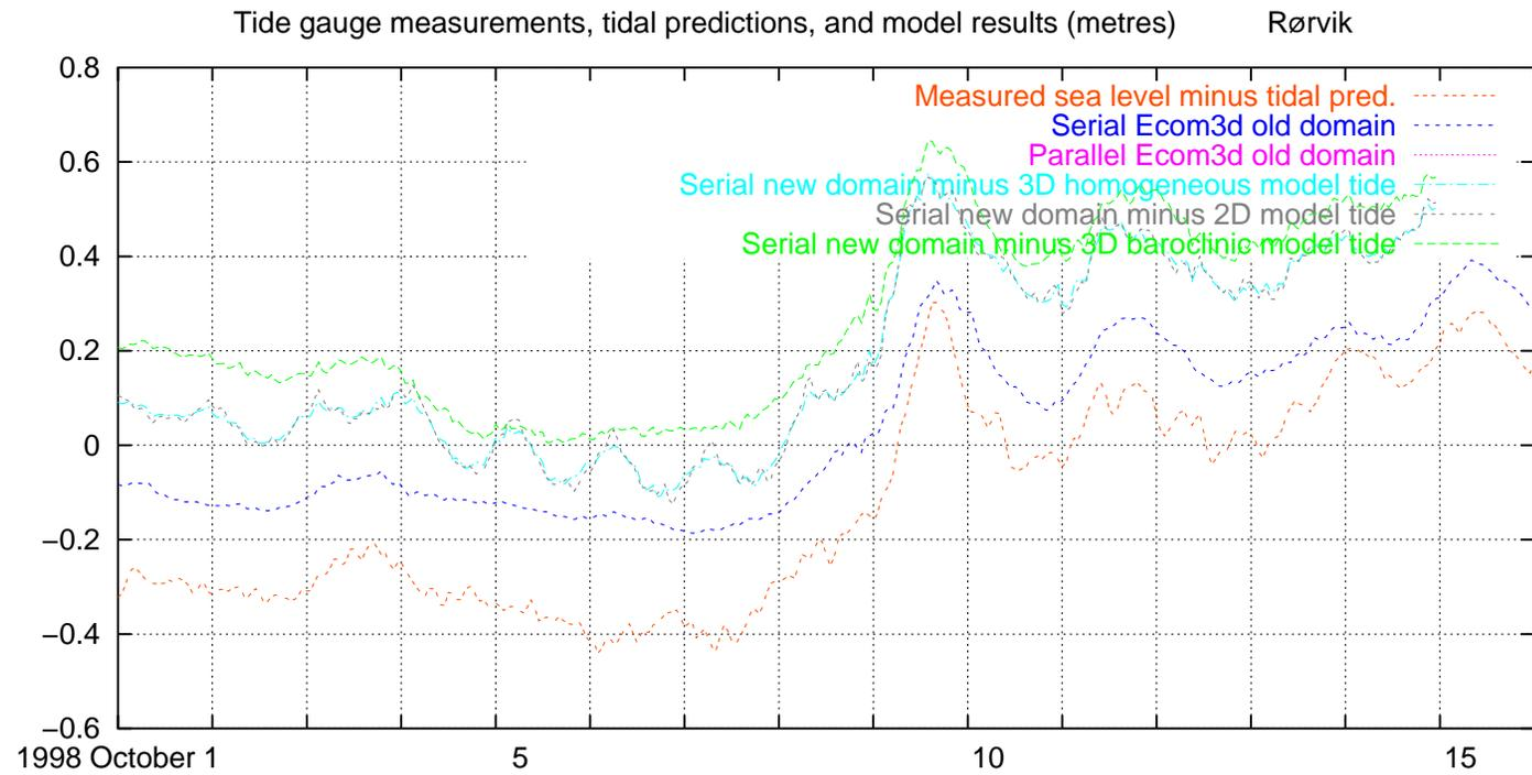
Fig. 59. Measured and modelled water level, excluding tides, Rørvik, 1998 October 1–15
