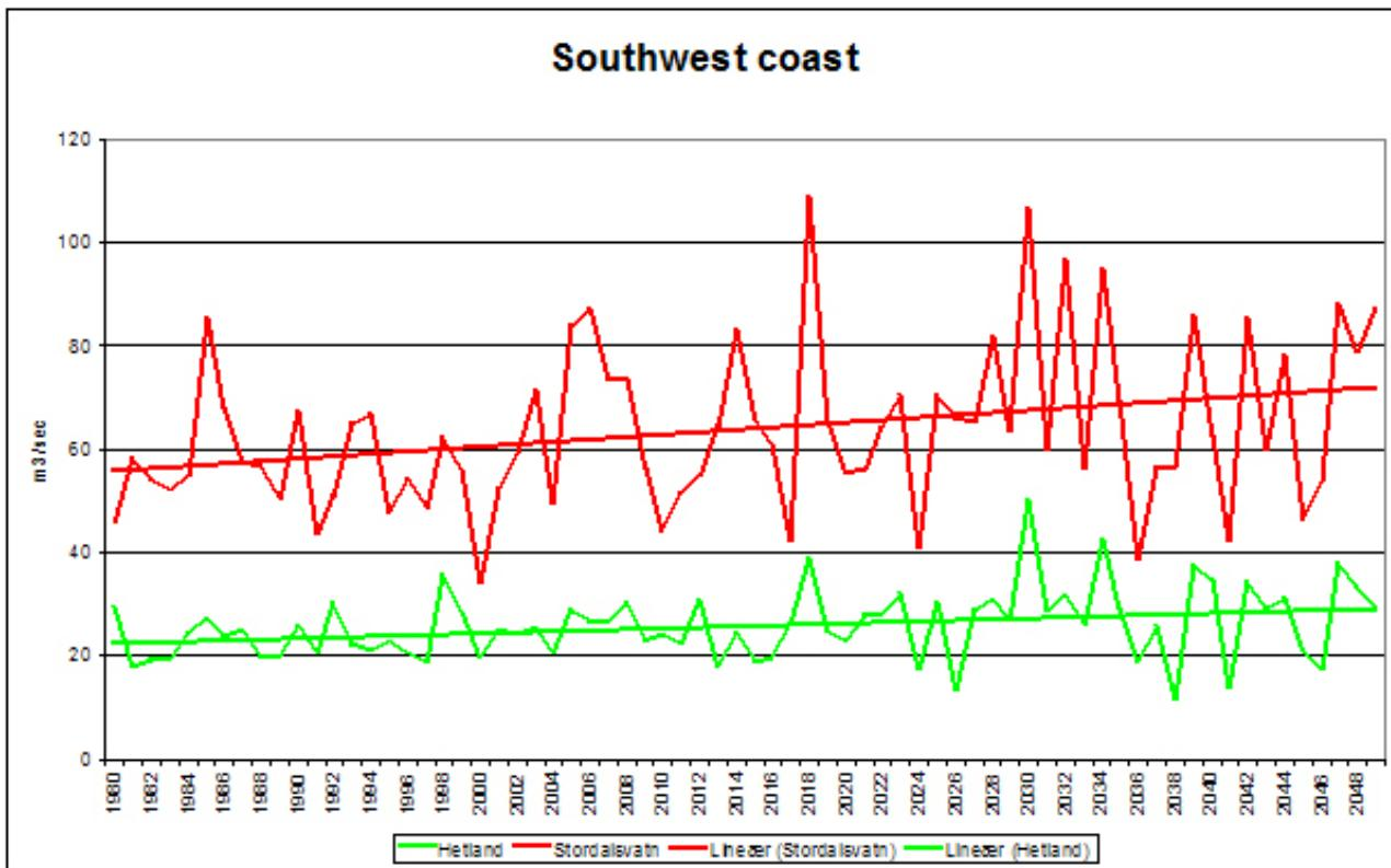
Figure 3.12 Variability of the annual flood in basins at the southwest coast of Norway based on a transient run 1980–2049 of the hydrological model driven by the ECHAM4/OPYC3 model, the IS92A emission scenario and downscaling by the HIRHAM model.
