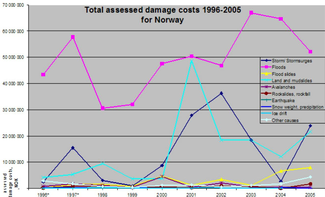
Figure 10.5 Overview of total assessed damage costs for the various categories of natural hazard, 1996-2005.
