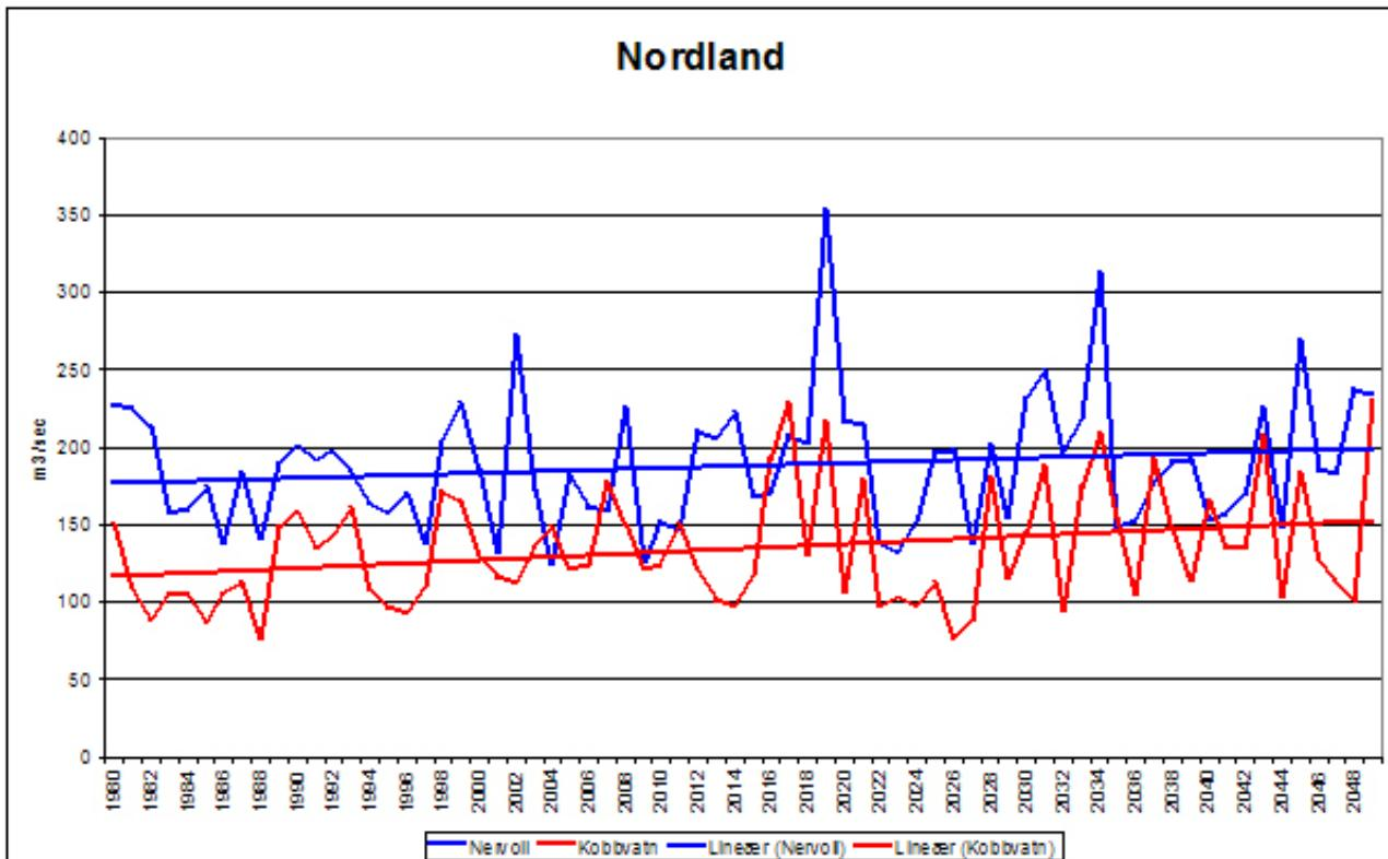
Figure 3.13 Variability of the annual flood in basins in Nordland based on a transient run 1980–2049 of the hydrological model driven by the ECHAM4/OPYC3 model, the IS92A emission scenario and downscaling by the HIRHAM model.
