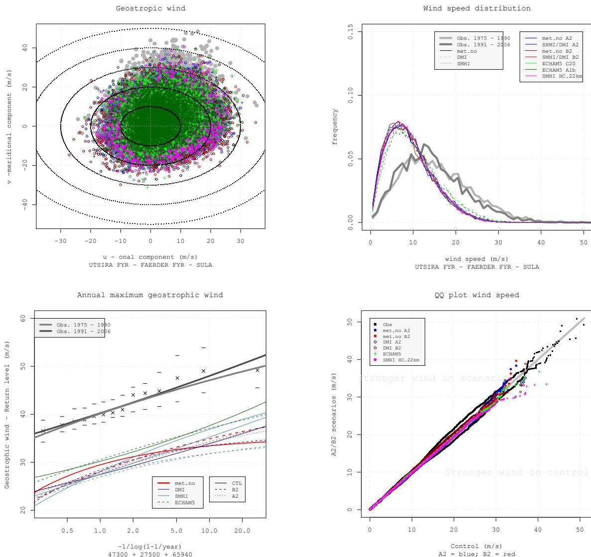
**Figure 5.4** Geostrophic wind analysis for various RCMs/GCMs (CTL and scenarios) estimated for a triangle over southern Norway. (a): scatter of the north-south and east-west wind components (positive values: west-to-east, and south-to-north); (b) distribution of wind speeds; (c) return-value analysis; and (d) quantile-quantile plots.
