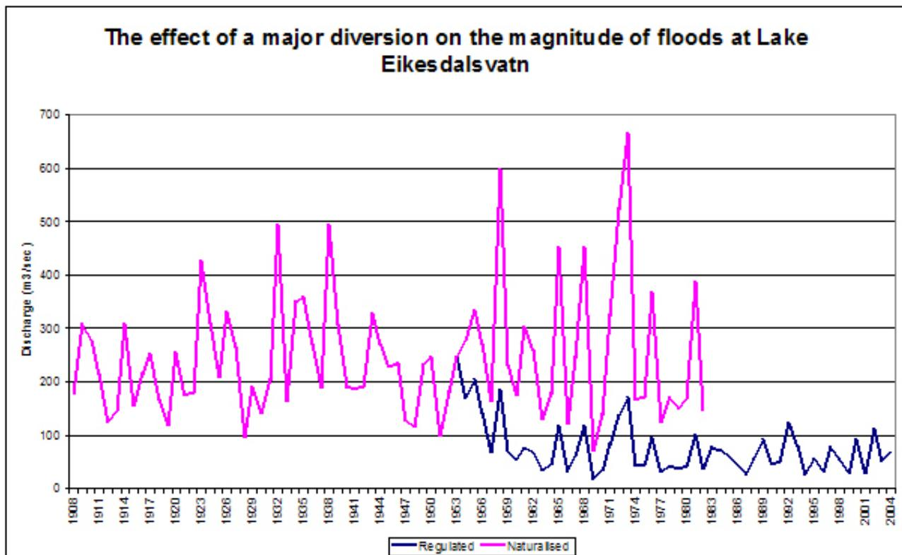
*Figure 3.6 Annual floods at the outlet of Lake Eikesdalsvatn in River Eira. A major part of the basin was diverted to the neighbour river from 1953, and the outflow is released from the power station there close to the sea. The naturalised flood series was calculated by adding the discharge used for hydropower production to the observed regulated flow series and correcting for the varying volume of the reservoir.*
