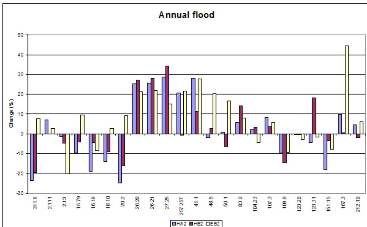
Figure 3.15 Projected change in the 50-year return period annual flood in 23 basins in Norway. Basin no 311.6–2.111 are in East Norway, 2.13 and 109.9 are mountainous basins, 15.79–26.21 are in the southernmost part of Norway, 27.26–83.4 West Norway, 104.23–123.31 Mid Norway, 151.15–167.3 North Norway and 212.10 Finnmarksvidda plateau.
