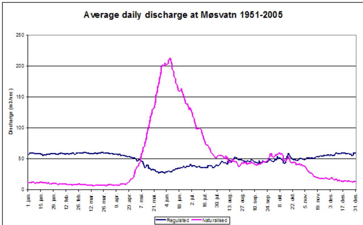
Figure 3.7 Large reservoirs can lead to a total redistribution of the regulated discharge over the year as shown for the Møsvatn reservoir where average daily values of regulated and naturalised discharge is shown for the period 1951–2004.
