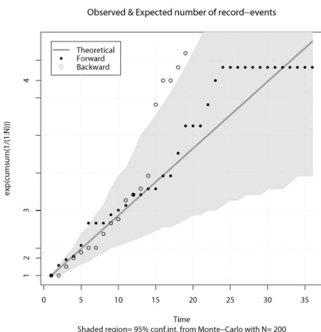
**Figure 5.13** Record-value analysis for the annual maximum wind speed (data from Knut Harstveit). The upper panels show the timing of new record-breaking events for forward as well as backward analysis, whereas the lower panels show the average number of record-events as a function of time. Left: the analysis for a few long series; right: the analysis for many shorter series.
