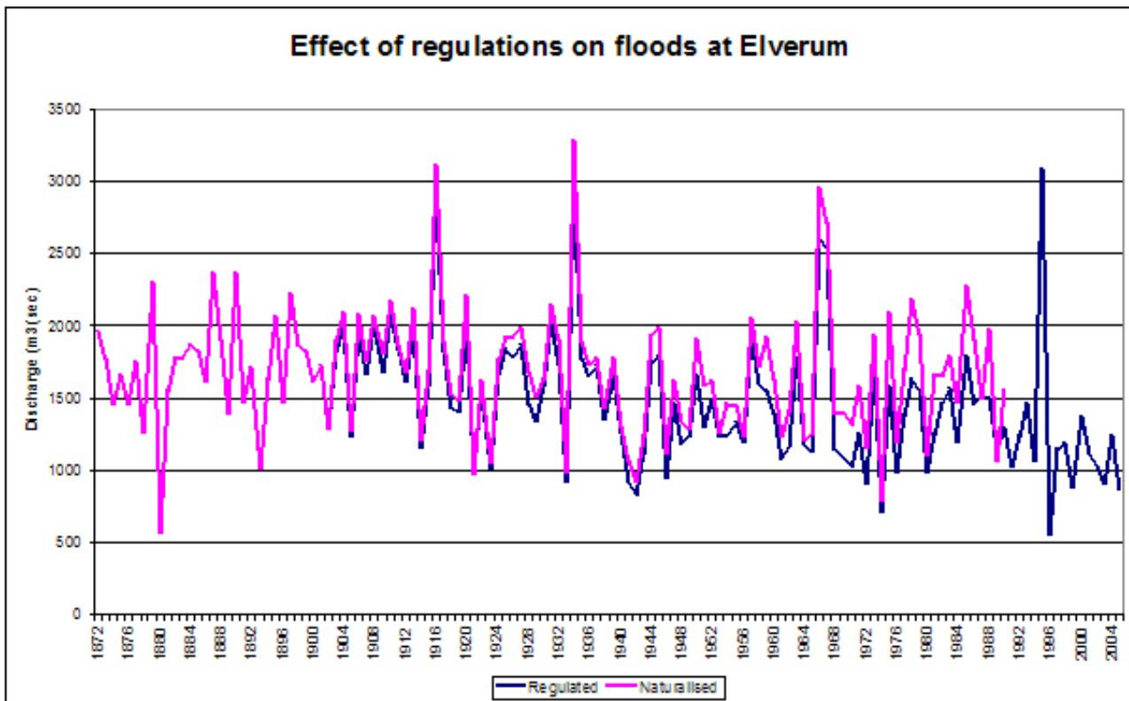
*Figure 3.8 Regulated and naturalised annual floods in River Glomma at Elverum. The degree of regulation is fairly low in the eastern branch of the river, but the 1995 flood would have exceeded Storofsen, if there had been no upstream reservoirs and preventive operation of the hydropower system as in 1789 (Tingvold 1996).*
