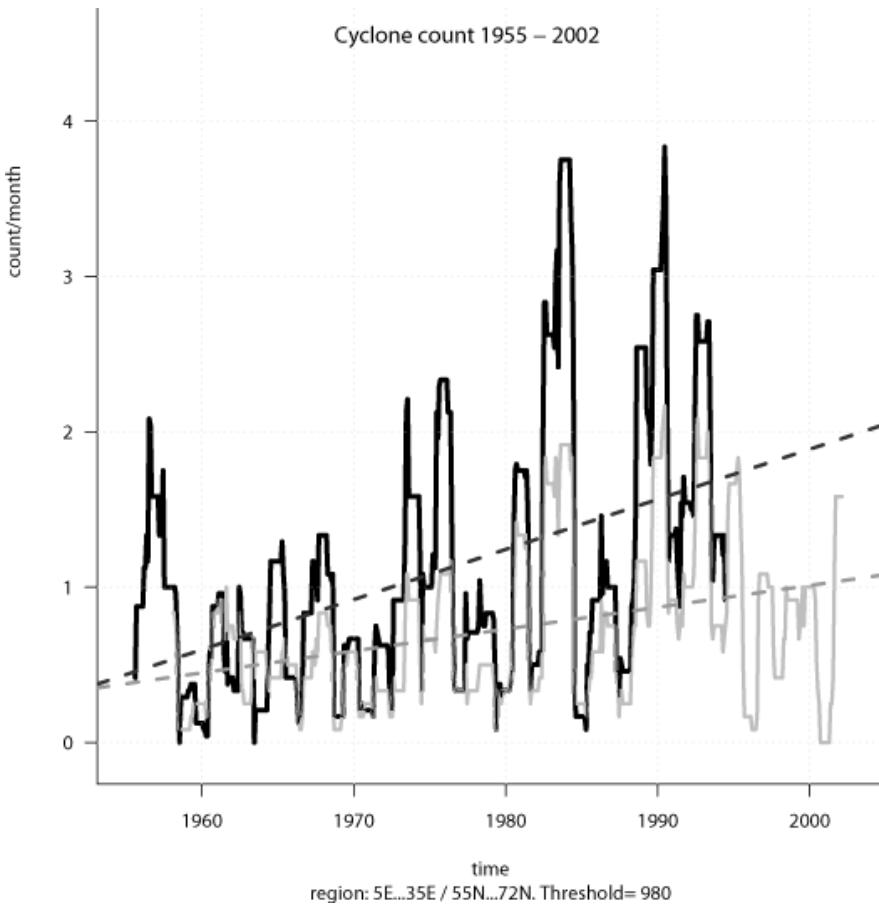
**Figure 5.6** Time series showing the time evolution of the number of low-pressure systems with central pressure lower than 980 hPa in the region 5 °E – 35 °E / 55 °N – 72 °N analysed from the ERA40 (grey) and NMC (black) gridded sea level pressure data.
