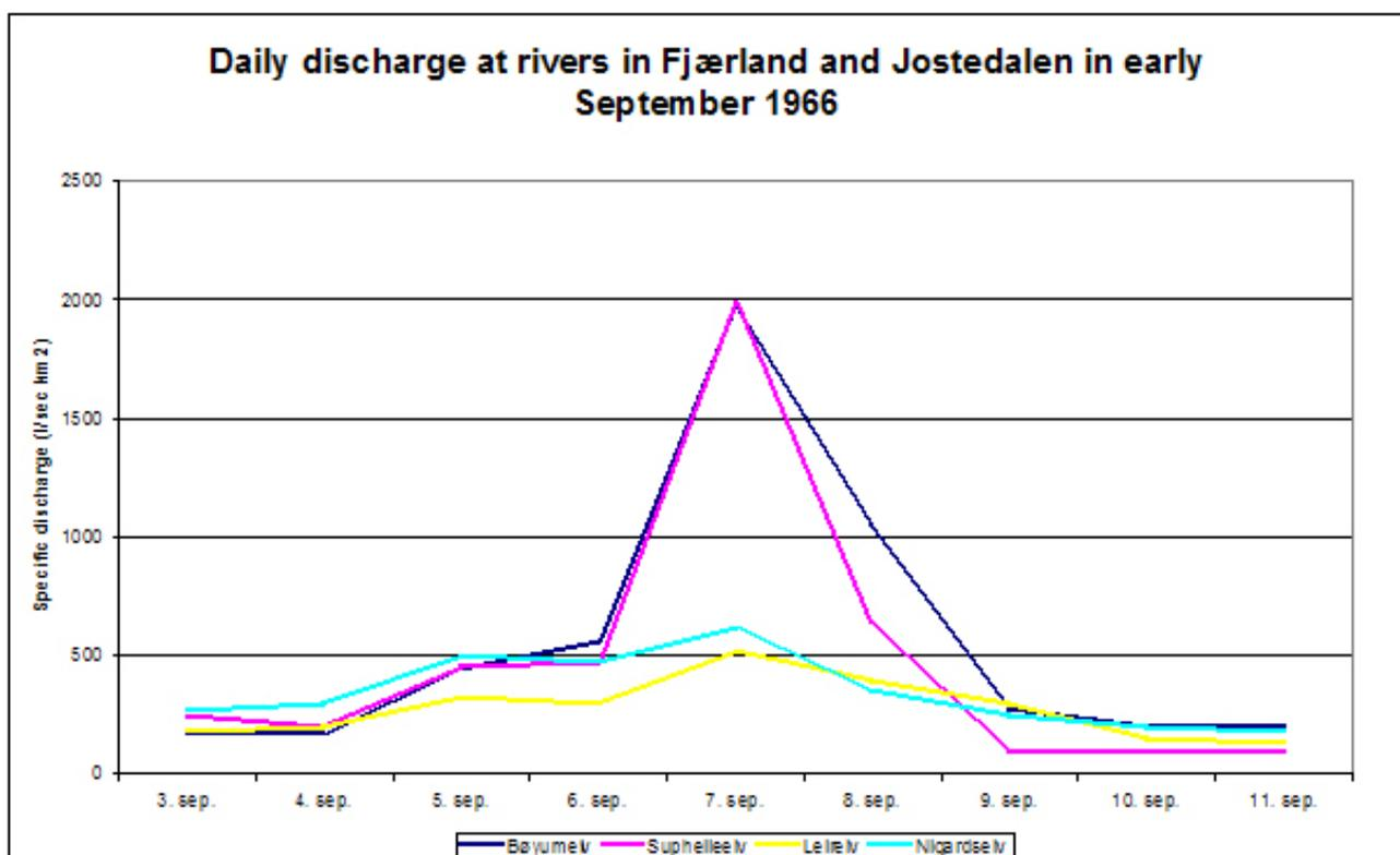
Figure 3.3 Observed flood at Fjærland caused by the remnants of tropical hurricane Faith 7<sup>th</sup> September 1966.
