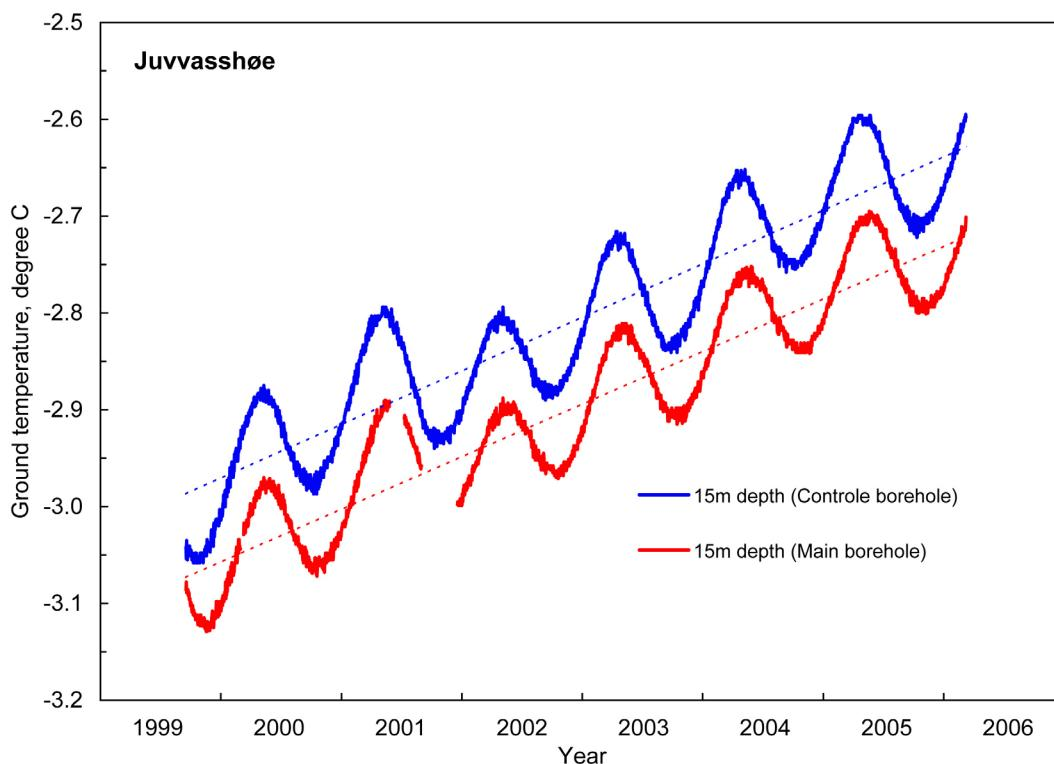
15 m depth. The time-series suggest that permafrost is warming at a significant rate. Results show that the ground temperature has increased by 0.2 °C at 25 m depth and increased by 0.1 °C at 30 m depth. Observed warming is statistically significant to 60 m depth. This result strongly supports the previous interpretation by Isaksen et al. (2001) that most of the anomalies observed in the temperature depth profiles (cf. Figure 8.2) are associated with surface warming.
