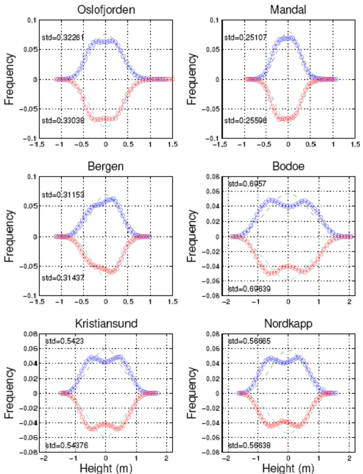
**Figure 6.1** Bi-histograms of SLH at six locations along the Norwegian coast. The lower curves correspond to the period 1980–1999 and the upper curves to the period 2030–2049. The histograms were constructed from hourly height data, from the Regclim MPI-GSDIO simulation. The curves are superimposed on Gaussian curves with the same standard deviations. The probability, from the Kolmogorov-Smirnov statistic, that the future and present histograms are statistically the same is 1000 in all cases.
