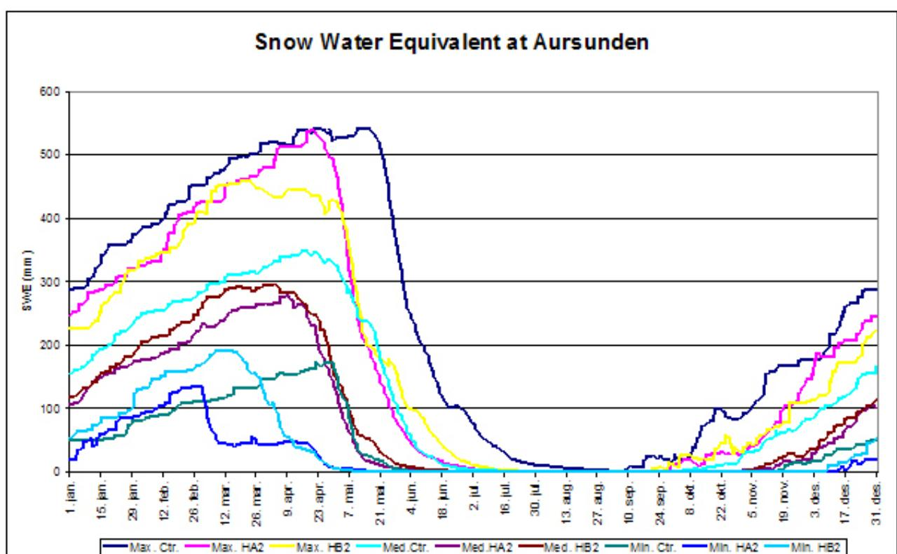
*Figure 3.10 Simulated Snow Water Equivalent (SWE) for the control period (1961–1990) and the scenario period (2071–2100) at Aursunden in Upper River Glomma. The figure shows the daily median, maximum and minimum value for the control period and the scenario period based on the A2 and B2 scenario of the HadleyAm3H- model.*
