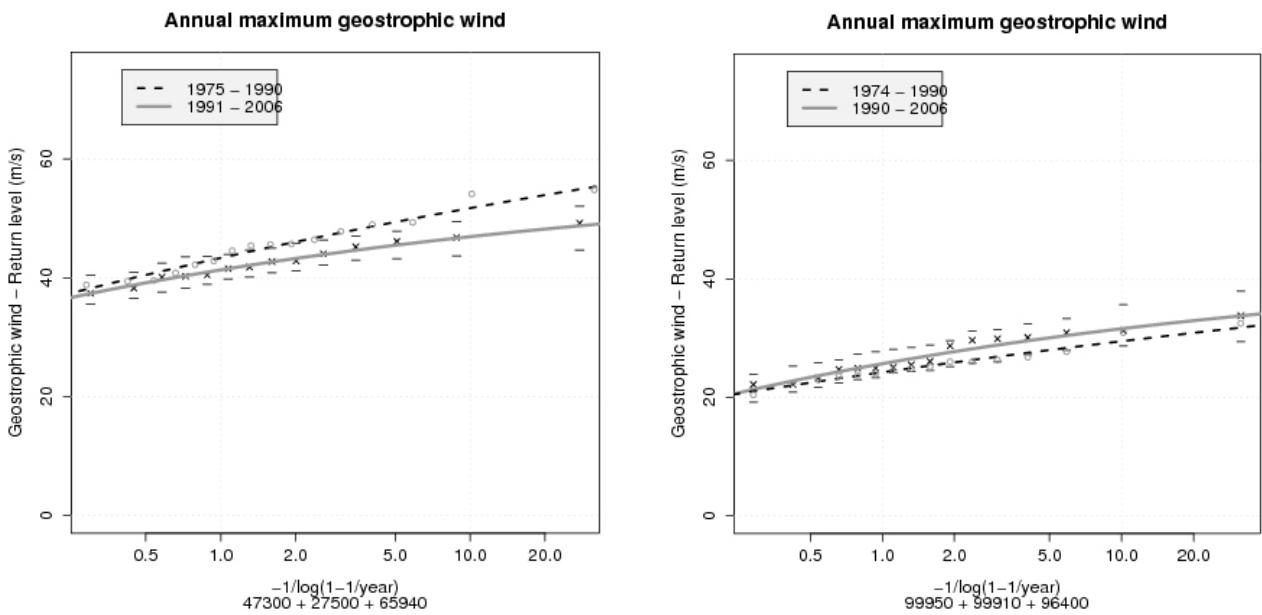
**Figure 5.3** Extreme value analysis of geostrophical winds estimated for two different triangles based on historical measurements from
