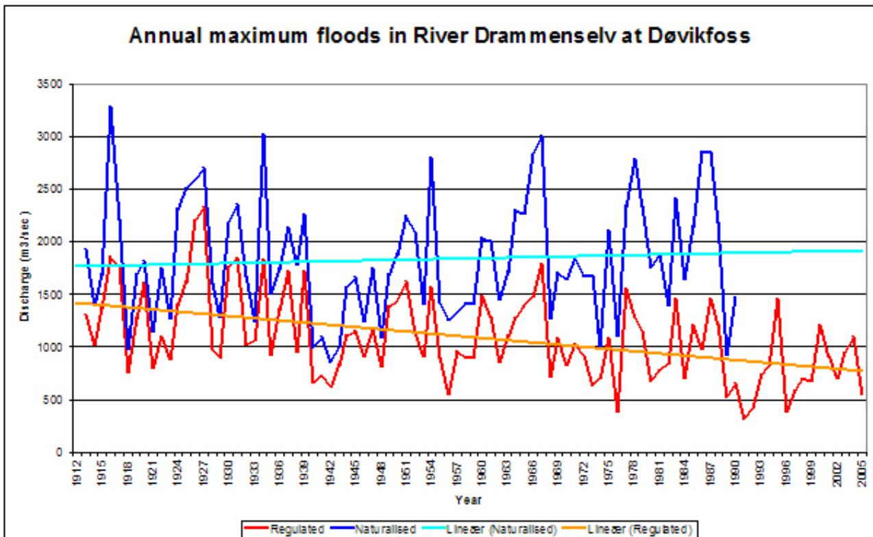
*Figure 3.9 Regulated and naturalised annual floods at Døvikfoss in River Drammenselv. The reduction in the flood magnitude is caused by 38 upstream reservoirs and the difference is typical of a heavily regulated water course.*
