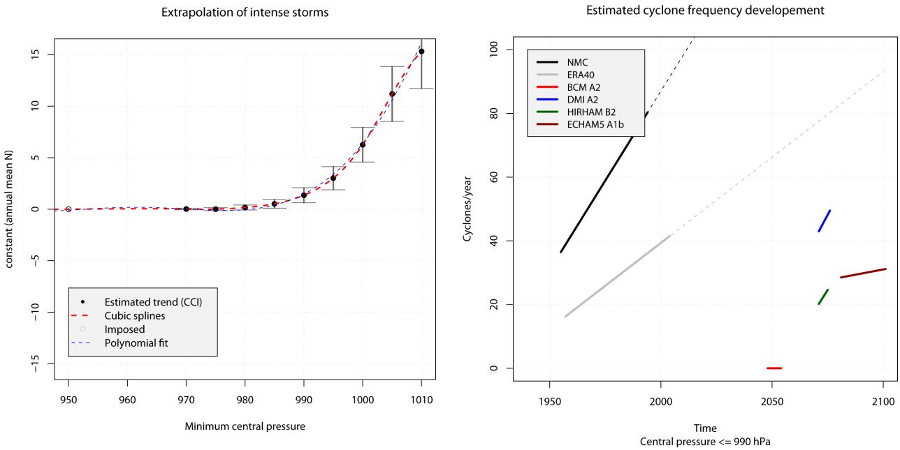
Figure 5.7 Left: function showing how the trend magnitude varies with the central pressure of the storms. Right: estimates of the storm frequency based on rCM results as well as observed trends (ERA40 & NMC).
