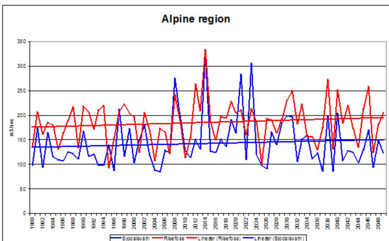
*Figure 3.11 Variability of the annual flood in alpine basins in Norway based on a transient run 1980–2049 of the hydrological model driven by the ECHAM4/OPYC3 model, the IS92A emission scenario and downscaling by the HIRHAM model.*
