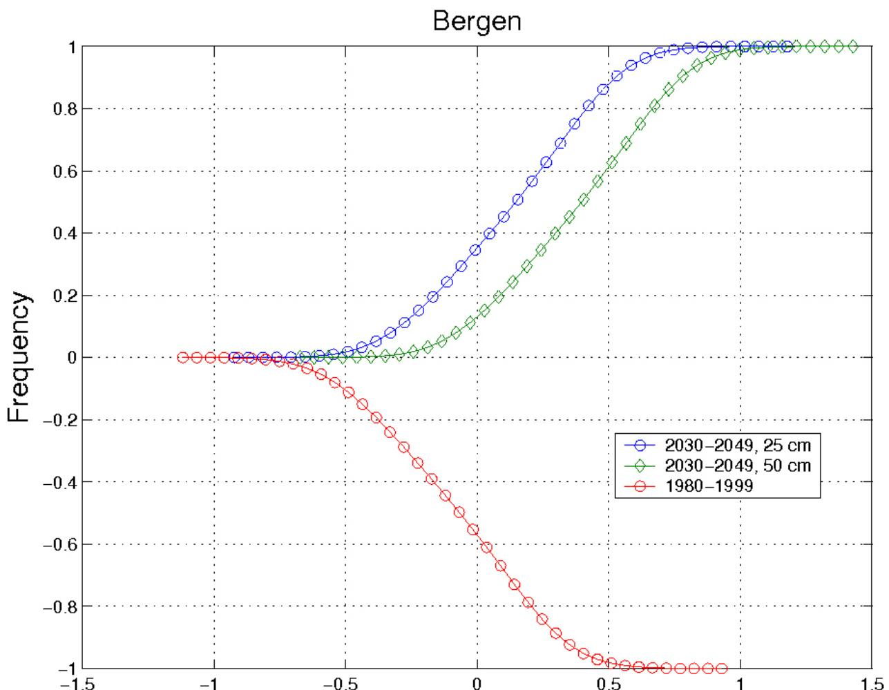
*Figure 6.4* Cumulative density functions for Bergen using the RegClim MPI-GSDIO simulations, with two different shifts in mean SLH in the future period (adjusted for continental uplift). The CDF is the integral of the PDF, shown in Figure 6.1, shifted to account for the mean SLH and the uplift.
