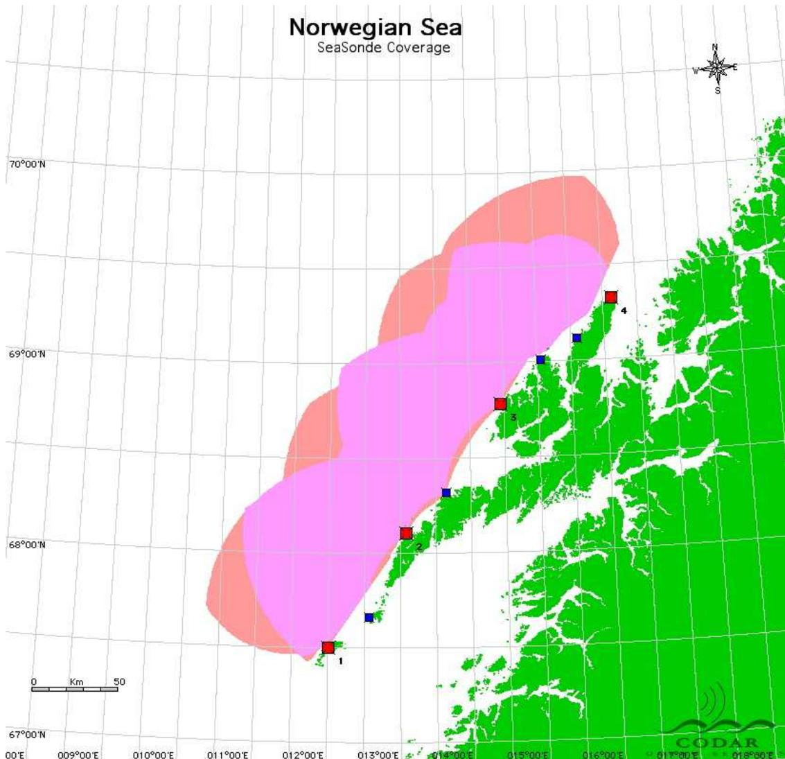
**Figure 26: Theoretical coverage using a medium-range HF system in Lofoten. The range goes up with lower frequency, but the spatial resolution goes down.**
