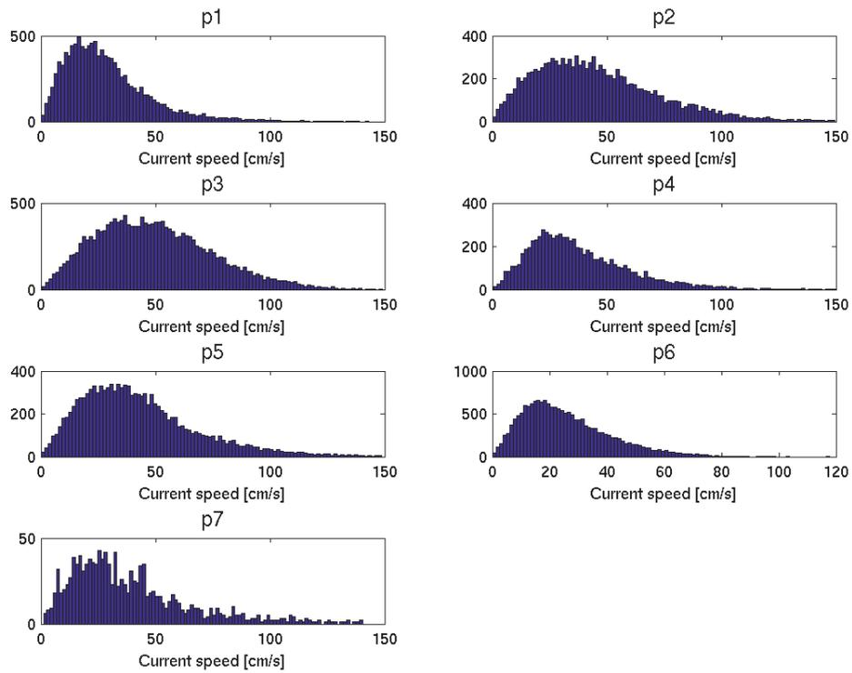
**Figure 5: Histograms of CODAR current speed for the 7 locations shown in Figure 4. No outliers have been removed.**
