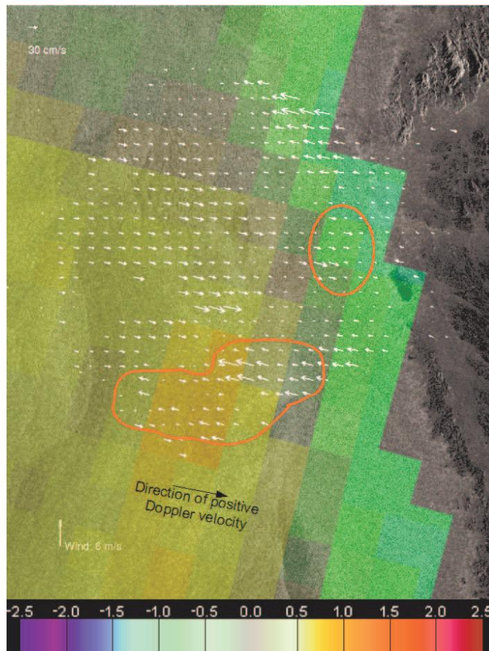
**Figure 19: Envisat ASAR roughness image (greyscale) overlaid surface Doppler velocity (colour scale m/s) for the same scene and HF radar current vectors which are projected into the direction of positive Doppler velocity (black arrow). The SAR image is acquired 26 December 2008 10:21 UTC, and the HF radar measurements are from the nearest hour. Wind speed and direction from the NCEP forecast model is indicated with the yellow arrow in the lower left.**
