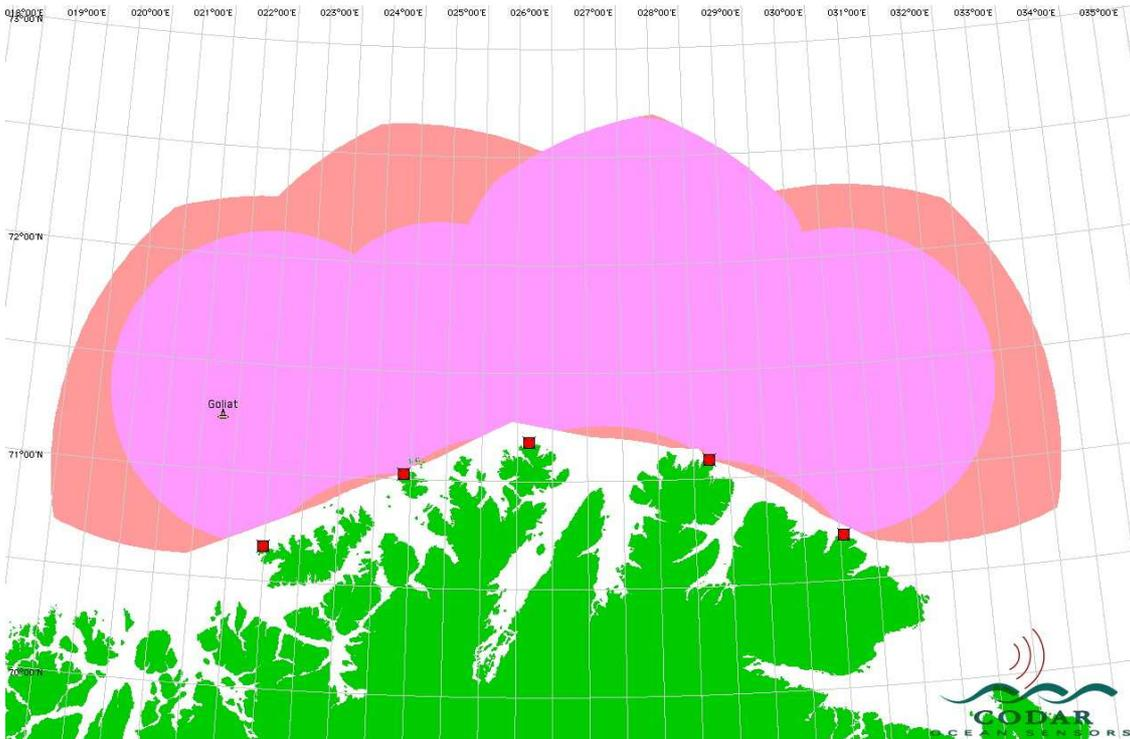
**Figure 28: Theoretical coverage using a long-range (5 MHz) HF system in Finnmark. This map covers Goliat adequately.**
