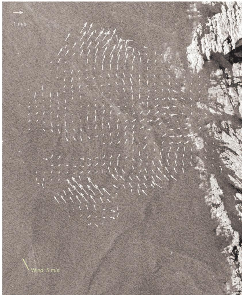
**Figure 17: Envisat ASAR roughness image from 24 December 2008, 21:10 UTC, overlaid CODAR current vectors for the nearest hour. Wind speed and direction from the NCEP GFS model is indicated with the yellow arrow.**
