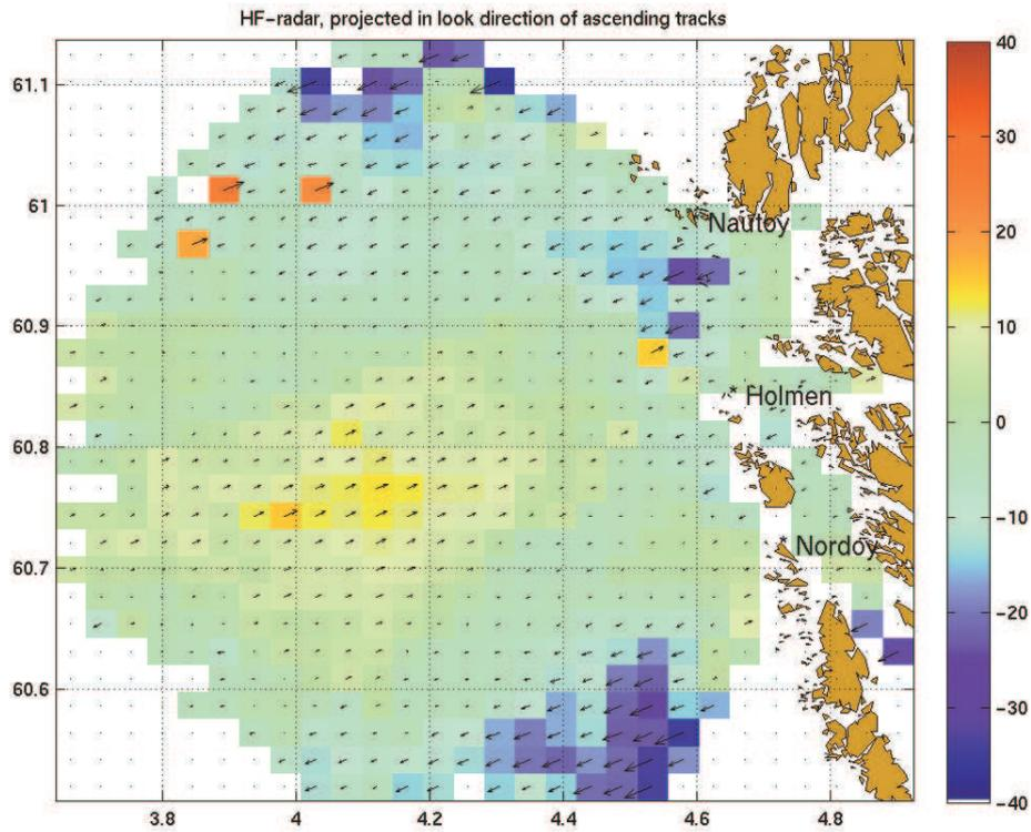
**Figure 22: Averaged CODAR vectors projected in the SAR look direction for ascending (northwards) satellite tracks. Only data collocated in time with 31 Envisat ASAR overpasses in 2008 are used. The background colour indicates the magnitude of the CODAR speed in this direction, and the arrows indicate the direction of positive Doppler velocity. The unit of the colour bar is cm/s.**
