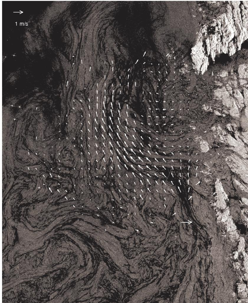
**Figure 16: An Envisat SAR roughness image from 8 May 2008, 10:12 UTC, off the coast of Fedje. The dark bands on the image are interpreted as areas where natural surface slicks (e.g. biogenic oils) are collected and redistributed by the surface current. The white arrows are the surface current measurements from the CODAR for the nearest hour, with the scale displayed in the upper left.**
