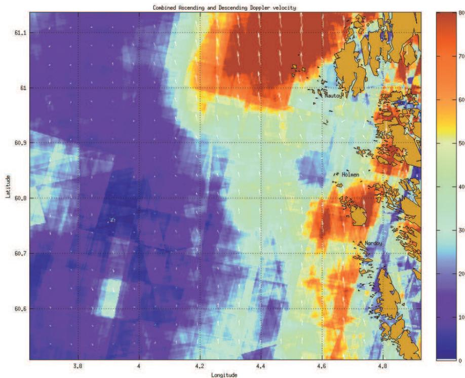
**Figure 25: 2D surface Doppler velocity field obtained by combining mean Doppler velocity fields for ascending and descending satellite passes. The contribution from wind has been removed by comparison with the Codar current field, as described in the text. Note that the coverage is slightly larger than for the mean Codar fields shown above.**
