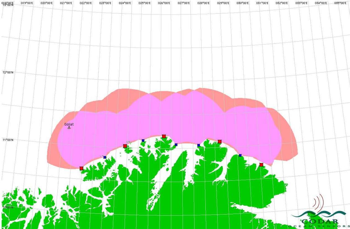
**Figure 27: Theoretical coverage using a medium-range HF system in Finnmark.**
