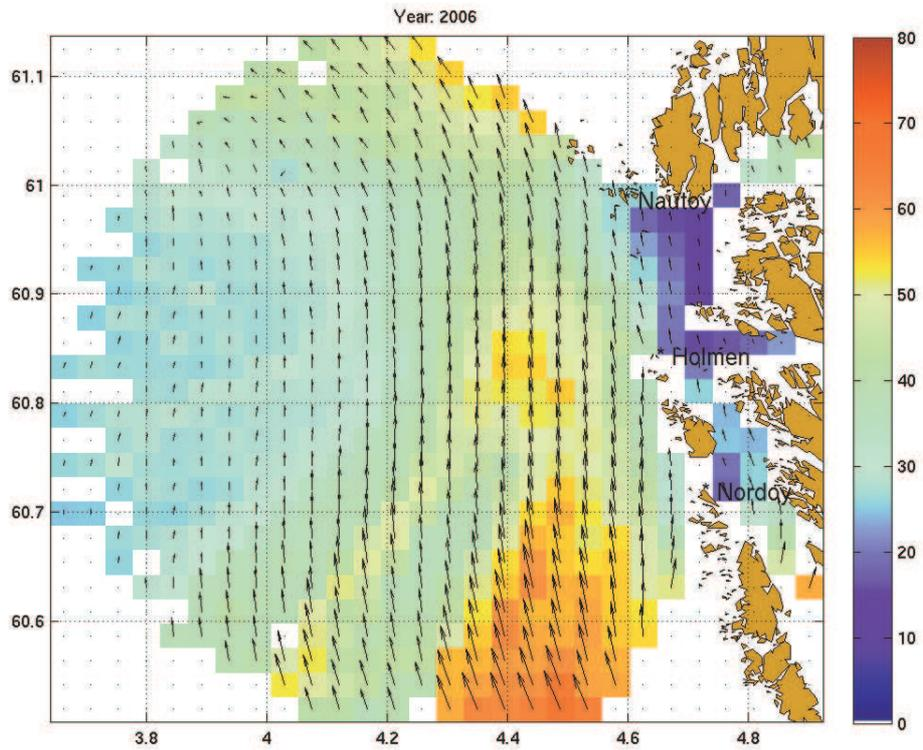
**Figure 1: CODAR current at Fedje averaged for the period 29 June – 31 Dec 2006. The colour scale indicates current speed [cm/s]. The overlaid vectors are obtained by averaging the eastward and northward components in time. The three radars are marked from south to north as “Nordoy”, “Holmen” and “Nautoy”.**
