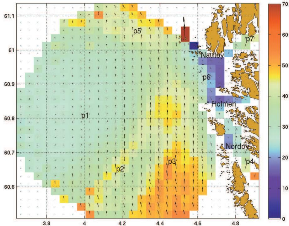
**Figure 4: Location of 7 positions (p1-p7) where temporal distribution of current speed and directions are investigated. The background colour and arrows are the CODAR current averages from 29 June 2006 to 31 Dec 2008.**
