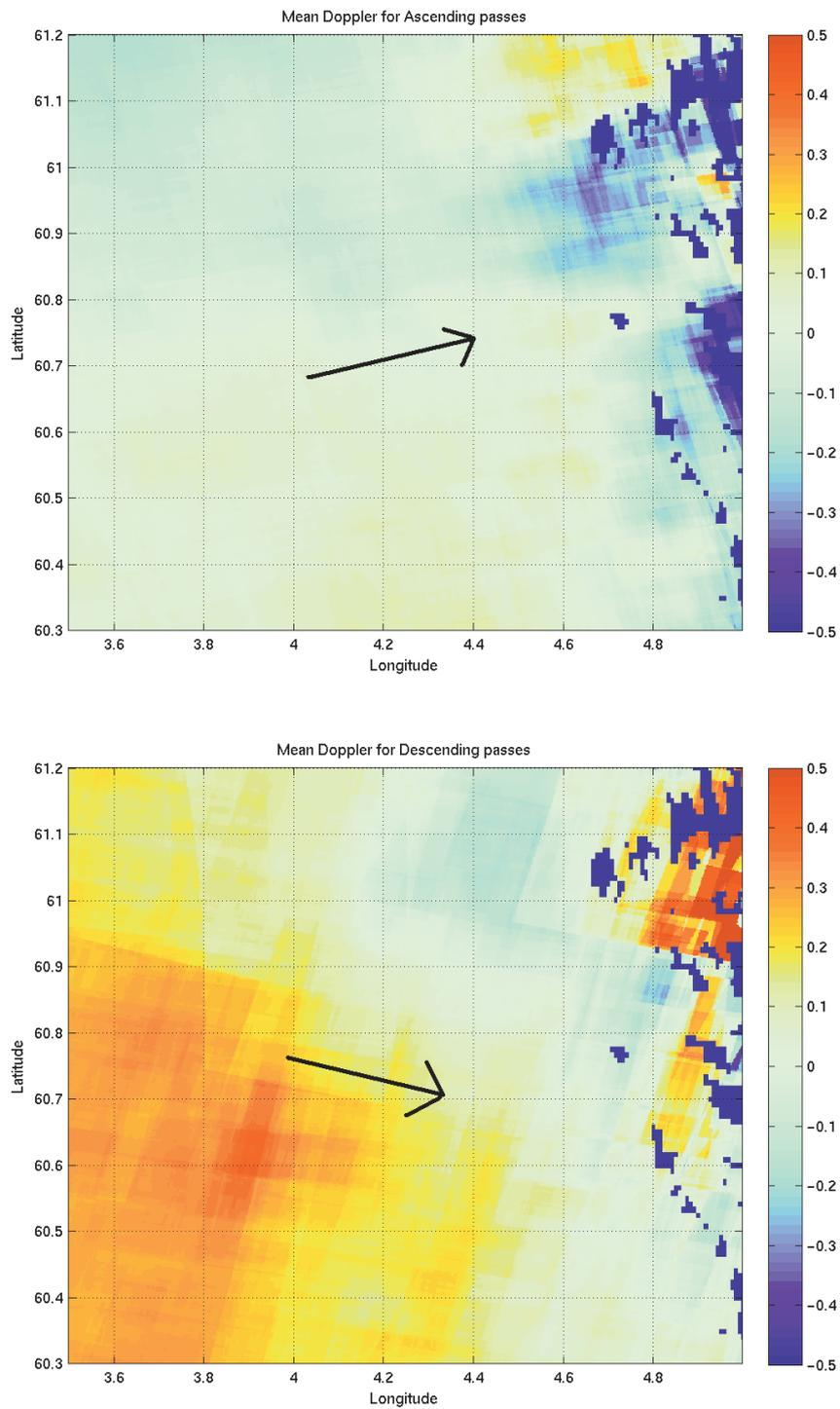
**Figure 24: Mean surface Doppler of 50 ascending (upper) and descending (lower) Envisat ASAR scenes from 2008. The angle between the look directions (marked with black arrows) is  $2\varphi=26^\circ$ .**
