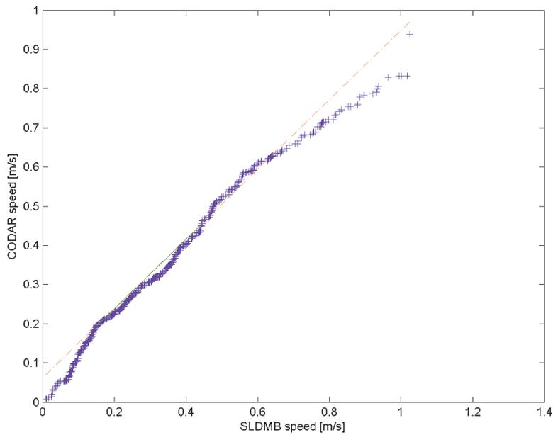
**Figure 8: Quantile-quantile plot of speed of drifters (SLDMB) and radar current (CODAR). The quantile-quantile plot juxtaposes measurements of similar cumulative probability, *i.e.*, values which are equally likely to be exceeded. As can be seen the distribution is comparable over the range of speeds observed, but the radars underestimate the speed somewhat.**
