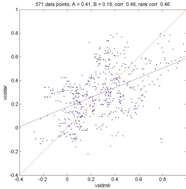
**Figure 7: Correlation between northward velocity  $v$  of drifters (SLDMB) and radar (CODAR).**
