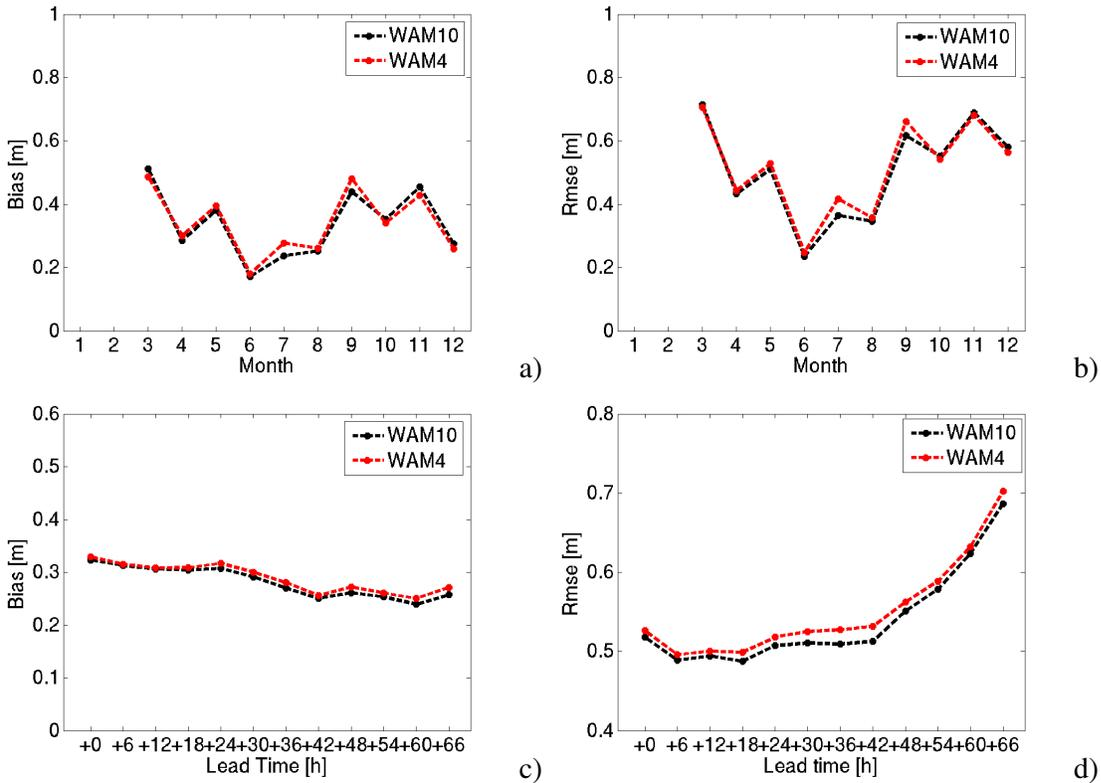
Figure 10: Comparison of the significant wave height from WAM10 and WAM4 during 2009. Figures a) and b) show the BIAS and the RMSE variation during the year for the analysis. Figures c) and d) show the BIAS and RMSE with Lead time.
