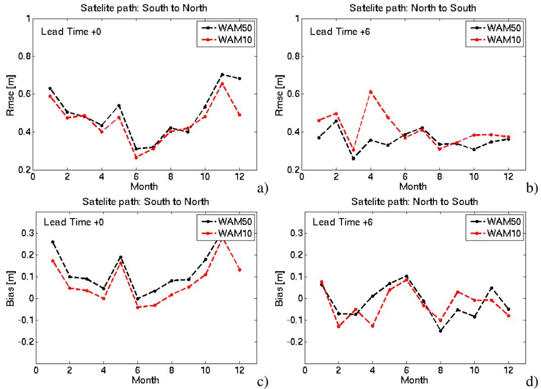
Figure 5: Displayed is a comparison of the wave height from WAM50 (black line) and WAM10 (red line) for each month in 2009. Figure a): shows the RMSE for the analysis, for the ascending path, figure b): shows the RMSE for the 6 hour forecast for the descending path. Figure c): shows the monthly BIAS (model minus observation) for the analysis for the ascending path and figure d): shows the BIAS for the 6 hour forecast for the descending path.
