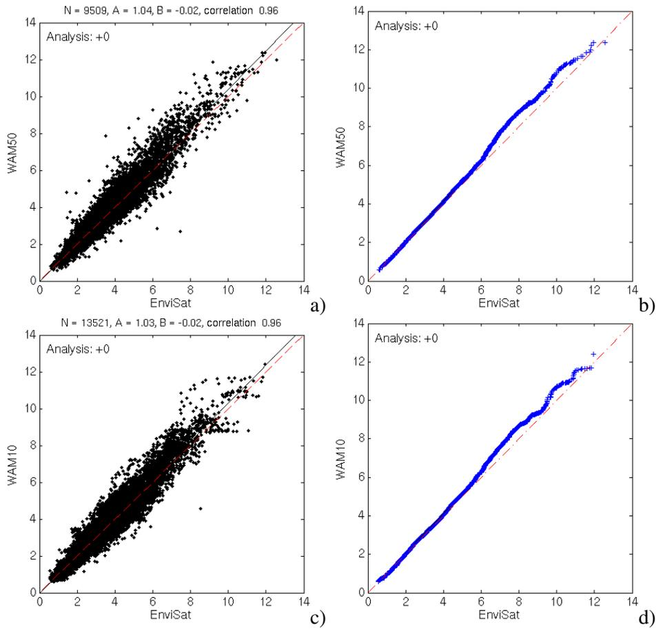
Figure 4: Shown are scatter and Q-Q plots between observed and modeled wave height for WAM10 and WAM50. The plots includes model results and observations from ENVISAT for the year 2009. The black line is the linear regression while the red dashed line represents the perfect fit between the two data sets.
