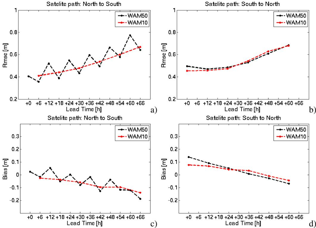
Figure 6: Displayed is the mean RMSE and BIAS (model minus observation) for each lead time for both WAM10 (red line) and WAM50 (black line). Figure a) shows the the RMSE for the descending path, while figure b) shows the RMSE for the ascending path. Figure c) shows the BIAS for the descending path, while figure d) shows the BIAS for the ascending path.
