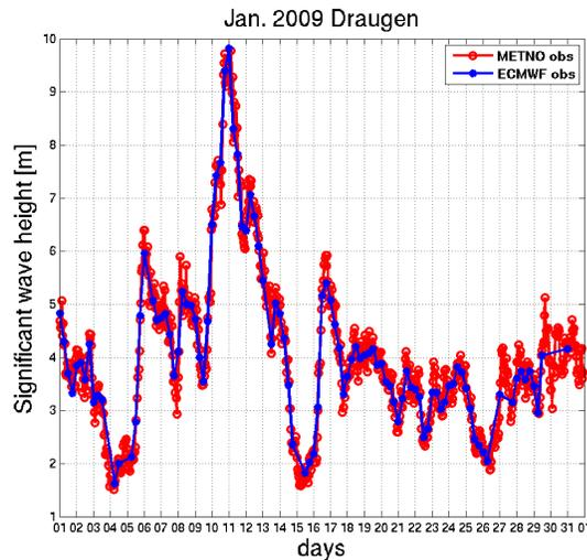
Figure 3: Time series of raw 20min (red line) and processed 4hr mean (blue line) observations for the month of January 2009 at station Draugen. The raw data are from met.no and the processed data from ECMWF.
