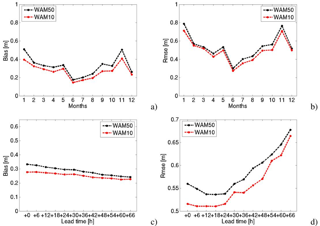
Figure 9: Comparison of the significant wave height from WAM50 and WAM10 during 2009. Figures a) and b) show the BIAS and the RMSE variation during the year for the analysis. Figures c) and d) show the BIAS and RMSE with Lead time.
