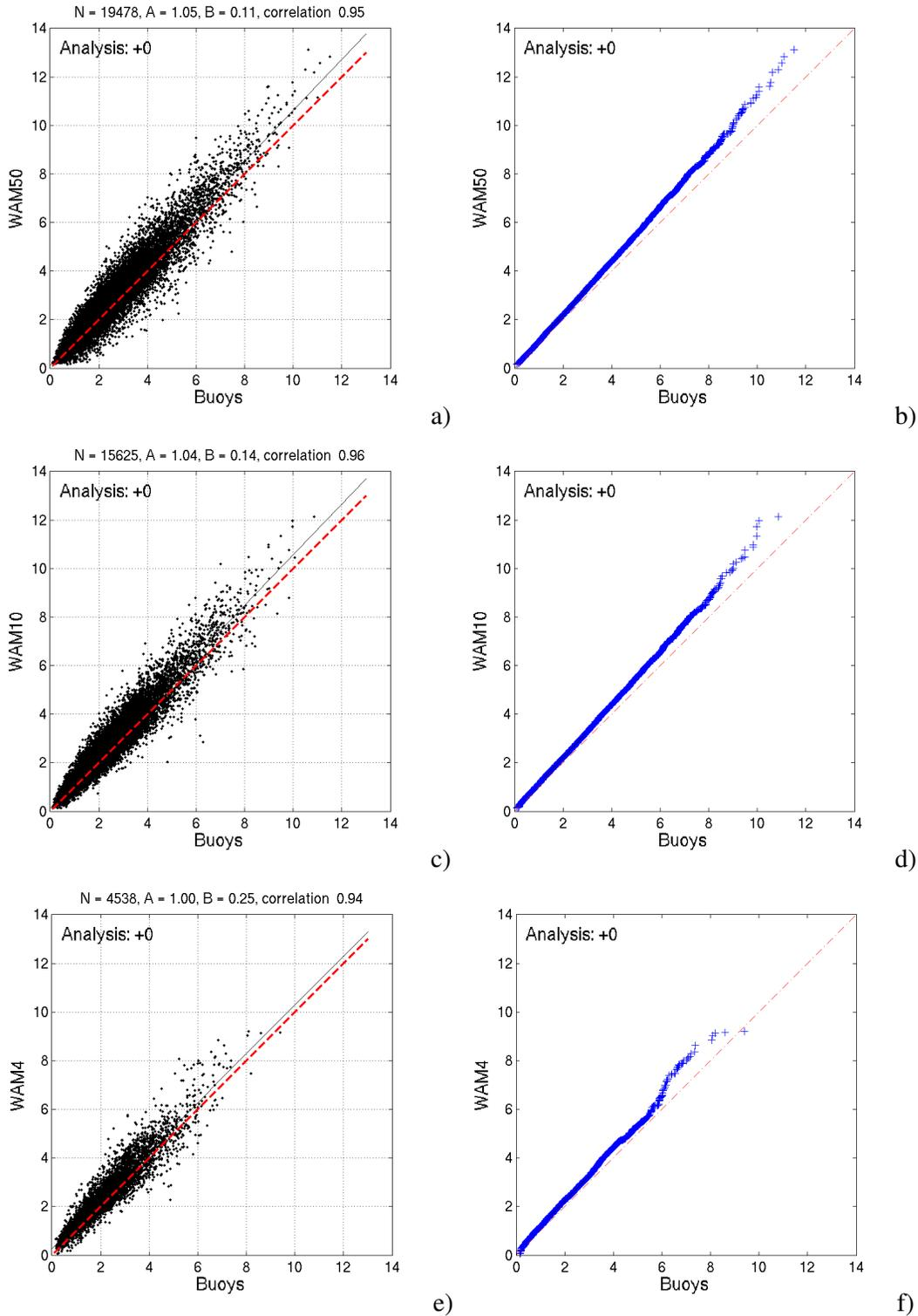
Figure 8: Scatter and quantile-quantile between observed and modeled significant wave height for WAM50 a) and b), for WAM10 c) and d) and for WAM4 e) and f). The black line is the linear regression line while the red line in the scatter plots refers to the perfect fit between the two data sets. The red line in the quantile-quantile plots indicates that the two sets come from a population with the same distribution.
