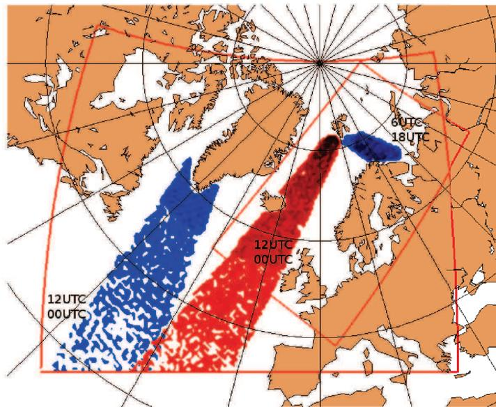
Figure 2: Displayed is the density of the collocated ENVISAT RA-2 observations during 2009. Red contours shows the coverage when the satellite is descending, while the blue contours shows the coverage when the satellite is ascending. The hours are the approximate time for the given paths, with a time span of +/- 30 min. The outer red area is the domain of WAM50, while the inner red area is the domain of WAM10.
