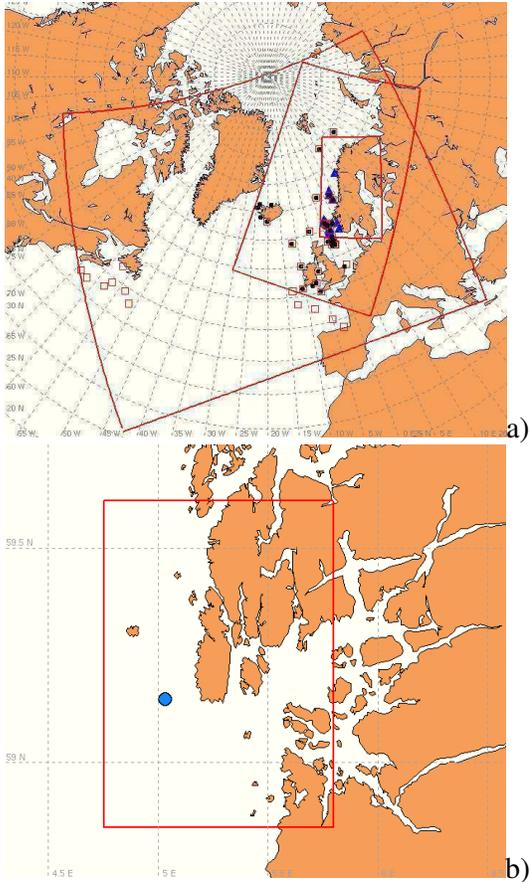
Figure 1: a) Buoys and domains of WAM50, WAM10 and WAM4. The large domain corresponds to WAM50 the middle to WAM10 and the smallest to WAM4. b) The domain of SWAN for the Karmøy area, with the one and only buoy, Hywind.
