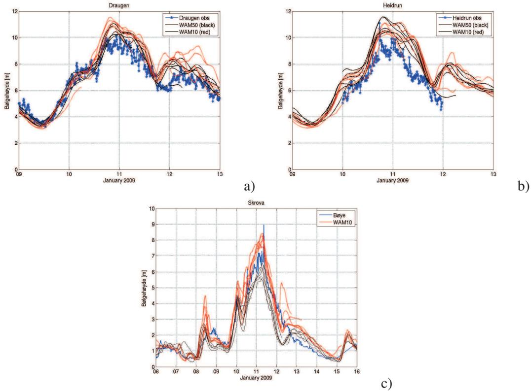
Figure 14: Observations of 10 min significant wave height at Draugen, Heidrun and Skrova (blue), and overlapping prognoses from WAM10 (red lines) and WAM50 (black lines). Figure a) and b) shows the results at Draugen and Heidrun for the period 9th - 13th of January 2009, and figure c) shows the results at Skrova for the period 6th - 16th of January 2009
