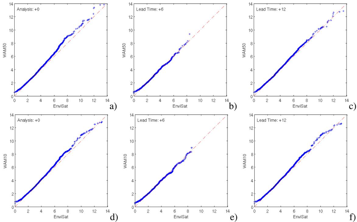
Figure 7: Shown are Q-Q plots between observed and modeled wave height for WAM10 and WAM50. The plots includes model results and observations from EnviSat for the year 2010. The black line is the linear regression while the red dashed line represents the perfect fit between the two data sets.
