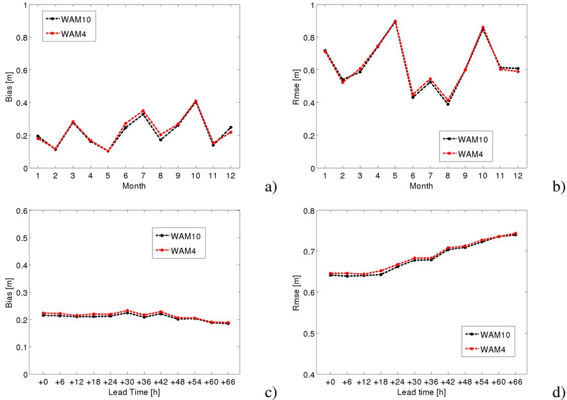
Figure 12: Comparison of the significant wave height from WAM10 and WAM4 during 2010. Fig.(a and b) show the bias and the rmse variation during the year for the analysis. Fig.(c and d) show the bias and rmse with Lead time.
