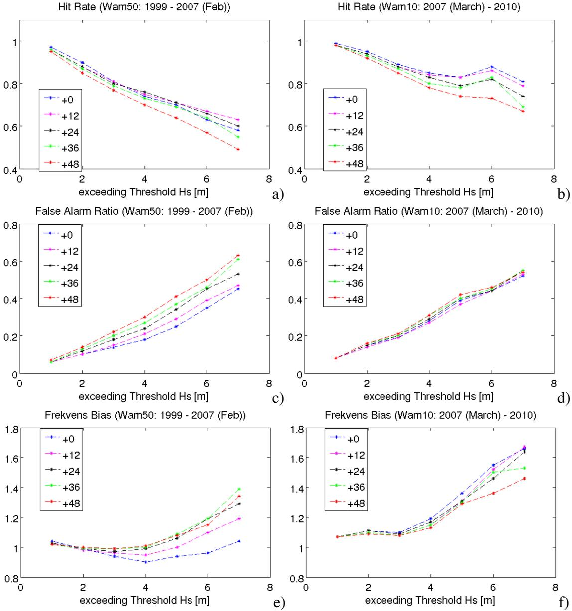
Figure 5: Shows the forecast skill of wave heights exceeding a threshold  $H_s$ . The statistics computed are Hit rate, False alarm ratio and Frequency bias. The left column shows results for the period 1999 to 2007 (February) for WAM50, while the right column show results for the period 2007 (March) through 2010 for WAM10.
