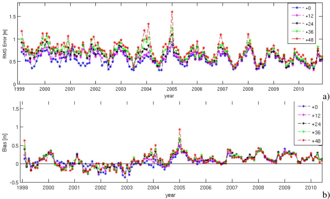
Figure 4: Time series of the rmse and bias for the forecast of Hs for the period 1999 to 2010. Note that model results from WAM50 are included for the period before March 2007, while model results from WAM10 are included for the later period. Observations from six sites in the Norwegian and the North Sea is applied. Ekofisk, Sleipner, Troll A, Gullfaks C, Draugen and Heidrun
