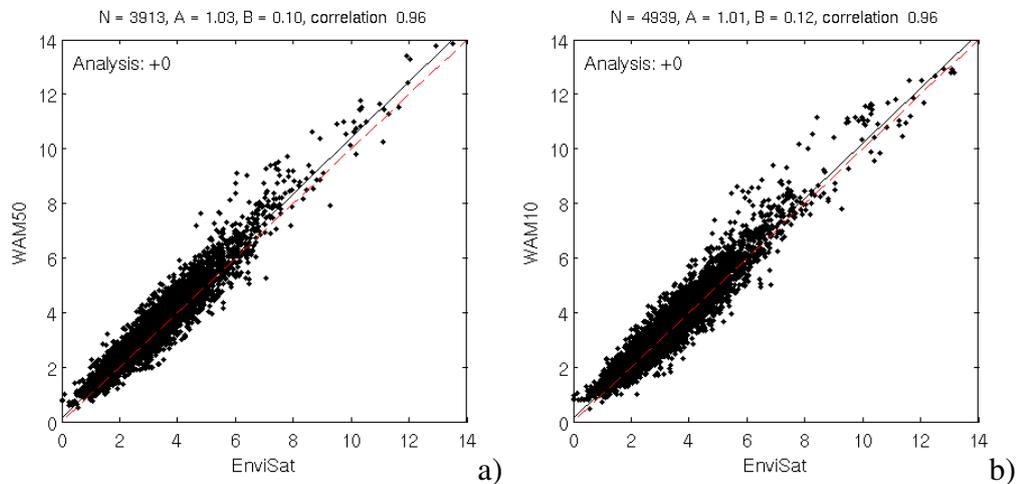
Figure 6: Shown are scatter plots between observed and modeled wave height for WAM10 and WAM50. The plots includes model results and observations from EnviSat for the year 2010. The black line is the linear regression while the red dashed line represents the perfect fit between the two data sets.
