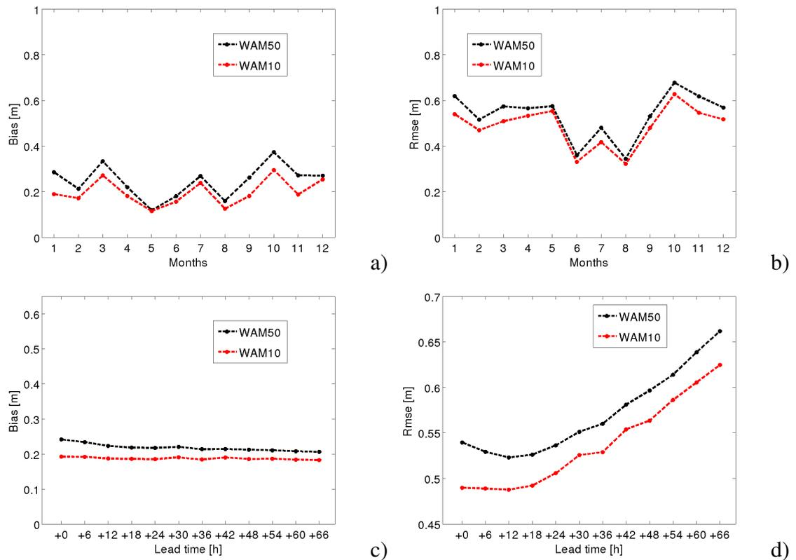
Figure 11: Comparison of the significant wave height from WAM50 and WAM10 during 2010. Fig.(a and b) show the bias and the rmse variation during the year for the analysis. Fig.(c and d) show the bias and rmse with Lead time.
