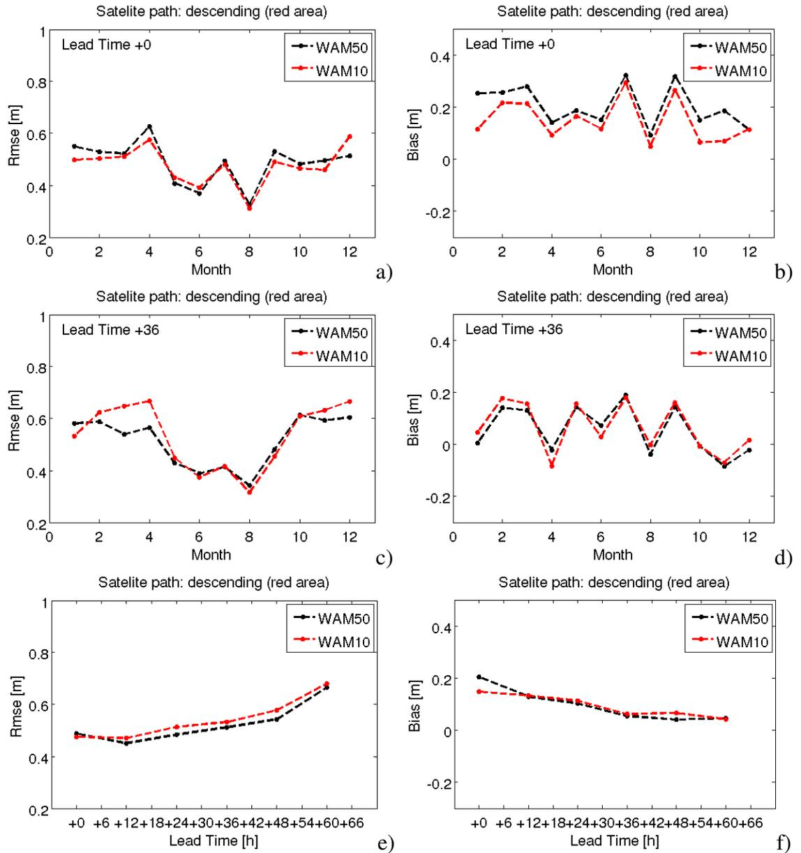
Figure 8: Displayed is a comparison of the wave height from WAM50 (black line) and WAM10 (red line) for the descending path. Fig.(a and b): shows the rmse and bias for the analysis, Fig.(c and d): shows the rmse and bias for the 36 hour forecast Fig.(e and f): shows the mean rmse and bias (model minus observation) for each lead time for both models.
