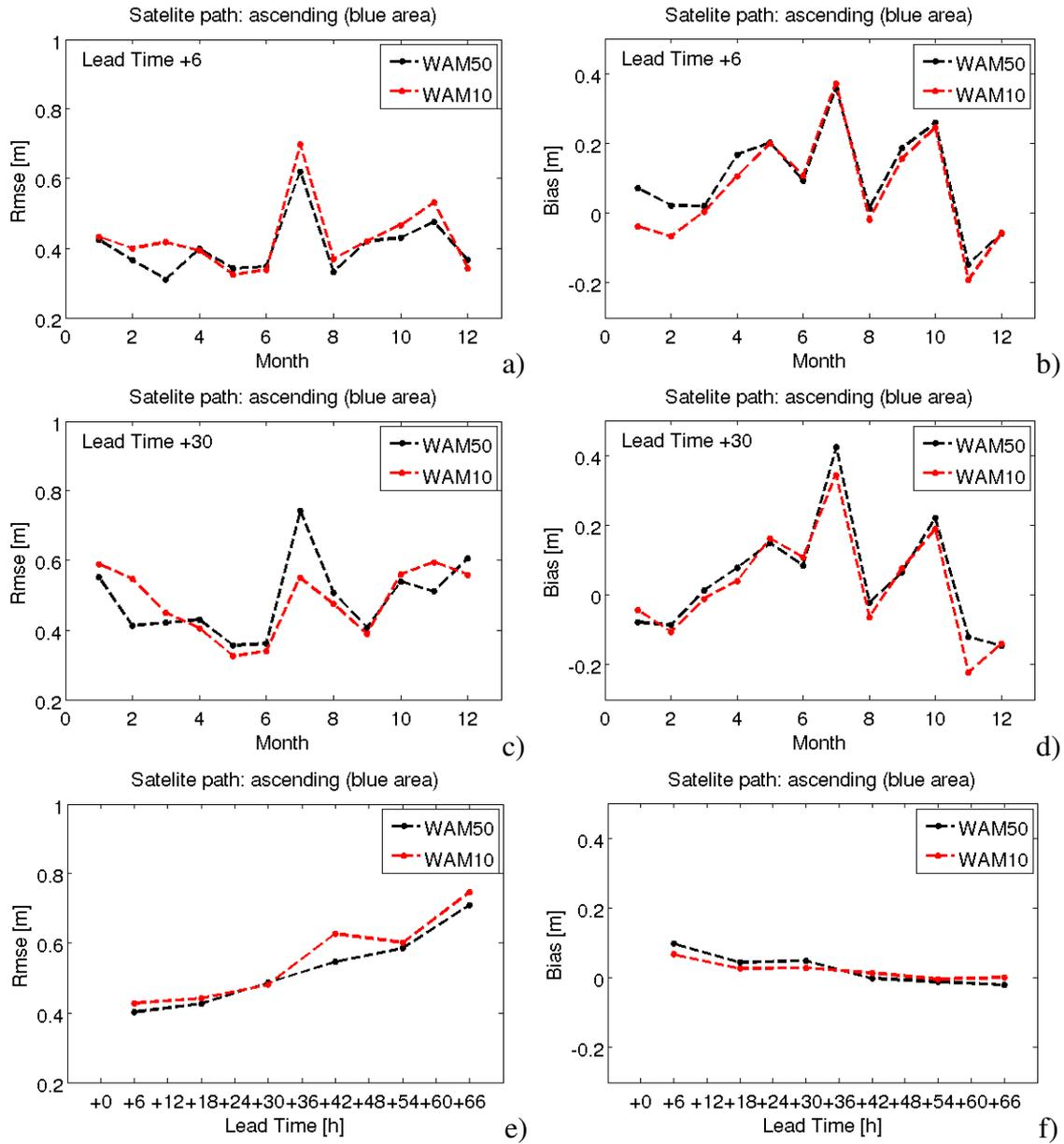
Figure 9: Displayed is a comparison of the wave height from WAM50 (black line) and WAM10 (red line) for the ascending path. Fig.(a and b): shows the rmse and bias for the 6 hour forecast, Fig.(c and d): shows the rmse and bias for the 30 hour forecast Fig.(e and f): shows the mean rmse and bias (model minus observation) for each lead time for both models.
