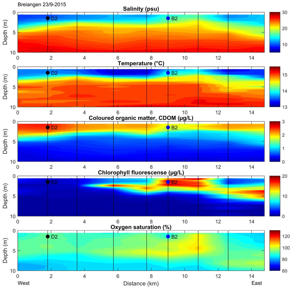
Figure 13: As for Figure 12, but for September 23rd 2015. The point D2 represents the river water and the point B2 represents marine water with algae.
