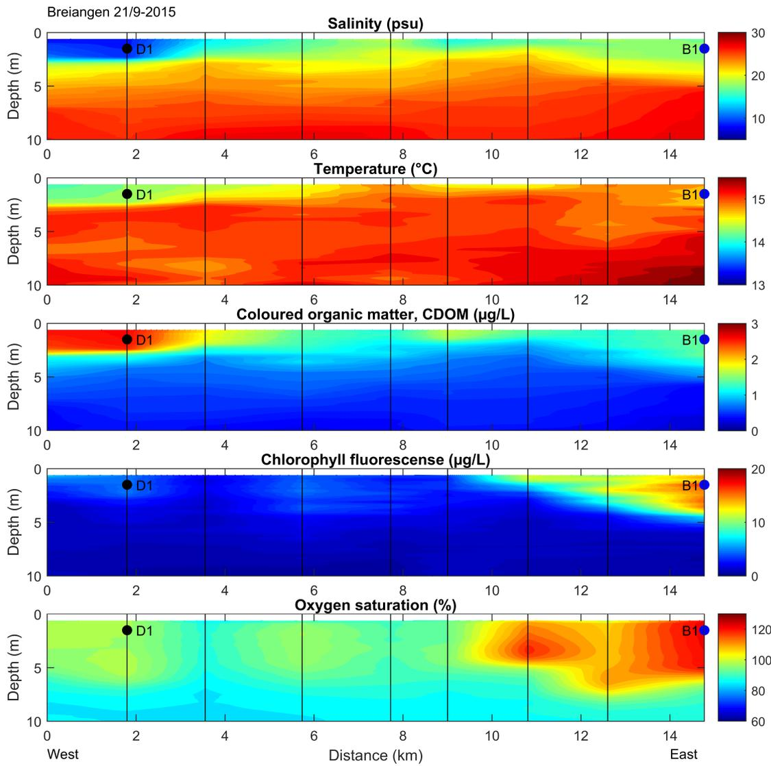
Figure 12: Salinity, temperature, coloured organic matter, chlorophyll fluorescence and oxygen saturation in the upper 10 meters of the Breianger transect, taken on September 21st 2015. The point D1 represents the river water and the point B1 represents marine water with algae.
