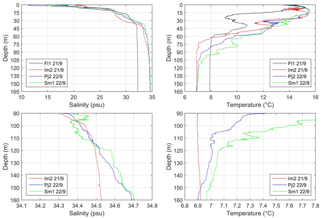
Figure 11: Profiles of salinity (left) and temperature (right) at four stations in the Oslofjord. The upper panels show the depth range from 0 to 165 m. The lower panels show the depth range from 90 to 160 m, and station FI1 is omitted.
