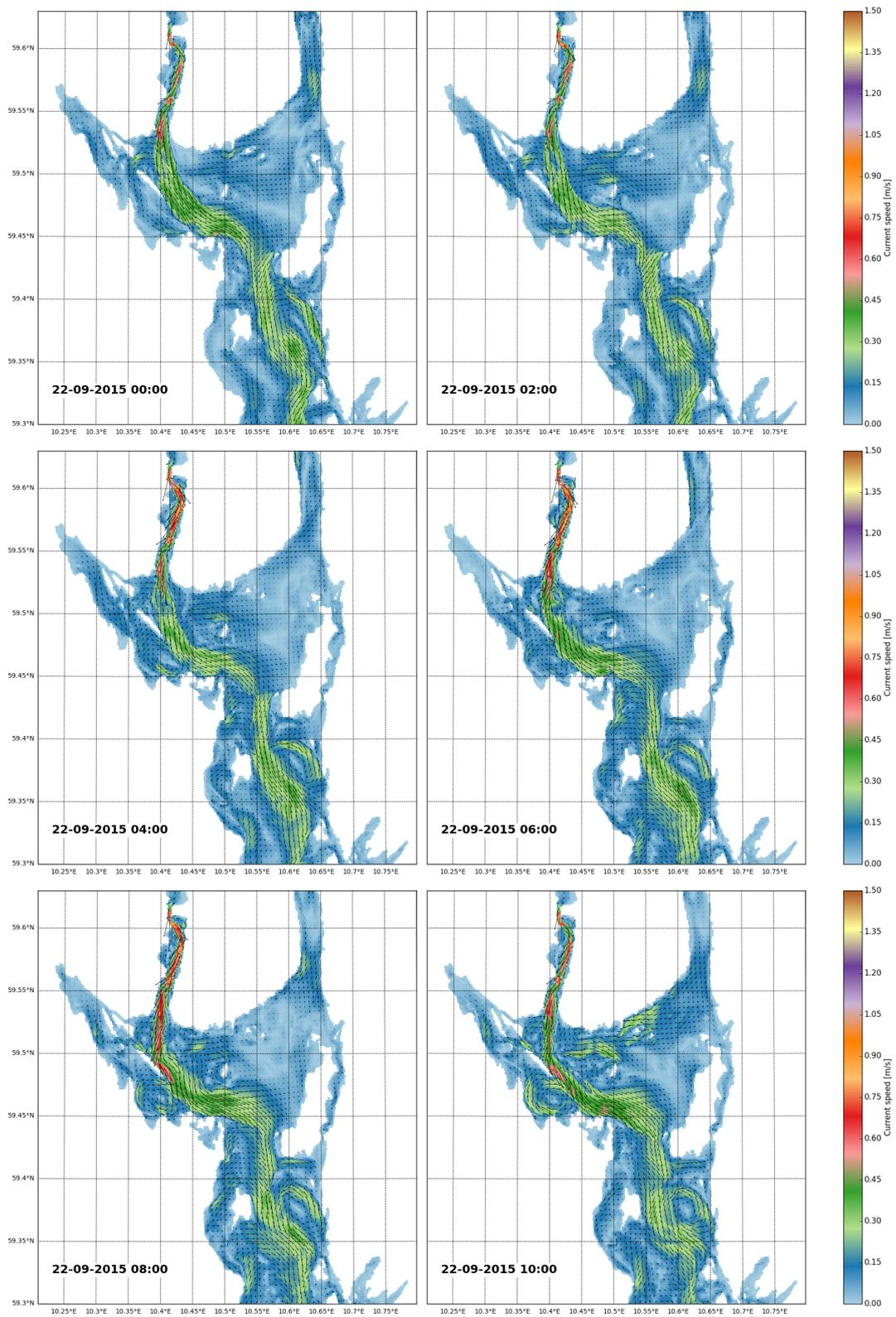
Figure 28: Simulated current fields at 2 meters depth every other hour during the cruise.
