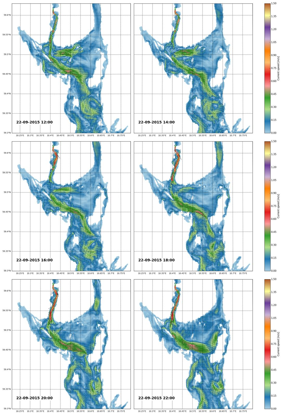
Figure 29: Simulated current fields at 2 meters depth every other hour during the cruise.
