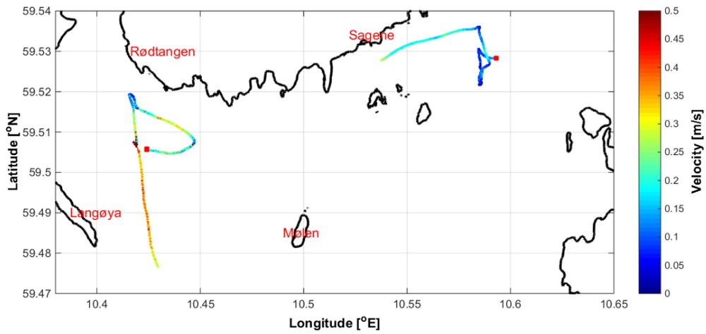
Figure 9: The path and velocity of the single drifters dropped in Breianger.
