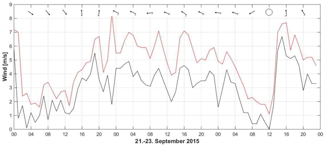
Figure 4: The hourly mean (black) and maximum (red) wind speed at Gullholmen measurement station during the time of the cruise. Data obtained from www.yr.no.
