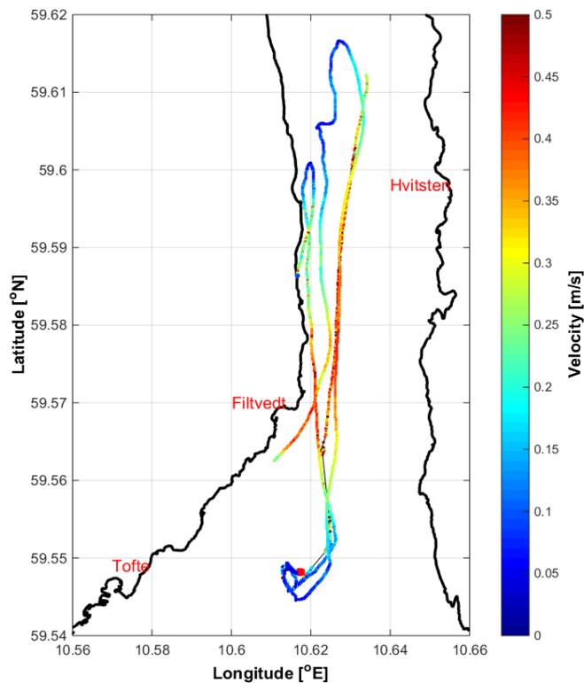
Figure 5: The path and velocity of the drifters dropped in zone A.
