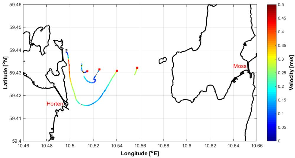
Figure 8: The path and velocity of the drifters dropped in zone C.
