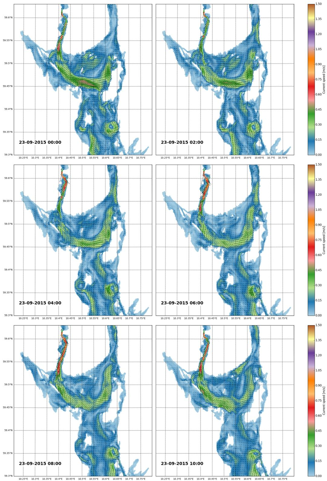
Figure 30: Simulated current fields at 2 meters depth every other hour during the cruise.
