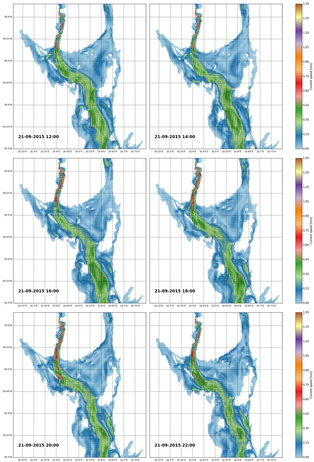
Figure 27: Simulated current fields at 2 meters depth every other hour during the cruise.
