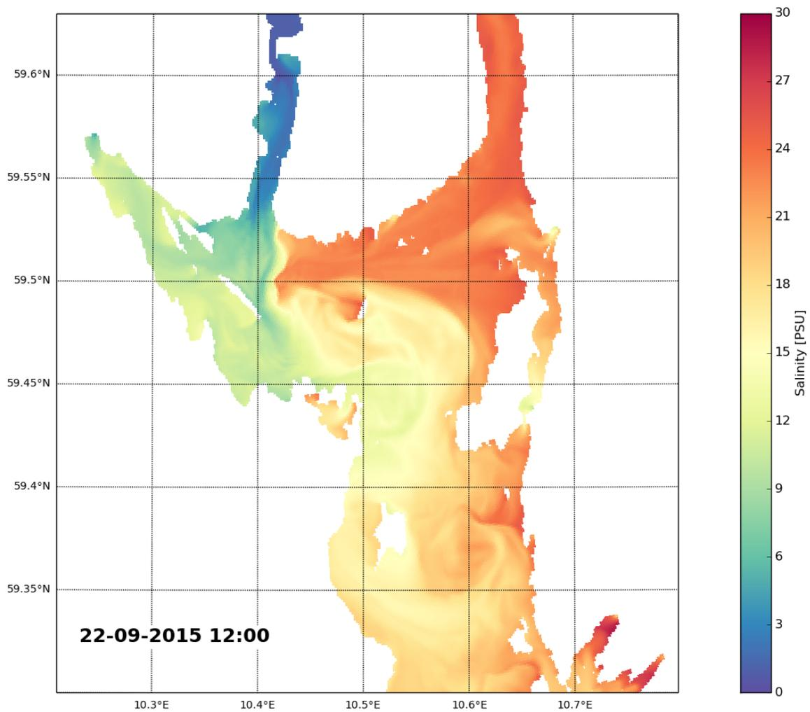
Figure 26: Sea surface salinity from the FjordOs model at approximately 24 hours into the cruise. Note the freshwater from the Drammensfjorden has spread out further compared to Figure 25.
