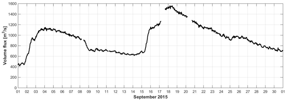
Figure 3: Observed flow rate of the Drammen river measured in Mjøndalen September 2015. Raw data obtained from NVE.
