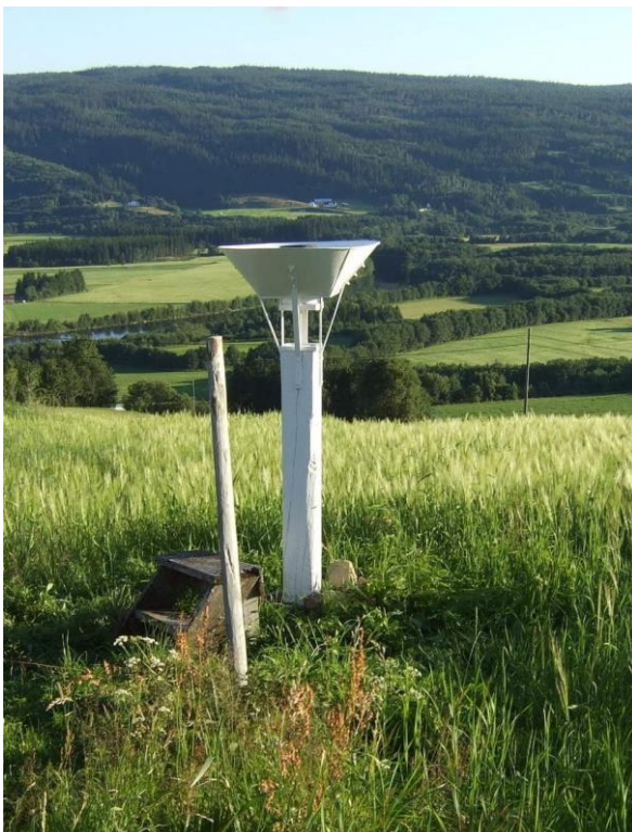
Fig 4. Precipitation gauge with a Nipher wind screen. There is a passage between the gauge and the screen that lets the snow fall to the ground avoiding filling up the area between the gauge and the screen (photo MET Norway: Lien in Selbu, Trøndelag county)
